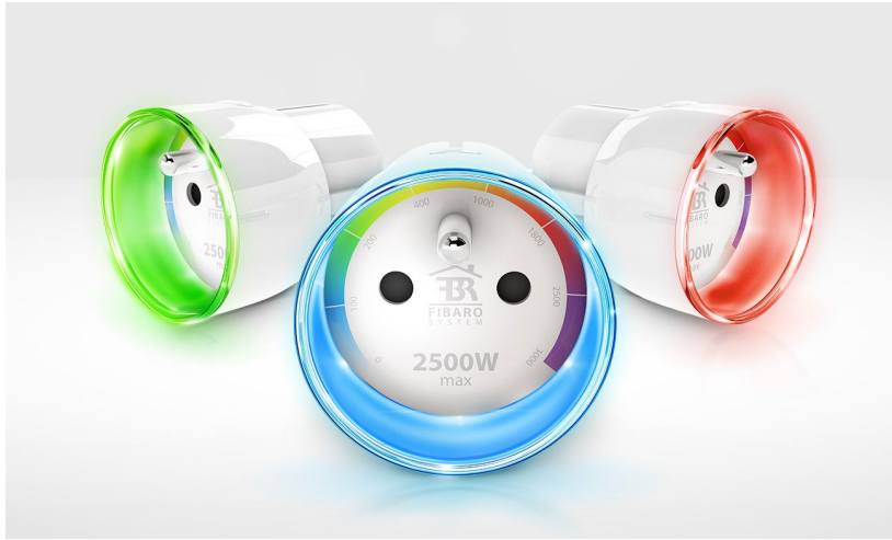
Figure 12 The Fibaro wall plug shows energy consumption from the plug is visualised through lighting up the rim of the plug with a color.
