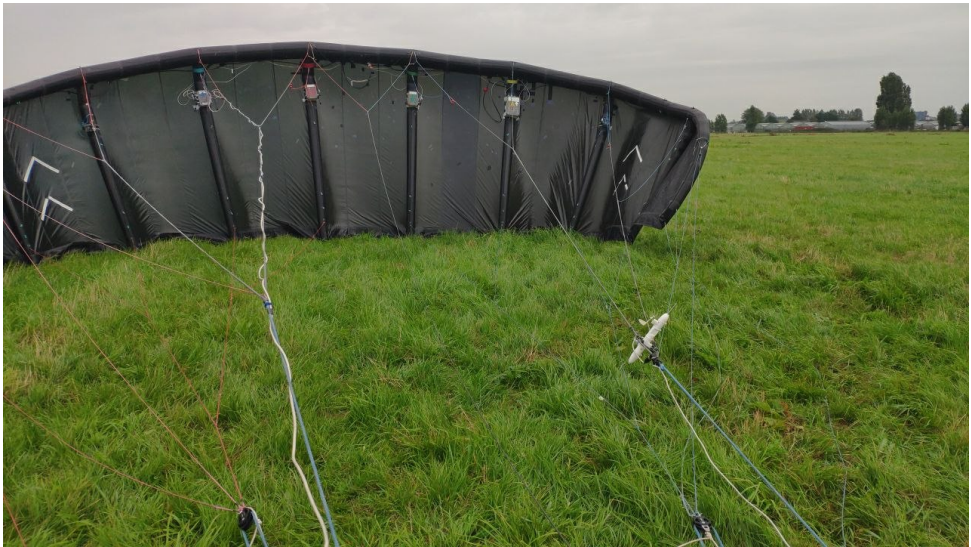
Figure 2.12: Fully instrumented V3.25B kite before launch. Courtesy of Kitepower B.V.
