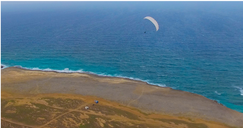
Figure 2.10: AWE system of Kitepower B.V. with a 60 m 2 kite and ground station integrated in a standard 20 ft container in operation on the Caribbean island Aruba in October 2021 (photo courtesy of Kitepower B.V.).
