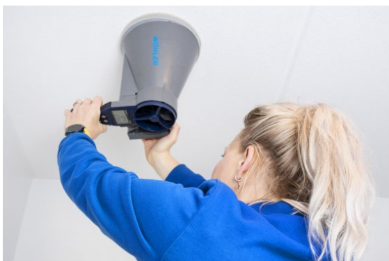
Figure 4.12: Ventilation calibration technician measuring flow
