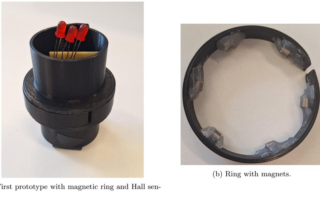
Figure 22: First complete prototype and a close up of the magnetic ring.
