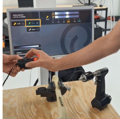
(b) The next screw type, locking (green), is selected by rotating the ring.
