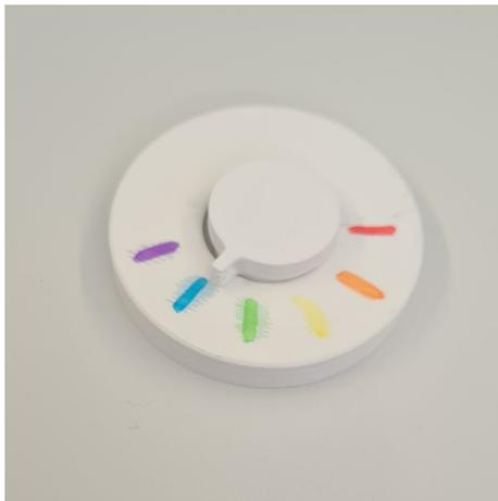
(a) Rapid prototype design for rotary knob.
