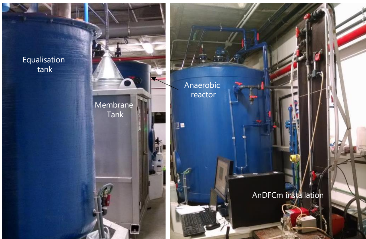
Figure 1.6. Pilot AnMBR plant (FCC-Aqualia) including the AnDFCm installation connected in bypass for in-situ sludge filterability measurements. The pilot was located at the Business Centre Porto do Molle, Nigrán, Pontevedra, Spain. Left and right are pictures taken from opposite sides.
