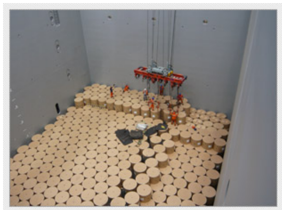
(c) Paper Roll Cargo: vertically oriented (Source: http://www.osy.co.jp/english/bulkers/secondary.php )
