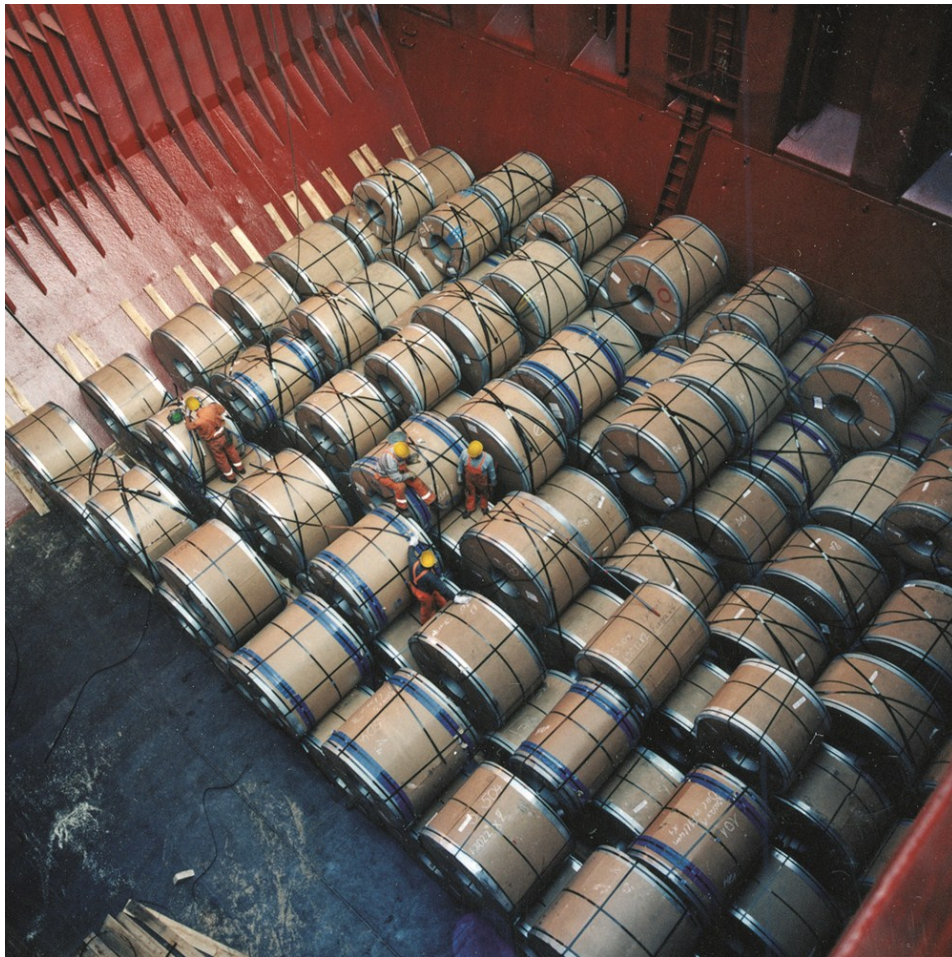
Figure H.1: Stevedores applying crossed lashing over coils
