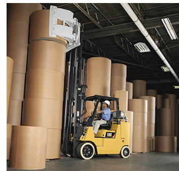
Figure 7.7: Paper roll lifted by clamp (Source: http://www.kellytractor.com/eng/products/forklifts/cat/Combustion-8000-15500-Lb.aspx )
