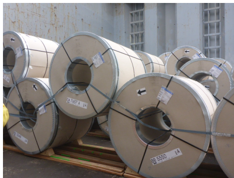
Figure 5.20: Hold 3: 4 lines of 3 layers thick hardwood dunnage, stacked max. 2 coils high
