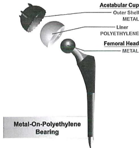
Figure 1.6: Various Components of a THR [21]
