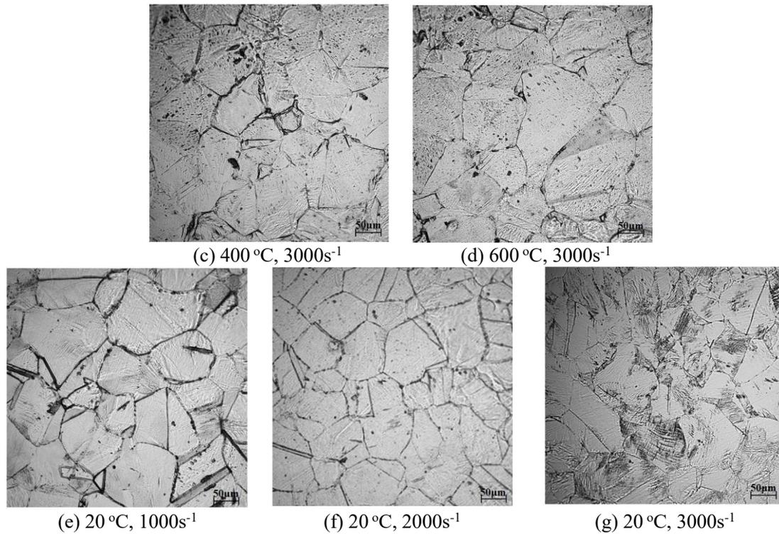
Fig. 12. Optical microstructures under different strain rates and temperatures.
