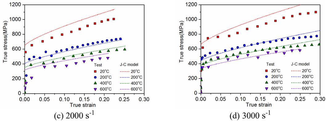
Fig. 11. Comparison between the test results and J-C model
