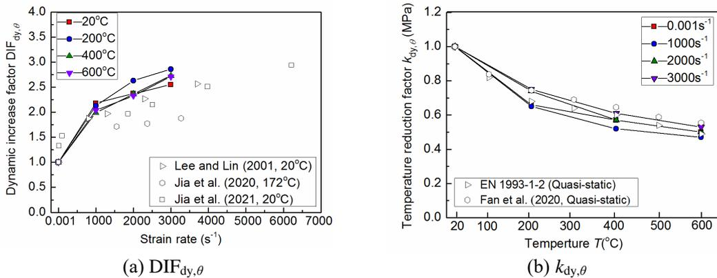
Fig. 9. Dynamic increase factors DIF<sub>dy,θ</sub> and temperature reduction coefficients  $k_{dy,θ}$
