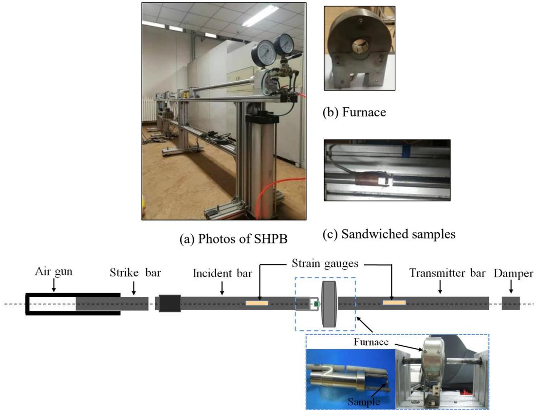
Fig. 4. Set-up for dynamic tests under elevated temperatures.
