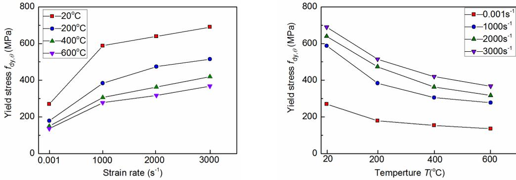
(a) Yield stress versus strain rate (b) Yield stress versus temperature
