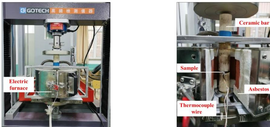
(a) Whole apparatus (b) Internal state of the furnace
