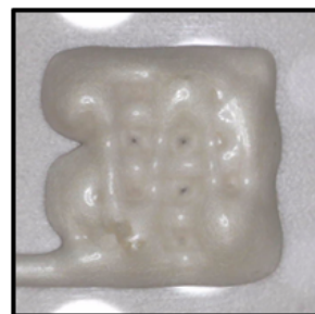
Figure 3.10: Raster print result for \text{Al}_2\text{O}_3 /HMWC mixture using the same volume-wise composition as the PS/PC mixture, showing significantly reduced print fidelity. 50% print speed (500 mm/min). Image size is approximately 10 × 10 mm.
