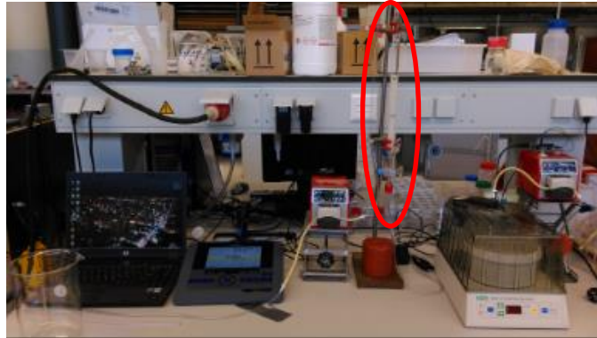
Figure 28 - An impression of the experimental IEX set-up, with the IEX-resin column (red oval).
