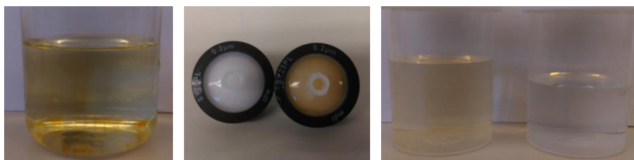
Figure 18 - Left to right: presence of \text{Fe}(\text{OH})_3 , difference between clean and spent 0.20 \cdot 10^{-6} [m] pore sized filters and difference between unfiltered and filtered \text{Fe}(\text{OH})_3 samples.
