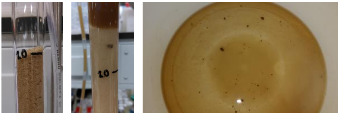
Figure 34 - Left to right: 0.20 [m] mixed solids in the column, fluidized mixed solids during washing including presence of a 'chunk' and a collection of washed solids, including 'chunks' after a failed attempt.
