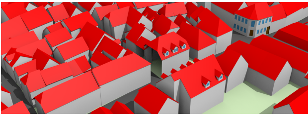
Figure 7: An example of a seemingly random error: missing wall polygons from a building, causing invalid solids. This error is likely caused by the conversion of the dataset from another format, during which the generation of the polygons failed.
