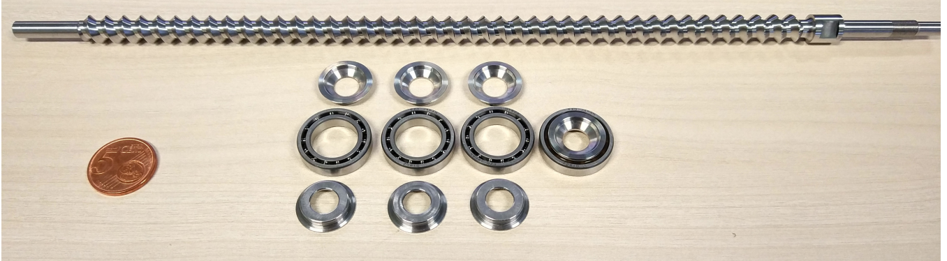
Fig. 25. The screw rod, rings and bearings for the functional prototype.
