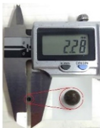
Figure 2. Conductive alginate capsule encapsulating a bitumen rejuvenator oil.
