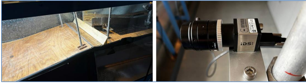
Figure 1. Photos of the 1:6 beach and 2:1 dike layout with berm (left) and detail of the IDS UI-31800CP-M-GL video-camera
