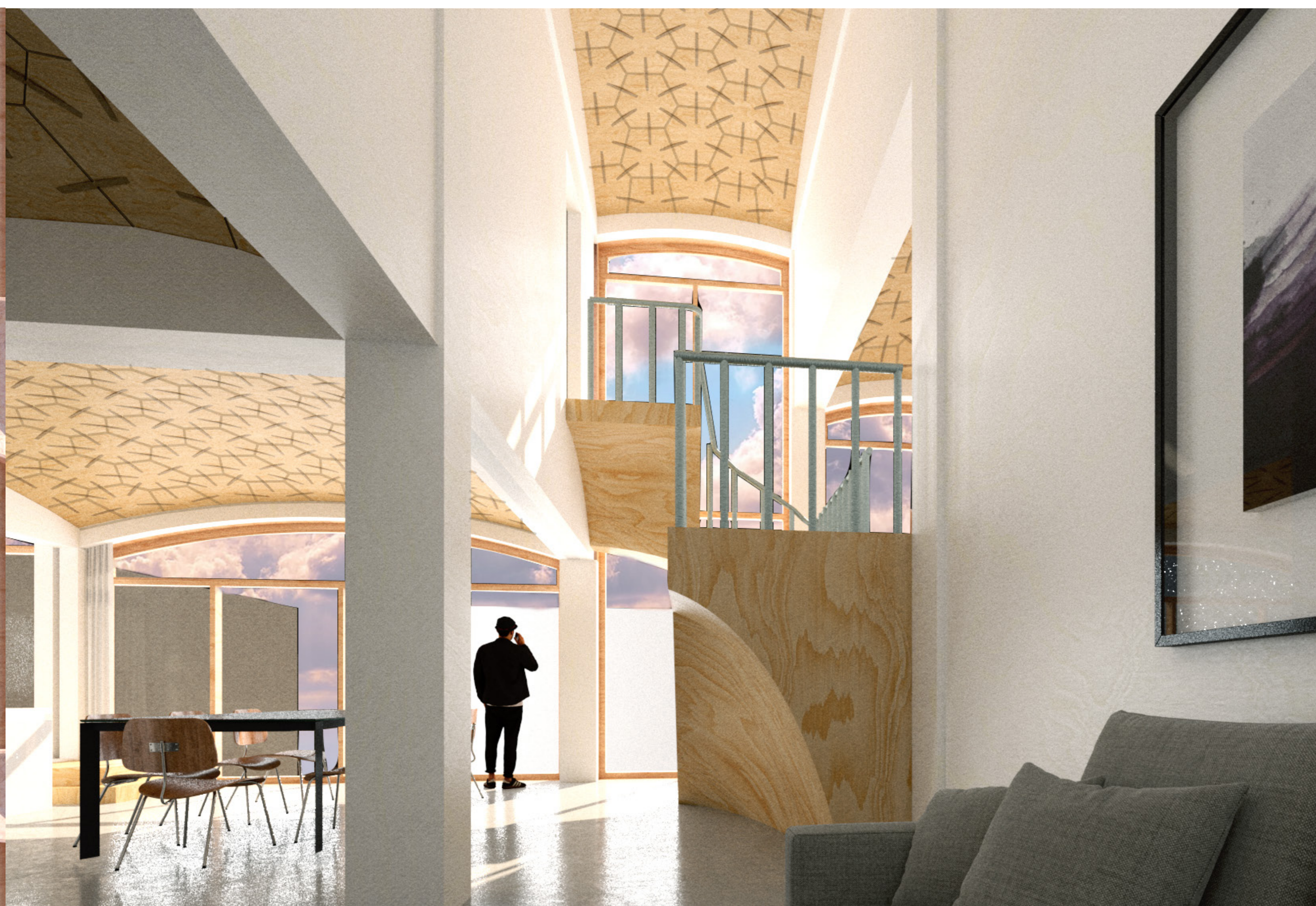
all parts are planar and can be cut out of a sheet of plywood using CNC-technology. (Studio RAP, 2016)
