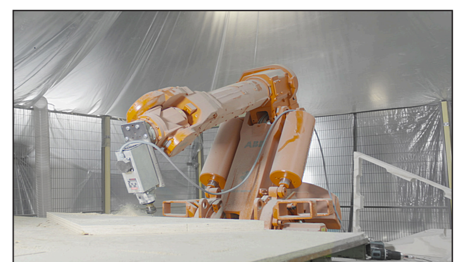
all parts are planar and can be cut out of a sheet of plywood using CNC-technology. (Studio RAP, 2016)
