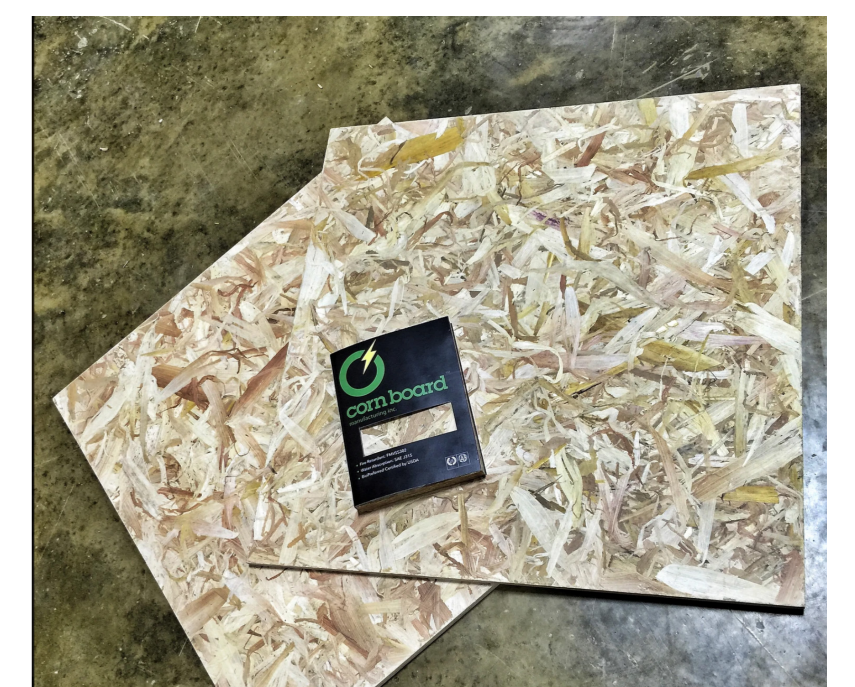
the facade panels are from bio composite made from compressed corn waste with natural resin.
