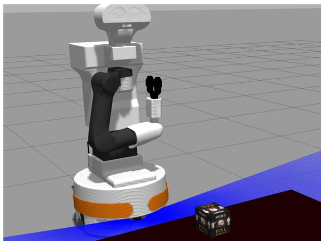
**Figure D.1:** A box with a texture on it for texture detection. The robot will try to detect the box pose by detecting the texture.
