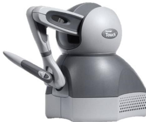
**Figure A.1:** Geomagic Touch device used to generate the demonstrations.
