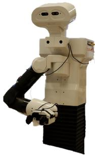
Fig. 10: Start configuration of the robot arm. The end-effector can easily rotate the yaw angle counter clockwise. It is hard to rotate it clockwise.
