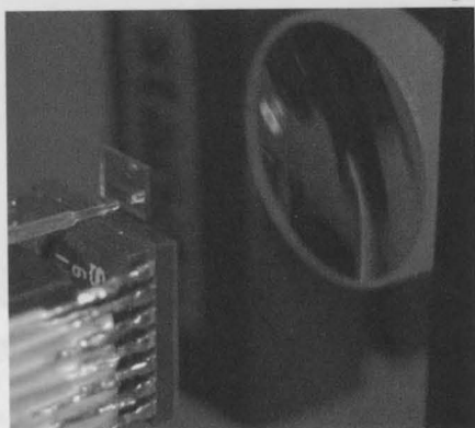
Fig. 6-15. Spectrometer chip aligned with a spherical mirror. Cleaved fiber tip visible in the left is used to illuminate the entrance slit of the spectrometer.
