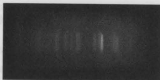
Fig. 4-22. Ne spectral pattern captured with the single grating spectrometer.
