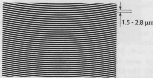
Fig. 4-17. Part of the lithography mask for the fabrication of a single grating spectrometer.
