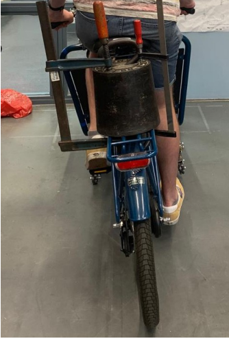
Fig. 11: Torque test with an 80-kilogram rider and 50 kilograms of weight on the luggage rack. The initial roll angle of the bicycle is 7.5 degrees.
