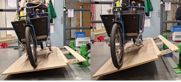
Fig. 13: Incline test with the system turned off on the left and the system turned on on the right.
