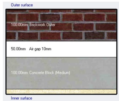
Figure A.10: Composition of External Walls
