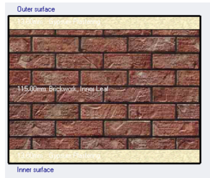
Figure A.12: Composition of Internal Partitions
