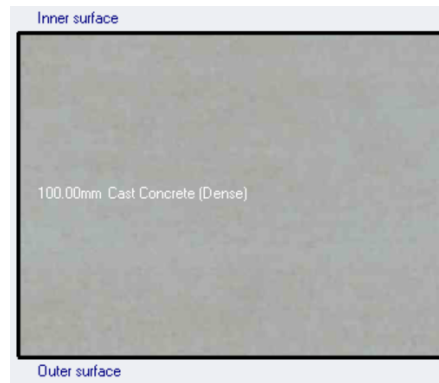
Figure 4.8: Composition of Internal Floor - Light Best Practice
