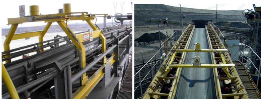
Fig. 6 Radiometric sensor measurement device, installed on the conveyor belt, measuring blend of coal resulting from multiple excavators, just before the stock pile
