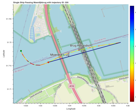
Figure 7.1: Trajectory plot with unrealistic data point, colour bar indicating vessel speed [m/s], Hollands Diep
