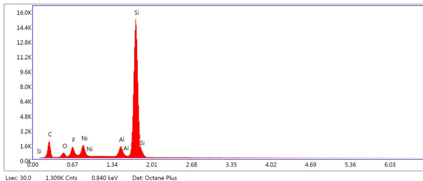
**Figure 4.12:** EDS analysis of SiC sample processed at pressure  $5.5E-2$  mbar. Nickel-coated silicon carriers were used.
