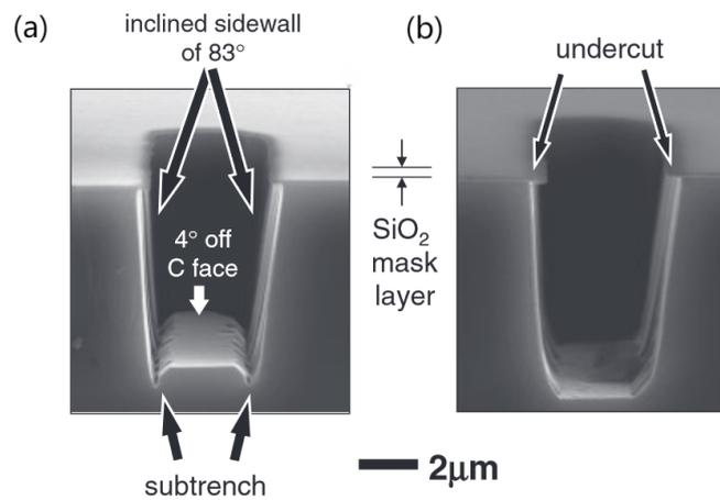
**Figure 2.15:** Etched 4H-SiC, (a) Before thermal  $Cl_2$  etching. (b) After 30 min thermal  $Cl_2$  etching[47].
