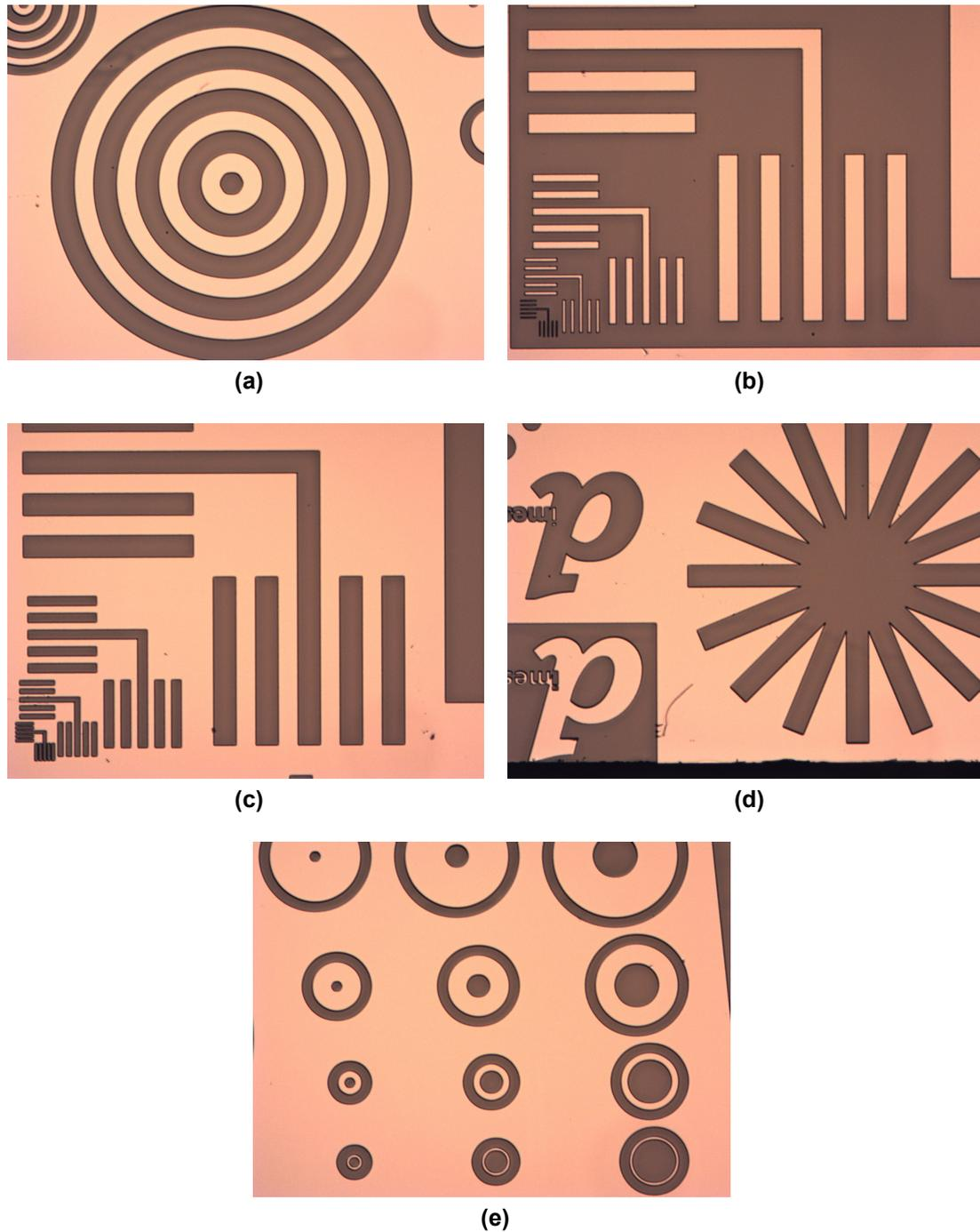
**Figure 3.11:** Microscope images of the etched 4H-SiC sample on an N-type silicon carrier wafer. Parameter settings in Table 3.5 apply.
