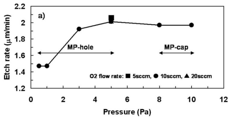
**Figure 2.11:** SiC Etch rate as a function of pressure in[40]
