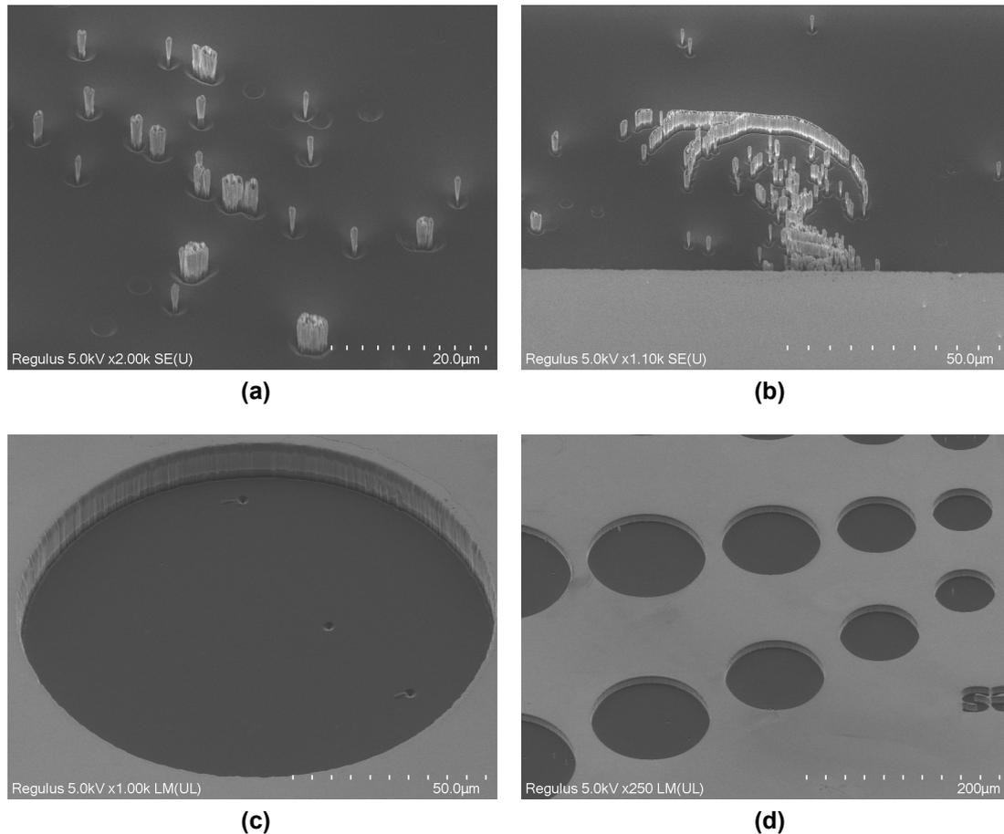
**Figure 3.7:** SEM images of the etched 4H-SiC sample with a pre-cleaning step by oxygen plasma. A sapphire carrier was used.
