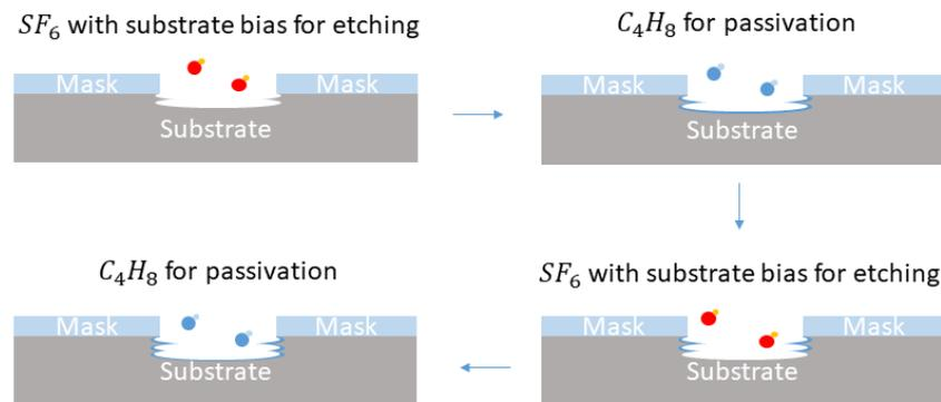
**Figure 2.1:** Illustration of the Bosch process mechanism for silicon etching
