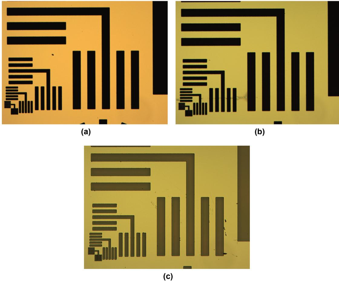
**Figure 4.10:** Microscope figures at pressure:(a) $4.5E-2$  mbar.(b) $5.5E-2$  mbar.(c) $1.5E-2$  mbar. Nickel-coated silicon carriers were used.
