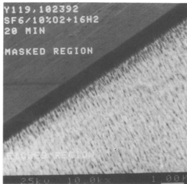
**Figure 2.3:** Micro maskings induced by aluminum hard mask[34]
