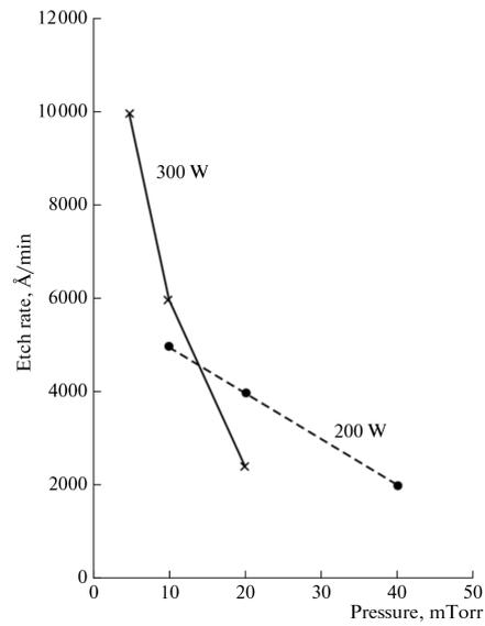
**Figure 2.10:** SiC Etch rate as a function of pressure at 200 W and 300 W chuck bias power, adapted from[39]
