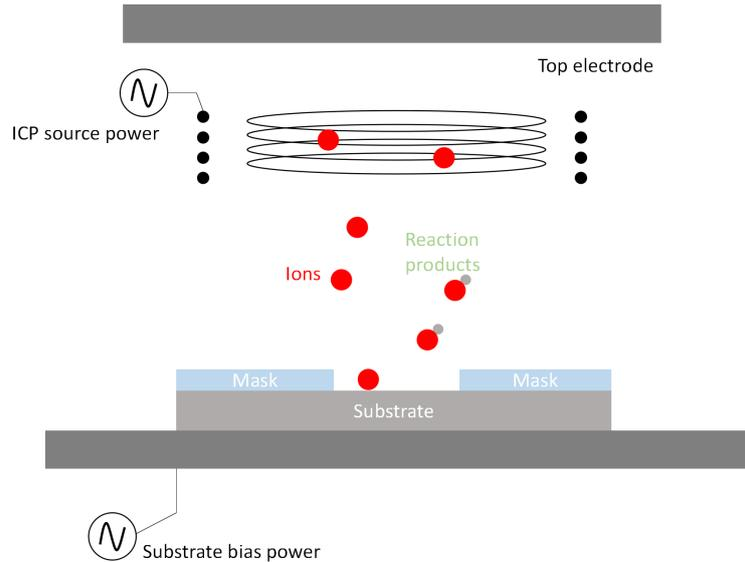
**Figure 1.3:** Illustration of ICP RIE process mechanism
