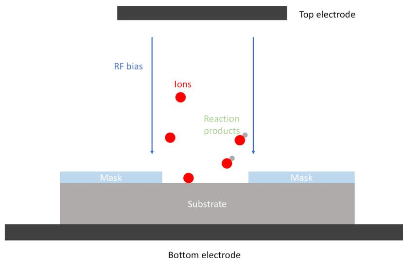
**Figure 1.2:** Illustration of RIE process mechanism
