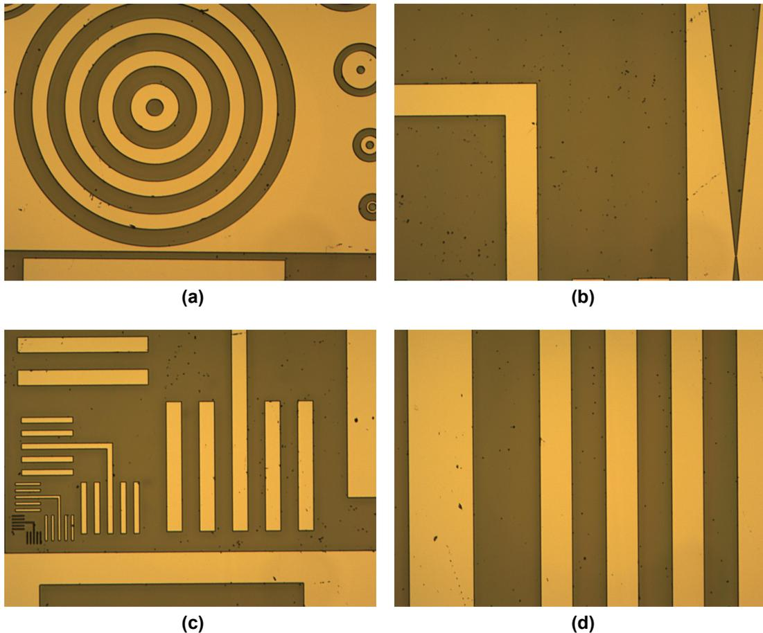
**Figure 3.10:** Microscope images of the etched 4H-SiC sample on a P-type silicon carrier wafer. Parameter settings in Table 3.5 apply.
