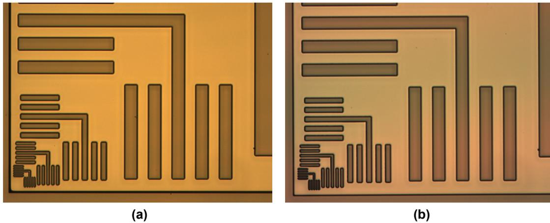
**Figure 4.22:** Microscope figures at substrate temperature:(a)-120 °C.(b)20 °C. Silicon carriers were used.
