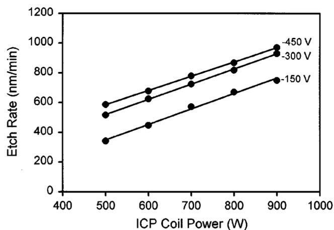
**Figure 2.5:** Etch rate as a function of ICP coil power in [37]
