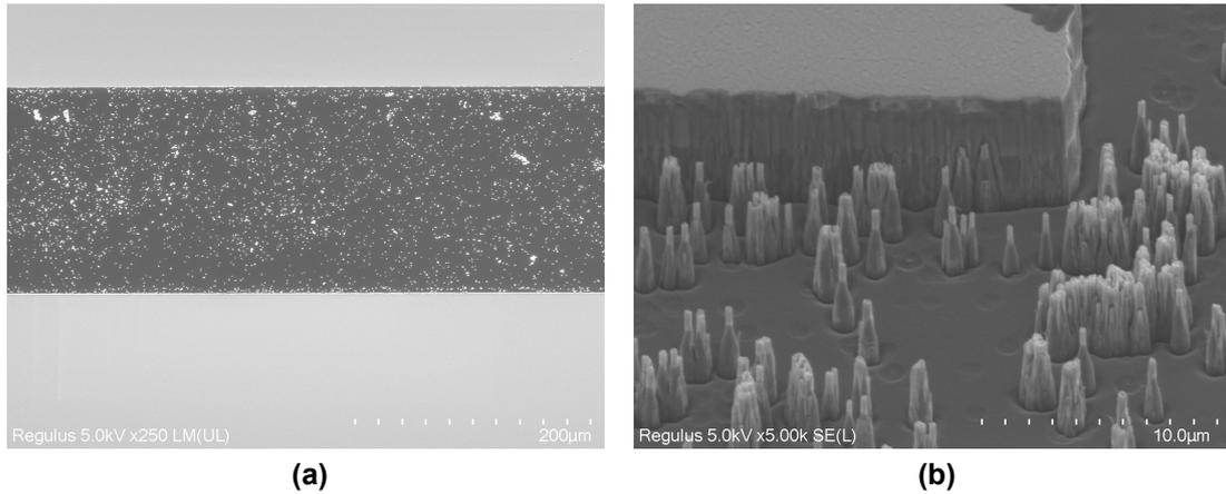
**Figure 3.5:** SEM images of the etched 4H-SiC sample with a pre-cleaning step by argon plasma, a sapphire carrier was used.
