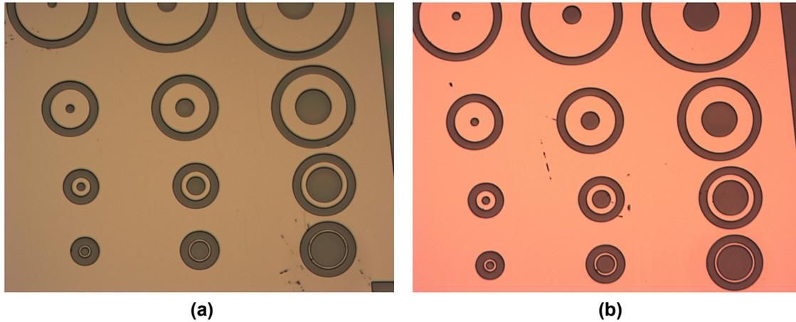
**Figure 4.8:** Microscope figures at ICP source power:(a)2000W(minimum setting).(b)2500W(maximum setting)
