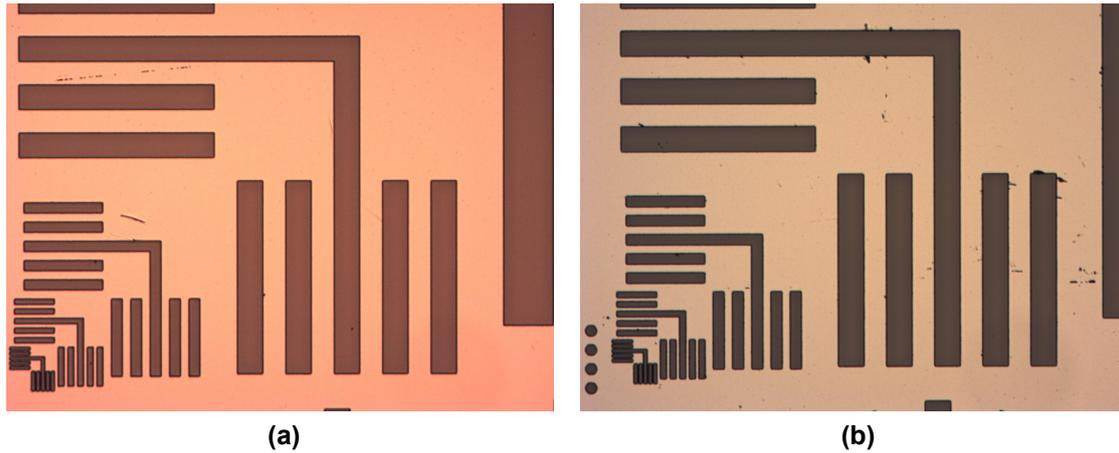
**Figure 4.4:** Microscope figures at chuck bias power:(a)100 W(minimum setting).(b)300 W(maximum setting).
