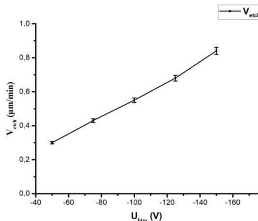
**Figure 2.7:** SiC etch rate as a function of chuck bias power in [38]
