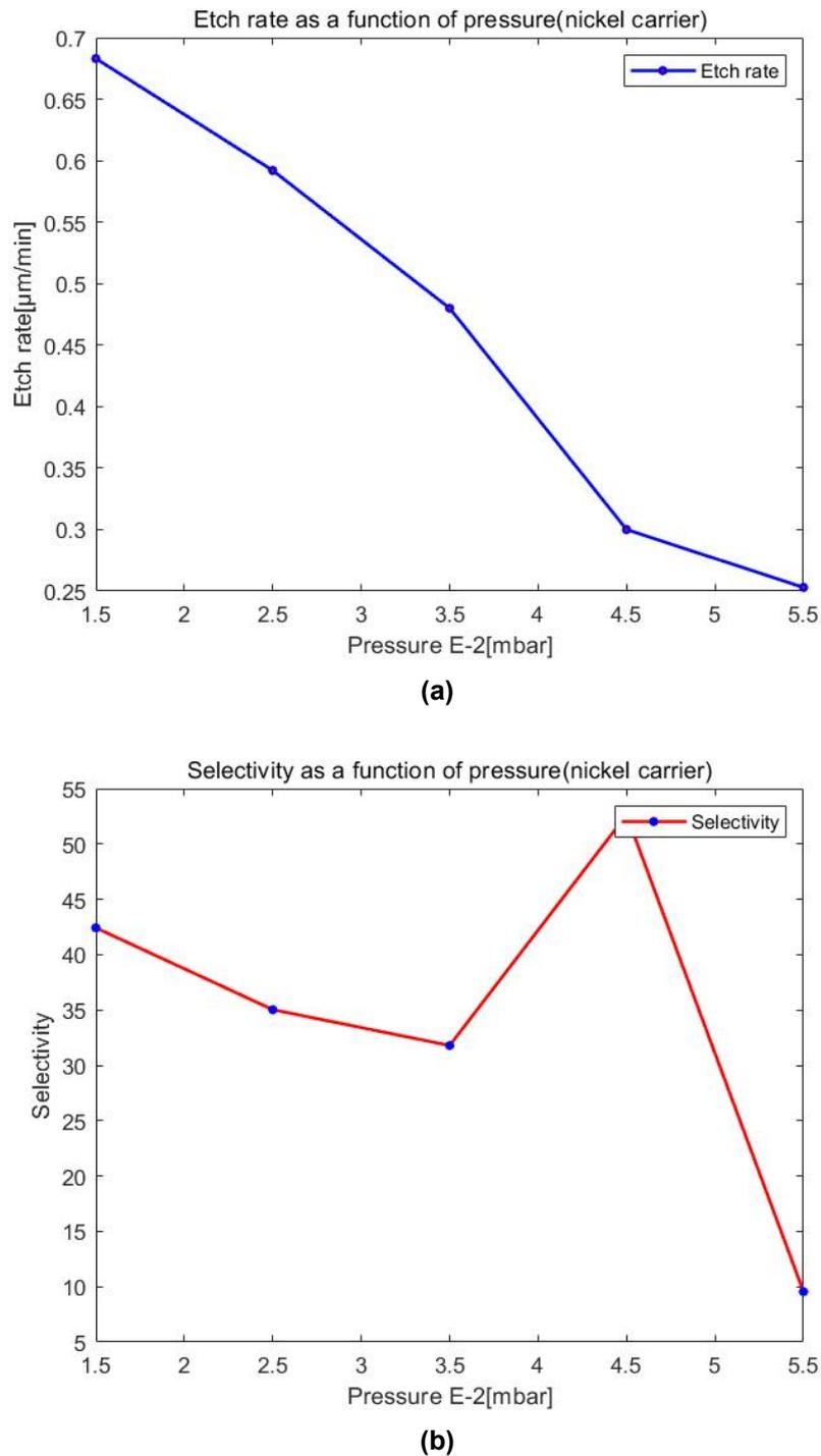
**Figure 4.9:** Role of pressure:(a)Etch rate as a function of pressure. (b)Selectivity as a function of pressure. Nickel-coated silicon carriers were used.
