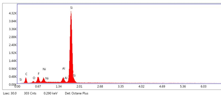
**Figure 4.15:** SEM figure of the cross-section and EDS analysis for SiC samples processed at 100W chuck bias power:(a)SEM image.(b)EDS analysis. Nickel-coated silicon carriers were used.
