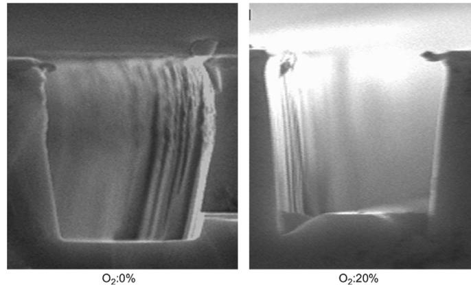
**Figure 2.16:** Etched 4H-SiC, with 0% O<sub>2</sub> and with 20% O<sub>2</sub>[48].
