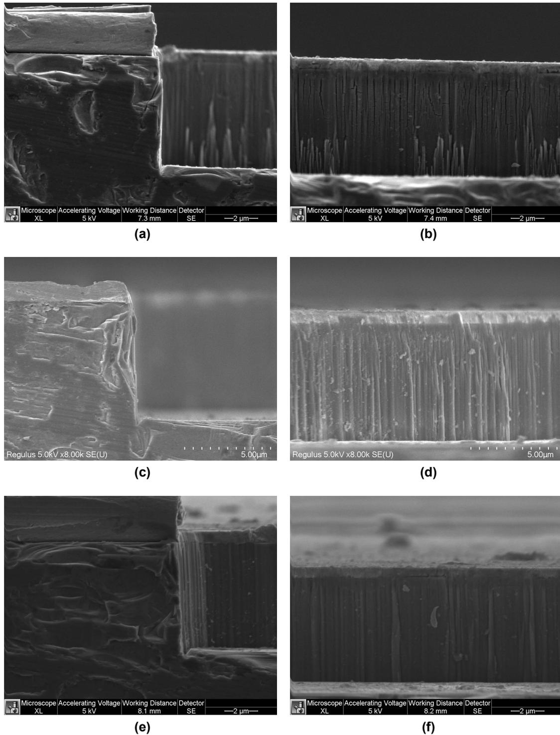
**Figure 4.17:** SEM figures of the cross-section. (a) and (b): 10 °C. (c) and (d): 20 °C. (e) and (f): 40 °C. Nickel-coated carriers were used.
