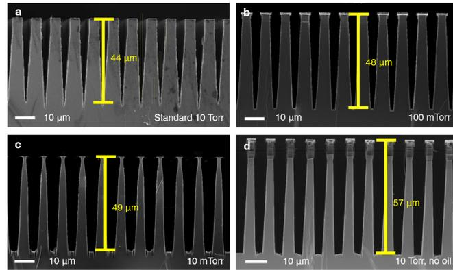
**Figure 2.2:** Etch profile of 4H-SiC after 2-hour etch in SF<sub>6</sub>/O<sub>2</sub> etch gas[13]
