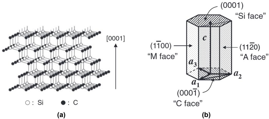
**Figure 1.1:** (a) Schematic crystal structure of 4H-SiC. (b) Hexagonal cell of SiC. [4]
