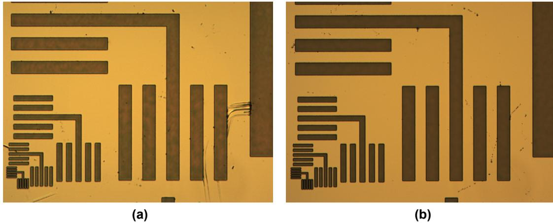
**Figure 4.19:** Microscope figures at ICP source power:(a)2000W.(b)2800W. Nickel-coated silicon carriers were used.
