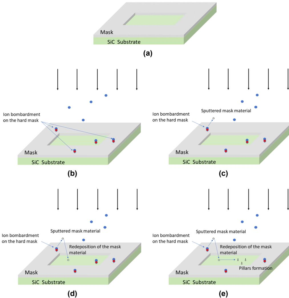
**Figure 2.13:** Micro masking effect mechanism
