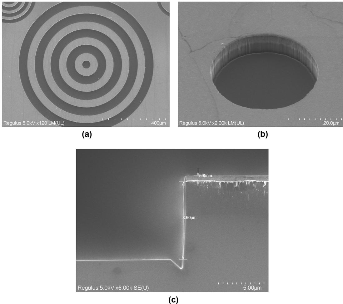
**Figure 3.9:** SEM images of the etched 4H-SiC sample on a P-type silicon carrier wafer:(a)Top view.(b)45 degree tilt.(c)Cross section
