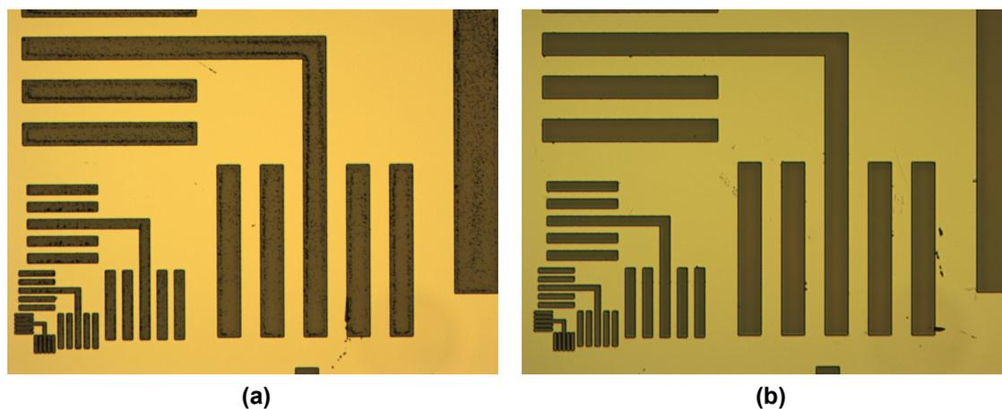
**Figure 4.14:** Microscope figures at chuck bias power:(a)100W.(b)300W. Nickel-coated silicon carriers were used.
