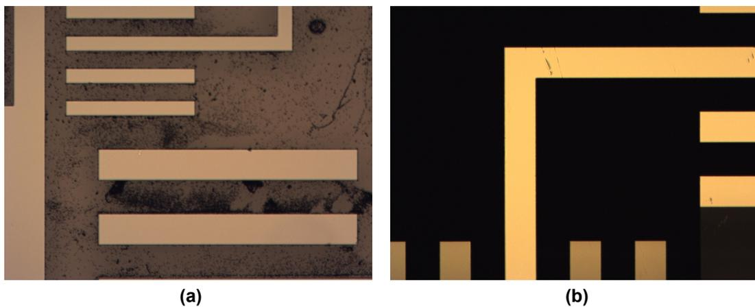
**Figure 3.6:** Microscope images of the etched 4H-SiC sample:(a)with a pre-cleaning step by argon plasma.(b)without a pre-cleaning step by argon plasma. A Sapphire carrier was used.
