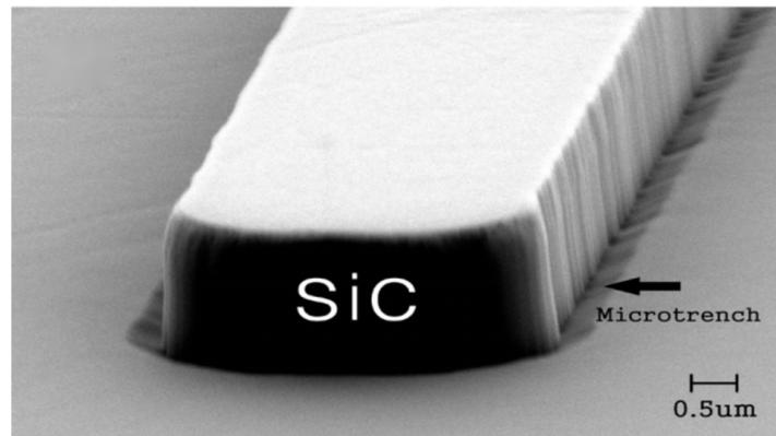
**Figure 2.14:** Micro trenches found at the bottom of the etched SiC structure with  $O_2$  plasma applied during the etching[44]
