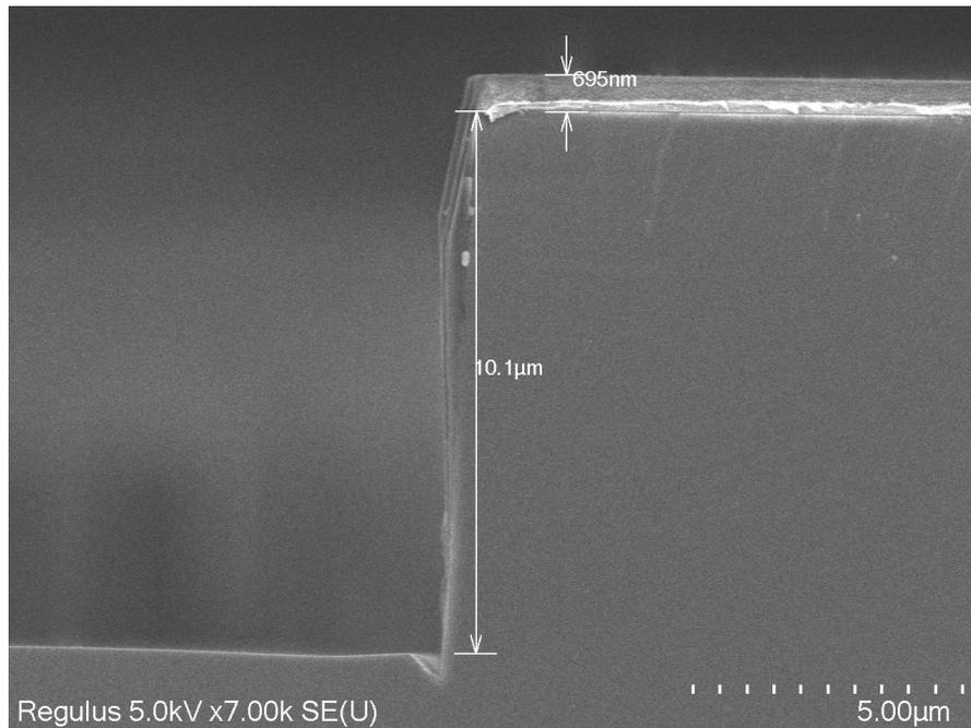
**Figure 3.8:** SEM image of the cross-section of the etched 4H-SiC after preliminary optimization
