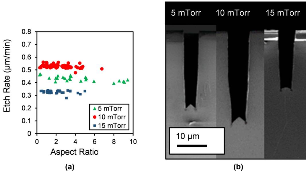
**Figure 2.9:** SiC Etch rate at different pressure[15]
