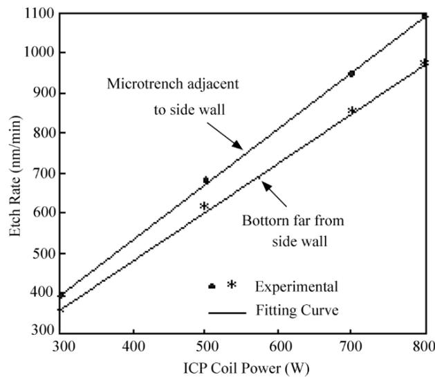
**Figure 2.4:** Etch rate as a function of ICP coil power in [35]
