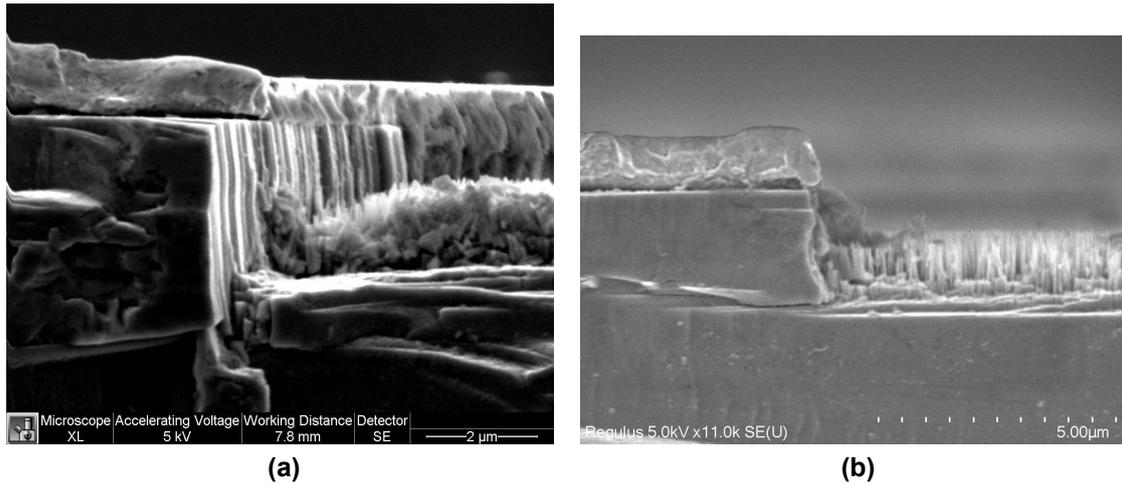
**Figure 4.11:** SEM figures of cross sections at pressure: (a)  $4.5E-2$  mbar. (b)  $5.5E-2$  mbar. Nickel-coated silicon carriers were used.
