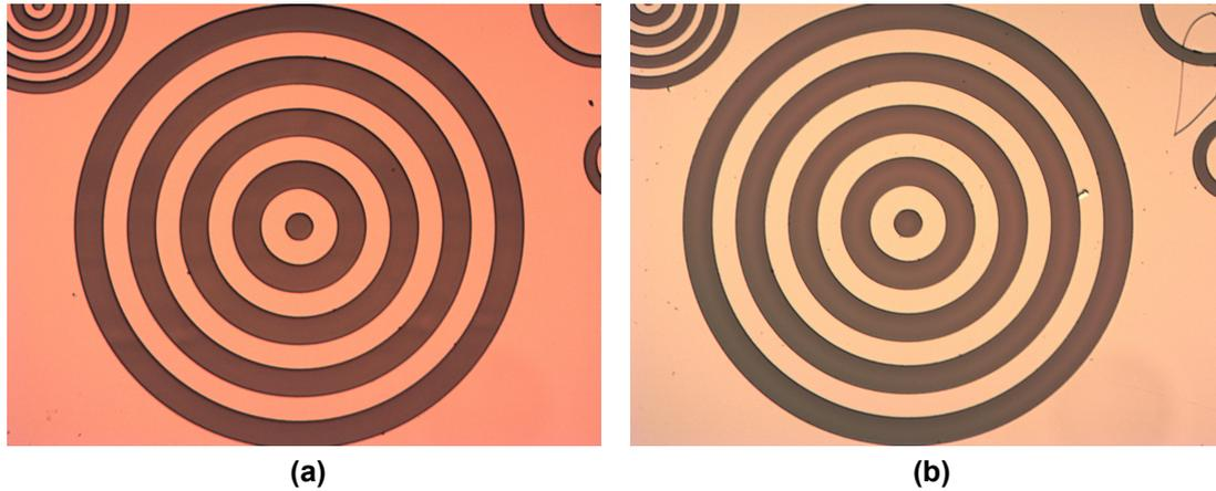
**Figure 4.2:** Microscope figures at pressure:(a)1.5 E-2 mbar(minimum setting).(b)5.5 E-2 mbar(maximum setting).
