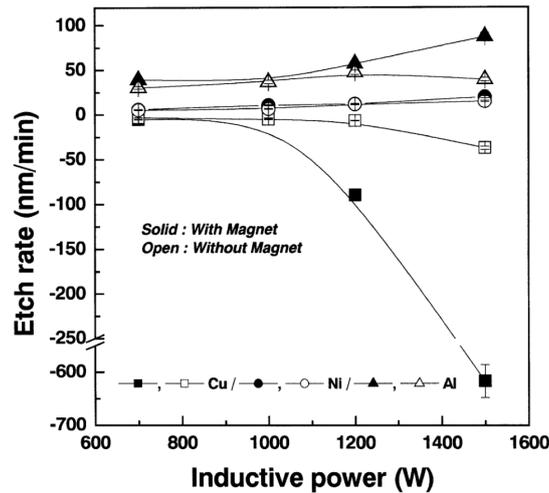
**Figure 3.1:** Etch rates of copper, nickel, and aluminum as a function of inductive power with and without magnetic field, at powers higher than 1200 W, deposition instead of etching of copper occurred[49].
