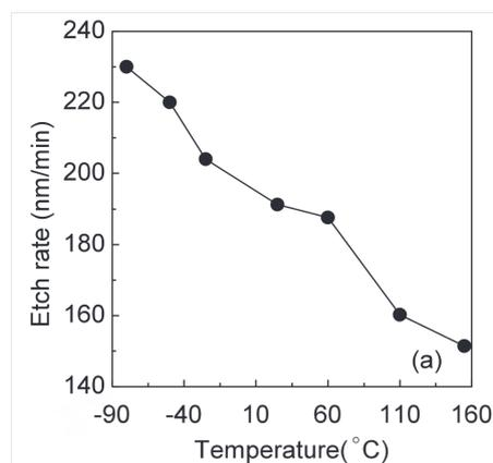
**Figure 2.12:** SiC Etch rate with  $\text{Cl}_2$  and Ar as a function of temperature[25]
