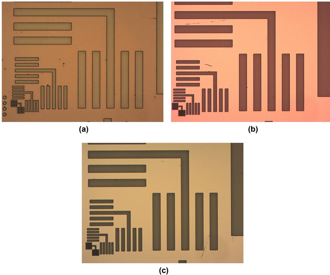
**Figure 4.6:** Microscope figures at substrate temperature:(a)10 °C(minimum setting).(b)20 °C.(c)40 °C(maximum setting)
