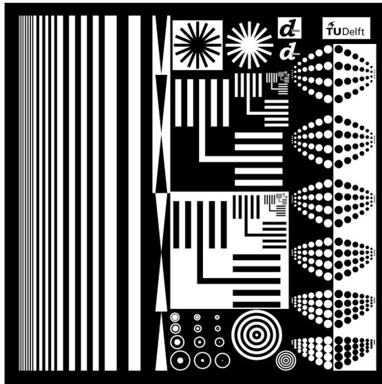
**Figure 3.2:** The mask used for patterning the substrate, provided by EKL
