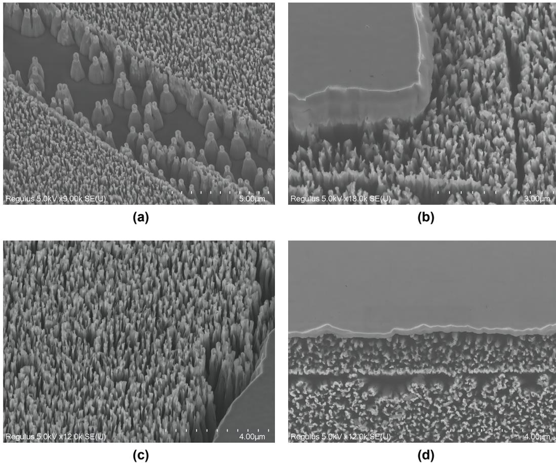
**Figure 3.3:** SEM images of the SiC structure after the initial test, a sapphire carrier was used. Parameters in Table 3.2 were applied
