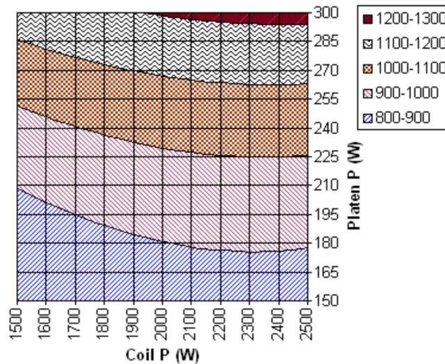
**Figure 2.6:** Contour plot of SiC etch rate as a function of ICP coil power and chuck bias power in [36], the nominal etch rate is  $1 \mu\text{m}/\text{min}$
