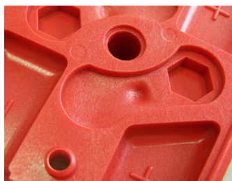
Figure 1.1: An example of a surface sink mark, an indentation of the surface of an object made with injection molding, source [2].
