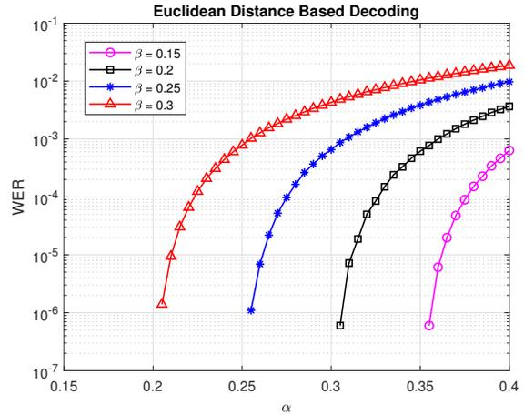
Fig. 1. Simulated WER of Euclidean distance-based decoding for codebook  $\mathcal{S}^*$  on channels with uniform noise  $v_i \sim \mathcal{U}(-\alpha, \alpha)$  and uniform offset  $b \sim \mathcal{U}(-\beta, \beta)$ .
