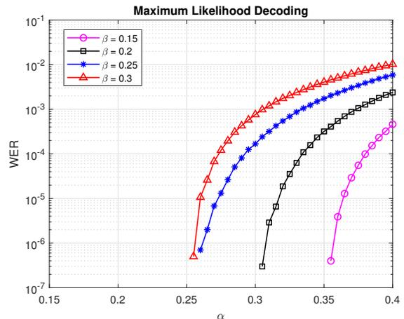
Fig. 3. Simulated WER of ML decoding for codebook  $\mathcal{S}^*$  on channels with uniform noise  $v_i \sim \mathcal{U}(-\alpha, \alpha)$  and uniform offset  $b \sim \mathcal{U}(-\beta, \beta)$ .
