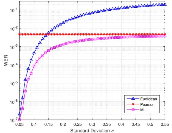
Fig. 6. Simulated WER for codebook  $\mathcal{S}^*$  on channels with uniform noise  $v_i \sim \mathcal{U}(-0.3, 0.3)$  and Gaussian offset  $b \sim \mathcal{N}(0, \sigma^2)$ .
