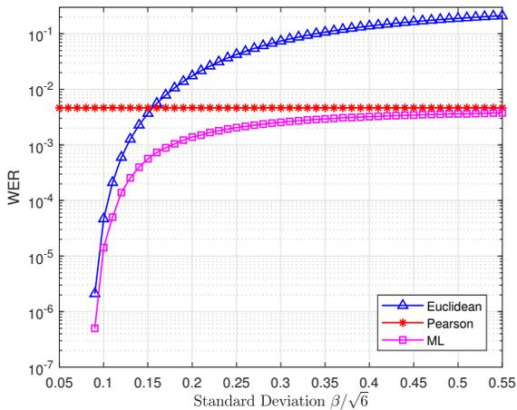
Fig. 5. Simulated WER for codebook  $\mathcal{S}^*$  on channels with uniform noise  $v_i \sim \mathcal{U}(-0.3, 0.3)$  and triangular offset  $b \sim \mathcal{T}(-\beta, 0, \beta)$ .
