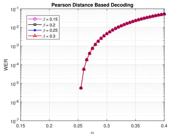
Fig. 2. Simulated WER of Pearson distance-based decoding for codebook  $\mathcal{S}^*$  on channels with uniform noise  $v_i \sim \mathcal{U}(-\alpha, \alpha)$  and uniform offset  $b \sim \mathcal{U}(-\beta, \beta)$ .
