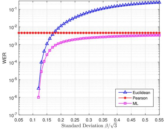
Fig. 4. Simulated WER for codebook  $\mathcal{S}^*$  on channels with uniform noise  $v_i \sim \mathcal{U}(-0.3, 0.3)$  and uniform offset  $b \sim \mathcal{U}(-\beta, \beta)$ .
