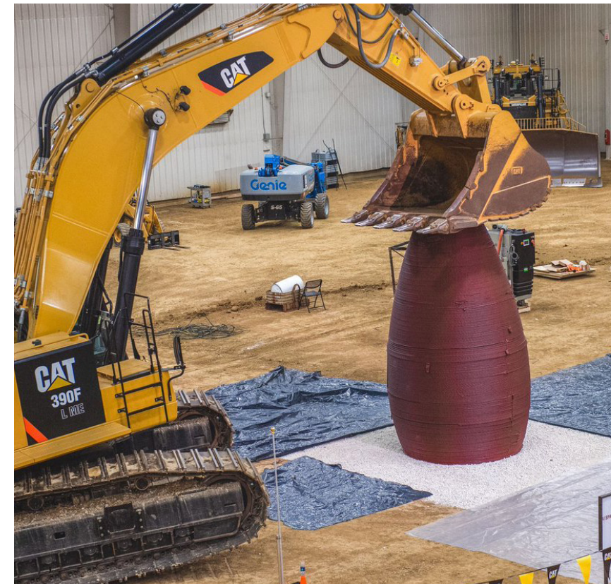
3D Printed BFRPLA: structure stays intact under load, does not collapse
