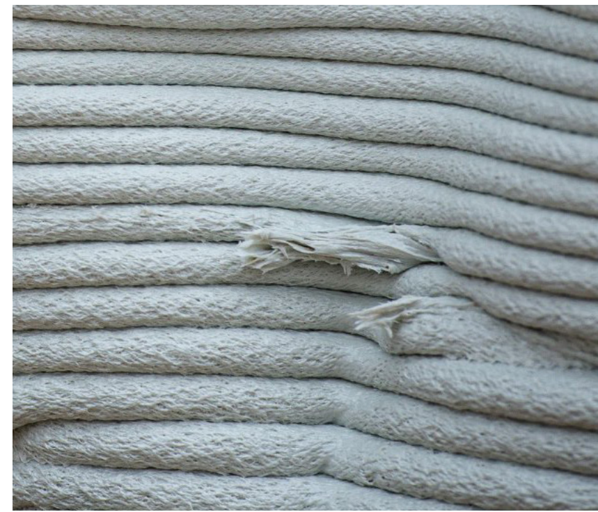
Textured surface 3D printed BFRPLA: good sound absorption
