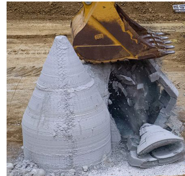
3D Concrete: Collapses under less pressure than BFRPLA
