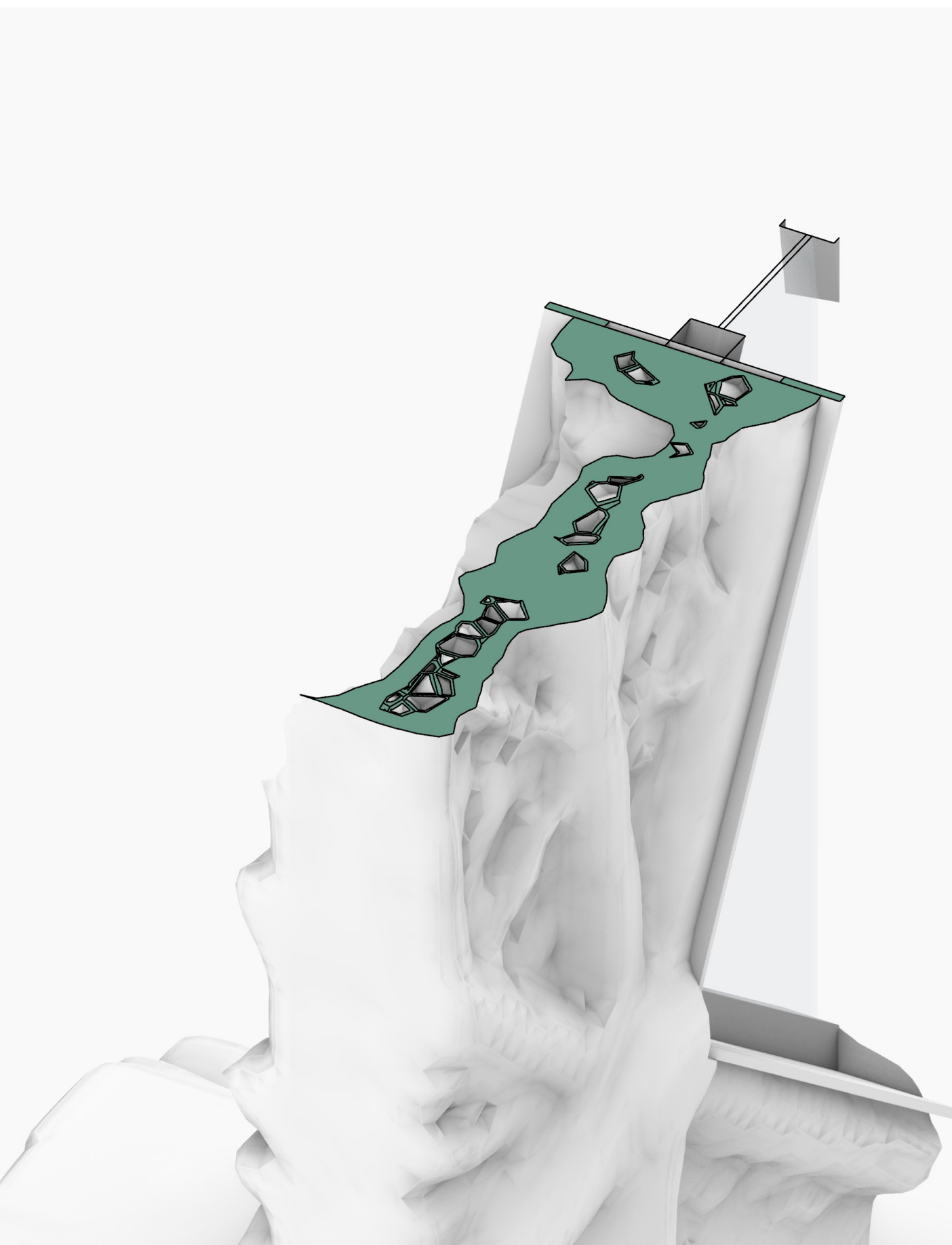
3D print wall until support floor + incorporate a thread insert in the 3D print
