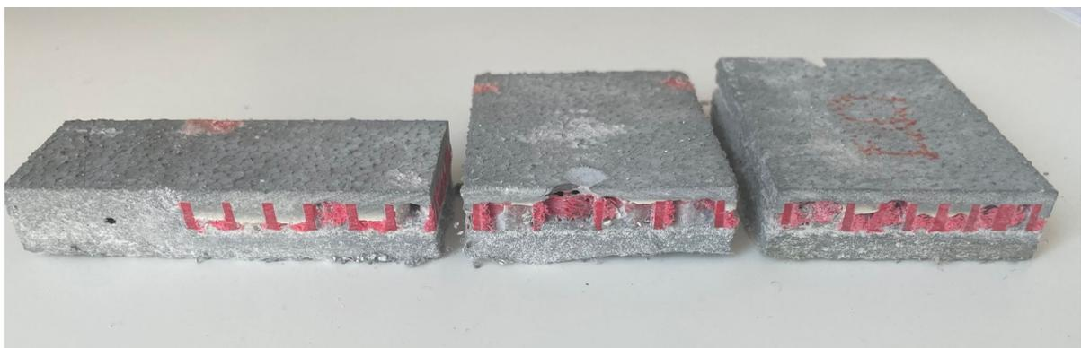
**Figure C.3:** Air void in Sample B-ABS
