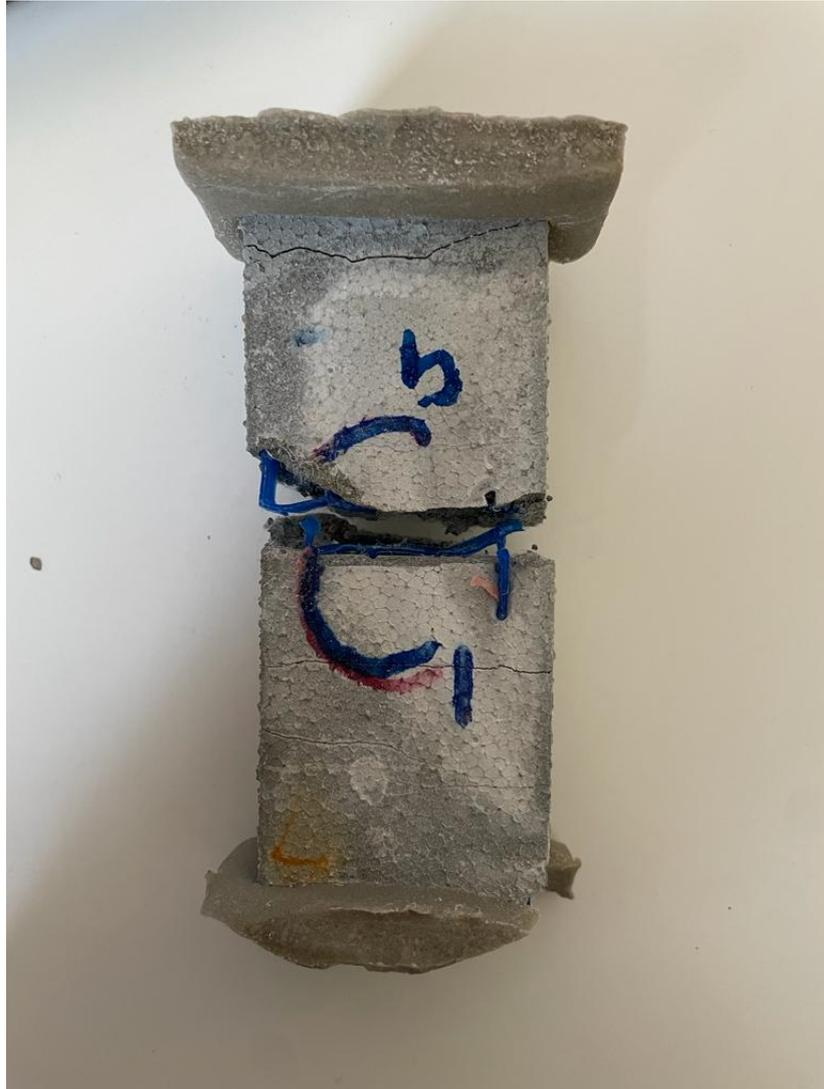
**Figure C.2:** Sample C<sub>1</sub>-TPU backside showing multiple cracks
