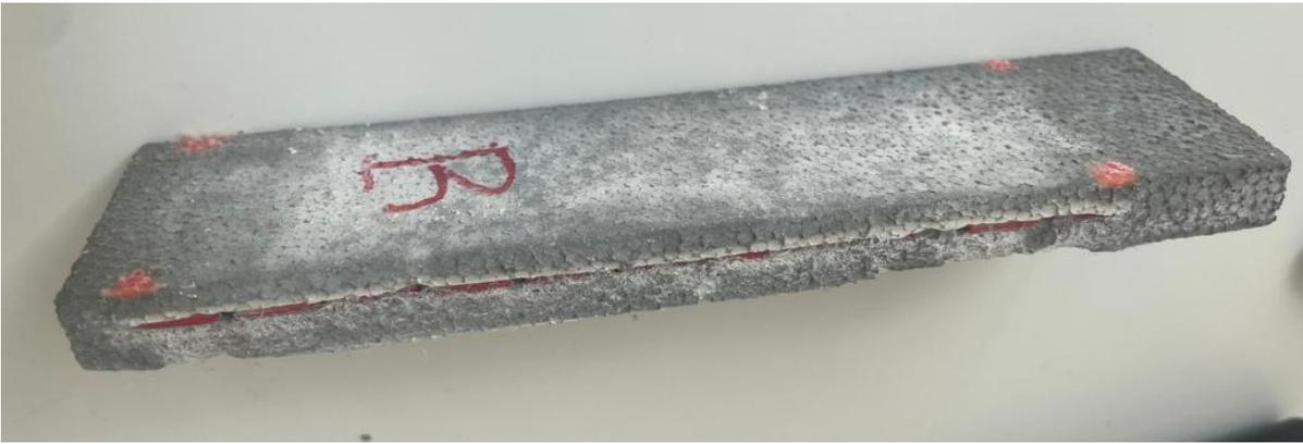
**Figure C.4:** Sample B casting complications
