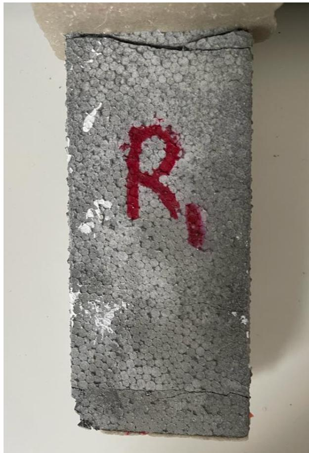
**Figure C.1:** Sample R<sub>1</sub> backside showing multiple cracks
