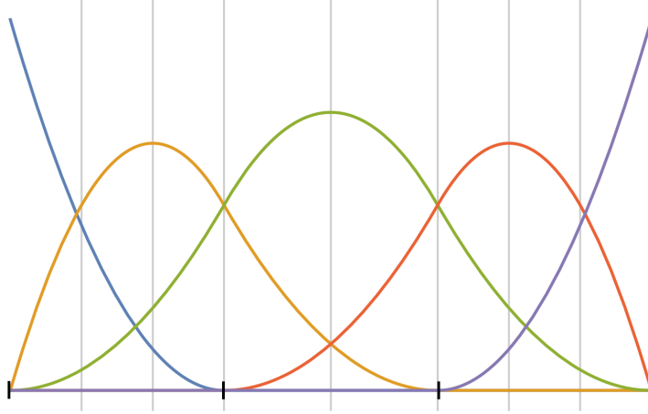
Figure 4.1: Basis functions of degree 2 for an open knot vector with three elements.
