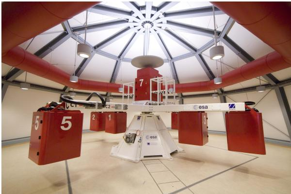
**Figure 4.1:** The Large Diameter Centrifuge at ESTEC (Photo: ©ESA)
