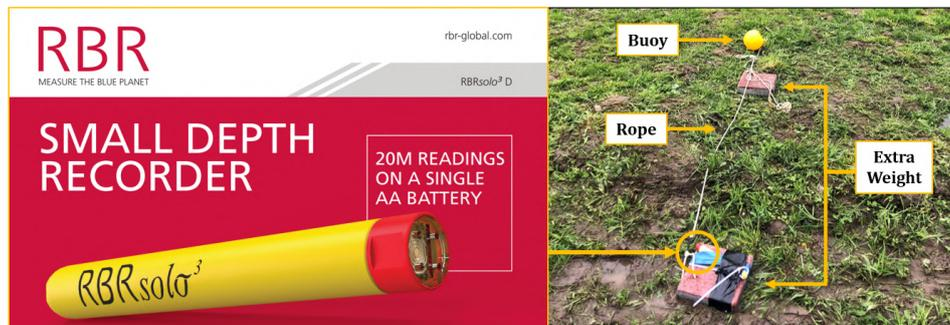
Figure 3.4: RBRsolo<sup>3</sup> logger information [34] and setup
