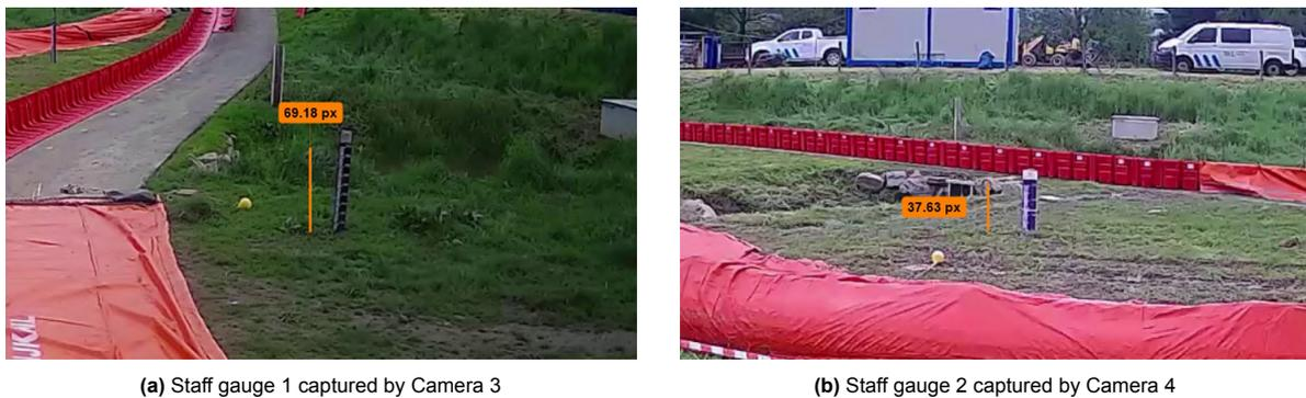
**Figure 3.12:** Pixel distance calculated by Kinovea — Water Level Measurement
