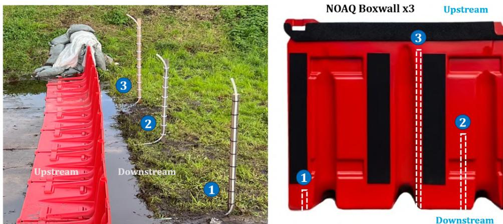
**Figure 4.9:** Position of the corresponding pitot tubes
