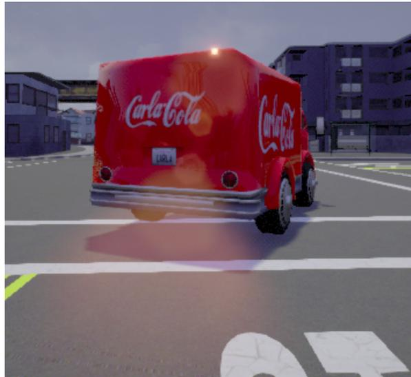
Figure 5.1: Example image of CARLA simulation that illustrates the realistic lighting and reflection physics of the simulator. These are important aspects for ORB SLAM which rely on pixel intensity to provide a pose estimations.
