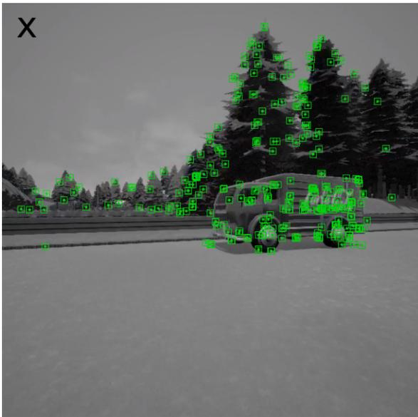
(b) Source of the large error peak at  $t = 45$  seconds. Many features describe the opposed moving vehicle which cause an error in the pose estimation, since the algorithm assumes matched features are static.
