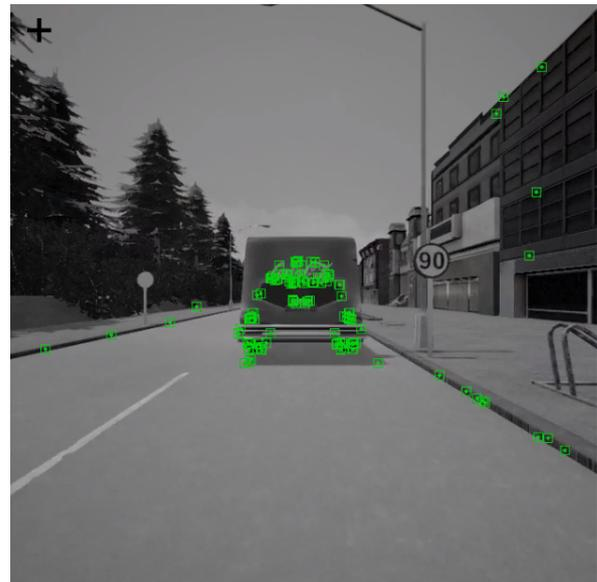
(c) Image of ORB SLAM in town 1 trajectory 1 with an inter-vehicle distance of 10 meters. Illustration of ORB features locking onto the vehicle in front and therefore expecting the ego-vehicle to stand still.
