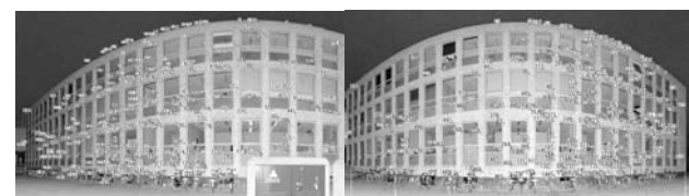
Fig.6 Evenly distributed corresponding points on building façade
