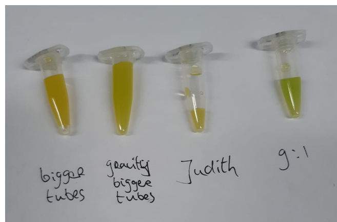
Figure 38. Left 3 tubes as a result of parallel flow, right tube with food colouring's mixed in the 9:1 ratio.
