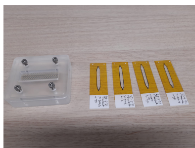
Figure 54. The stencil maker (left) is screwed on the bottom part of the flow chamber.
