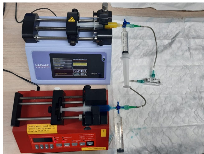
Figure 40. Set-up with food colouring's and mixing part.
