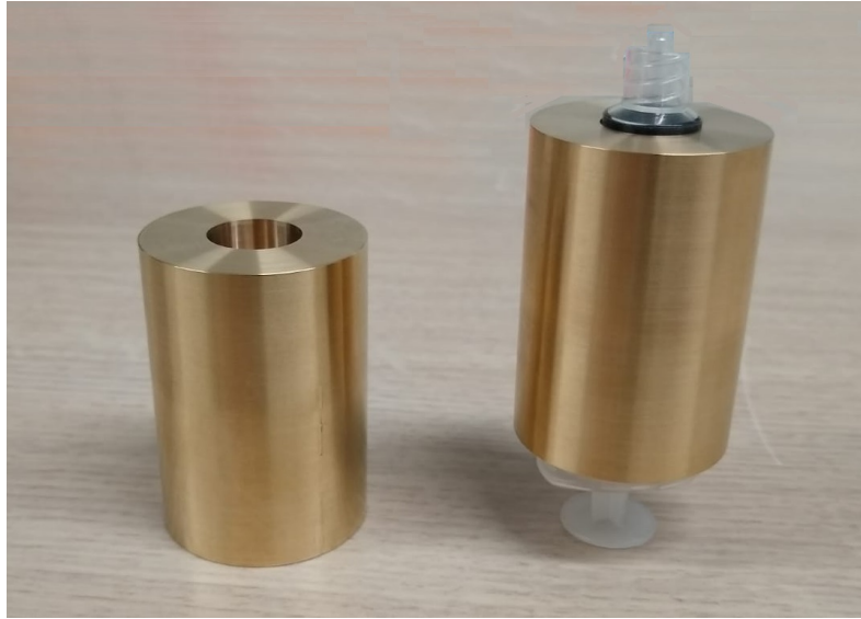
Figure 3. Cylindrical shell weights which mimicked blood pressure in a static way.
