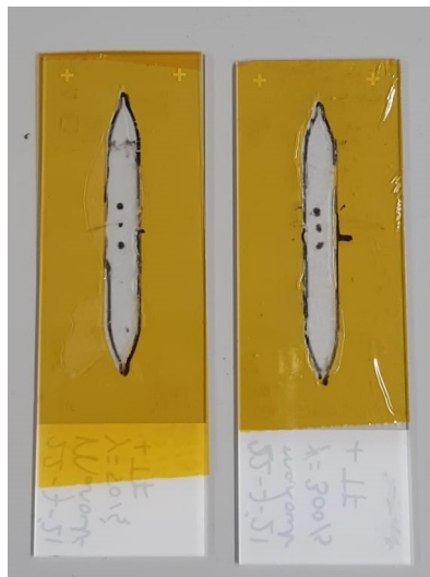
Figure 53. The microscopic glass, marked, and with the cut out shape of the flow channel, with solid buffer on it.
