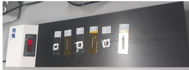
Figure 49. Microscopic glass slide temperature generator, with TF coated slides.
