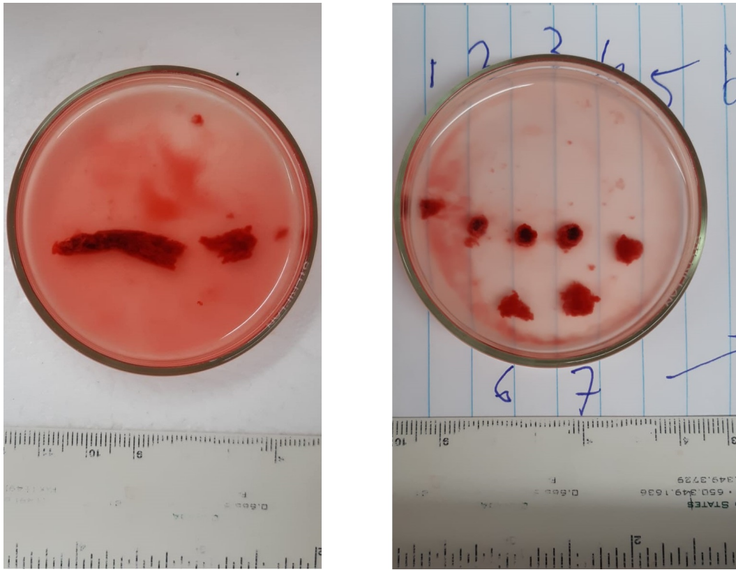
Figure 43. The resulting clot, one can see a bigger part on the left and a small part on the right which was ruptured in the tubing. The resulting clot cut in 3 mm high pieces, the top row is the big clot, the bottom row is the small part.
