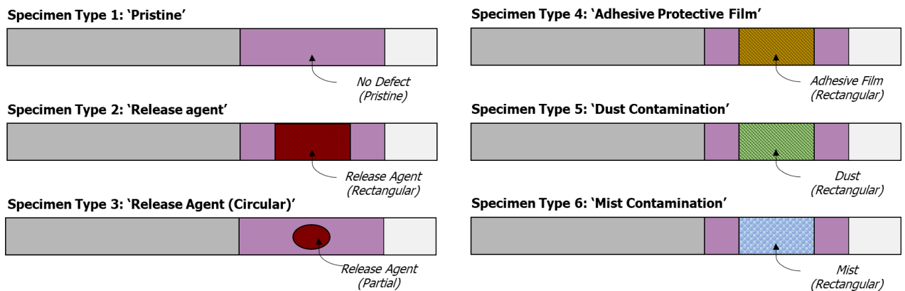
Figure 20: Specimen Defect Types
