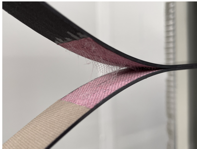
Figure 102: Bridging of Adhesive Carrier fibers
