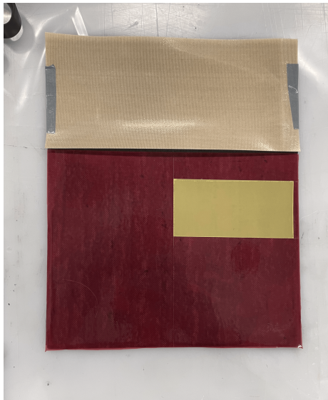
Figure 34: Adhesive Carrier Film remaining on the adherend surface
