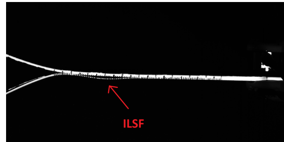
(b) Inter-Laminar Failure RA-U3. Occurring at Crosshead-displacement 43 [mm]
