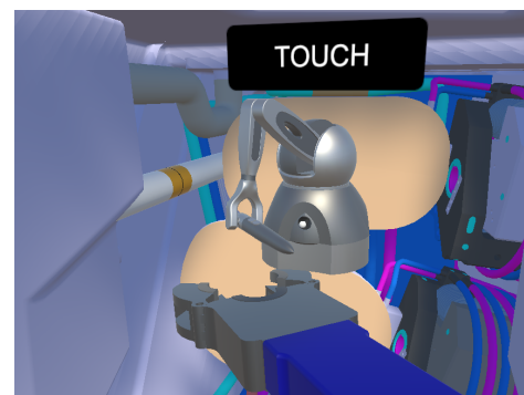
Fig. 4. Image of the virtual Touch. The virtual Touch appears above the welding tool when the human-operator is re-indexing (i.e. clutching) to show the configuration of the physical Touch haptic device.
