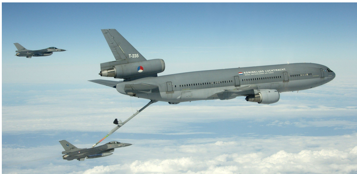
Figure 1.2: A KDC-10 tanker aircraft of the Royal Netherlands Air Force aerial refuels an F-16 fighter jet [17]
