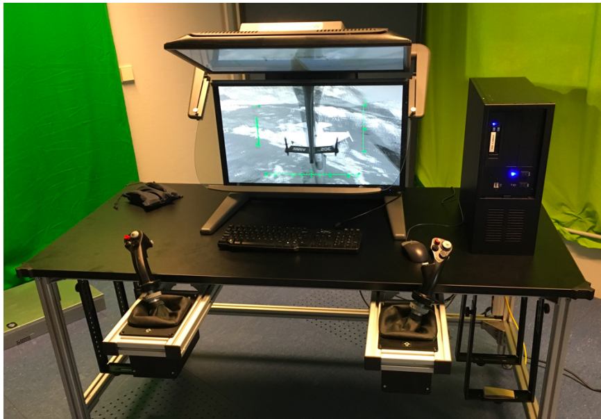
Figure 2: The TRVS AAR simulator loaded with the second task on aerial refuelling. During the experiments, the left side-stick will be removed to avoid confusion of input possibilities
