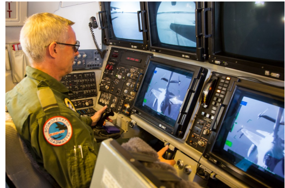
Figure 1.1: A Royal Netherlands Air Force aerial refueling boom operator using a stereoscopic three-dimensional display as a remote vision interface [10]
