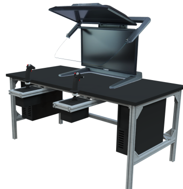
Fig. 5: An illustration of the 3D Aerial Refueling Simulator developed by multiSIM Ltd. used as a measurement setup for acquisition of human-in-the-loop experimental data.
