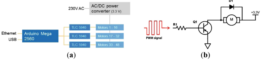
Fig. 2. (a) Functional diagram of the vibrotactile seat. Orange lines represent digital connections, whereas grey lines are power connections. (b) Electrical circuit of a single vibration motor that is PWM-controlled
