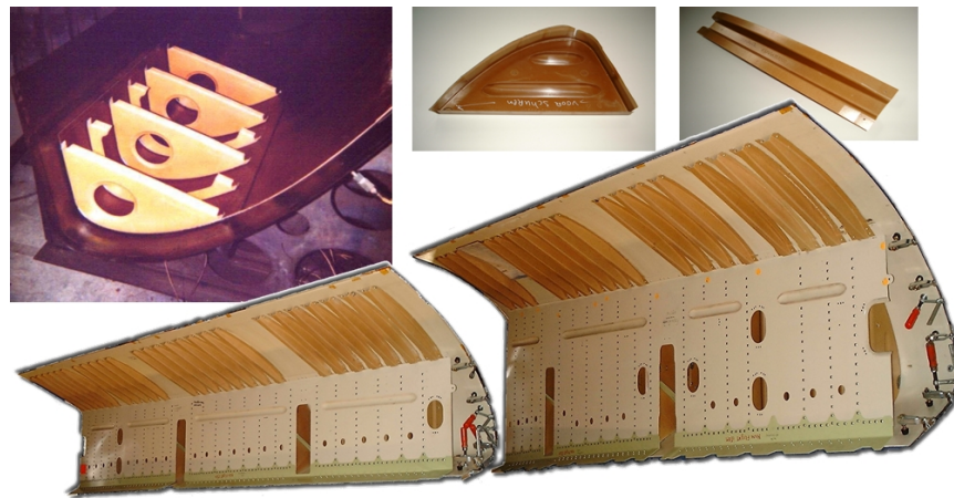
Fig. 1.9: Airbus A350 inboard leading edge or 'J-Nose', manufactured by Stork Aerospace, The Netherlands.
