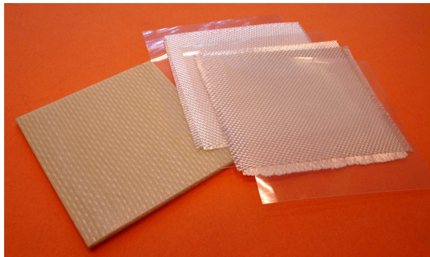
Fig. 1.6: Thermoplastic composite intermediate materials. Left: pre-consolidated laminate sheet material, right: a stack of alternating layers of polymer films and woven fiber reinforcement.
