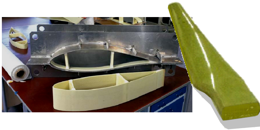
Fig. 1.10: Thermoplastic composite blade parts manufactured at the Risø National Laboratory in Denmark. Left: cross-section made of glass/PP [24], right: small blade made of glass/PET [25].
