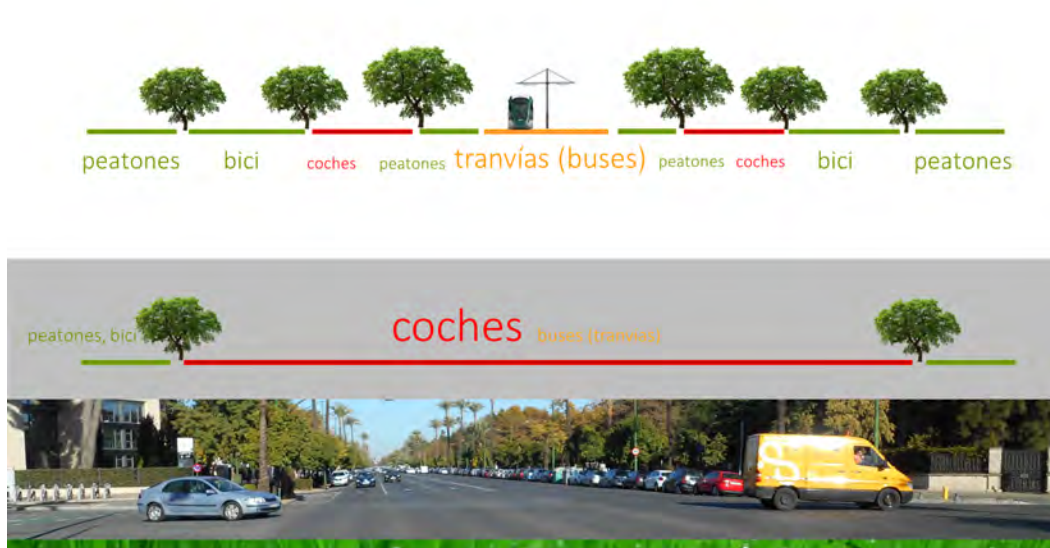
Fig. 26. Swapping the mobility system towards sustainable modes, example for Avenida de la Palmera. Above: proposed scheme, under: actual situation.
