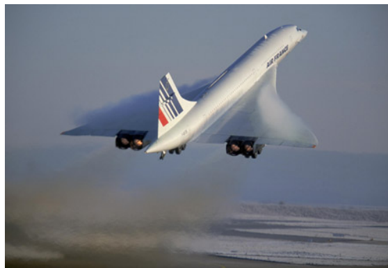
(b) Concorde at take off. Notice the condensation in the vortex above the wing. (©The Global Aircraft Organisation)
