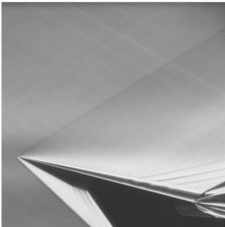
Figure 5.3: Schlieren image at \alpha = 15^\circ and M_\infty = 2.0 .
