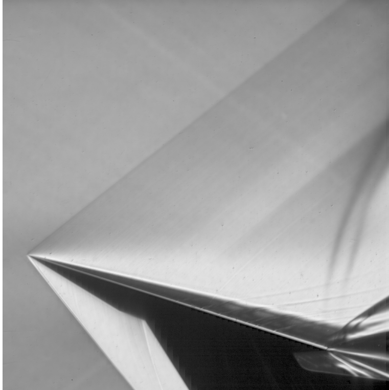
Figure 5.4: Schlieren image at \alpha = 18^\circ and M_\infty = 1.7 .
