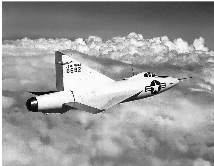
Figure 1.1: The XF-92A research aircraft which was one of the first aircraft to incorporate delta wings in its design (©NASA).
