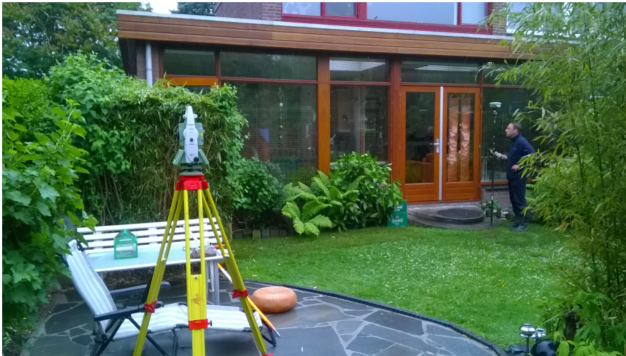
Figure 3.7: A tachymeter with a prism (photo taken by the author)
