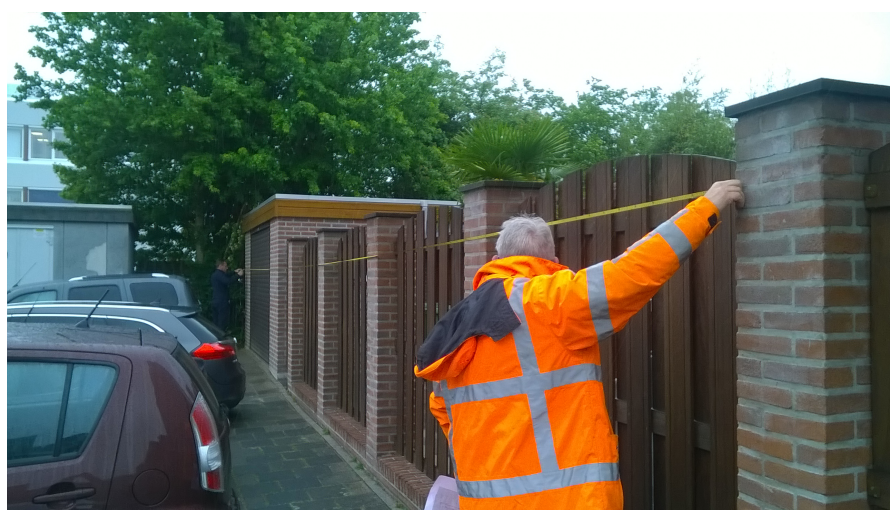
Figure 3.3: Land surveyors of the Kadaster reconstructing a boundary (photo taken by the author)
