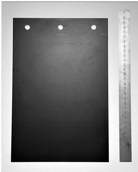
Figure 2.17: Photograph of the wing model having 200mm chord, 300mm span and 2mm thickness (in planform view) that was produced for the experiment performed for the present research. Next to it is a 30cm ruler. The three holes on the top serve for mounting of the wing to the frame of the experimental setup.
