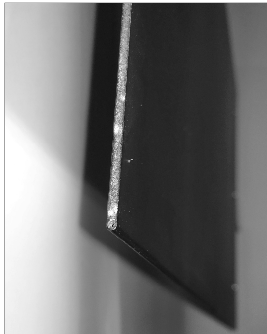
Figure 2.18: A photograph of the wing model (which is also shown in Figure 2.17) showing a cross-sectional view, zoomed-in on the trailing edge part. The white particles on the wing surface are dust particles.
