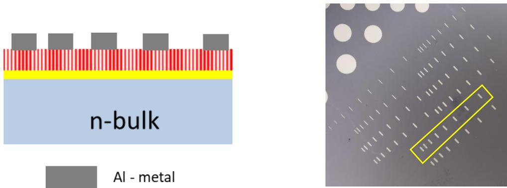
Figure 3.11 Left: Schematic of the TLM sample for  $n^+$  - CSPC. Right: Prepared sample for TLM measurements. Note: The yellow box on the right picture encloses the line of measurement used to measure the resistance.
