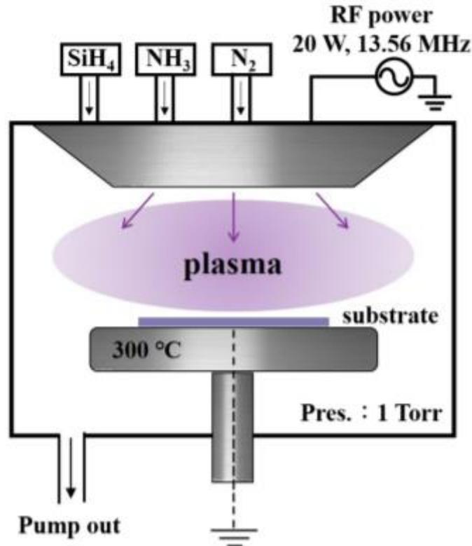
Figure 2.5 Schematic of Plasma Enhanced Chemical Vapour Deposition [26].
