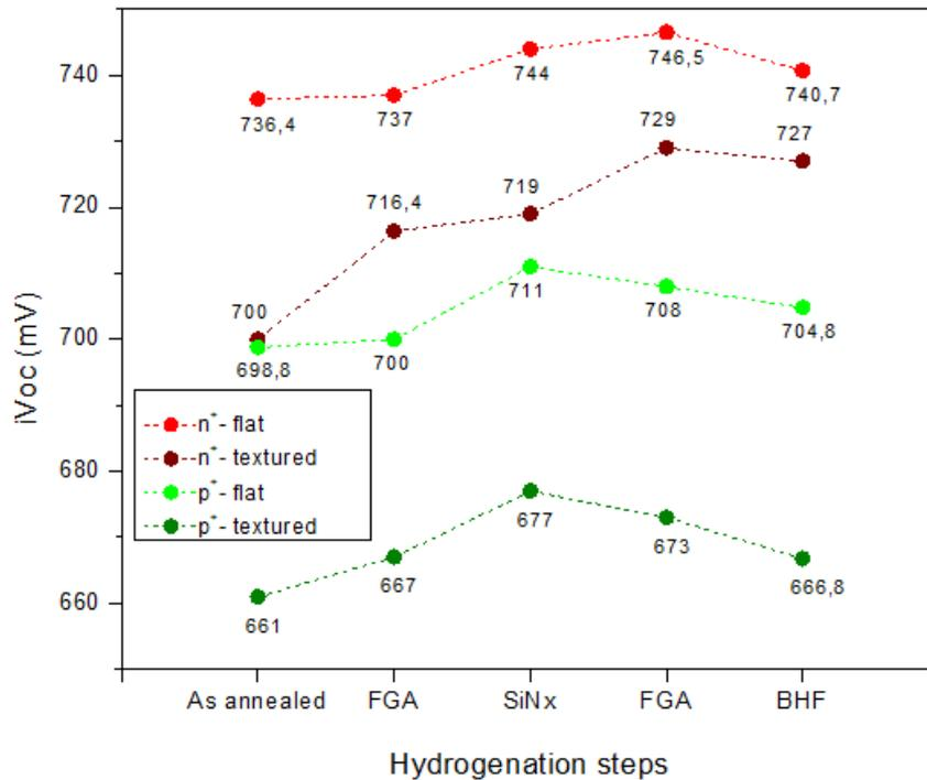
Figure 4.7 Passivation quality of the symmetric samples along the hydrogenation steps of SiN<sub>x</sub>-FGA. NOTE: The data points are connected with dotted line just to guide the eyes.
