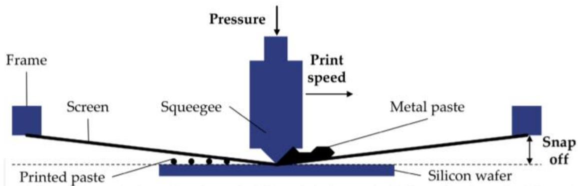
Figure 2.8 Schematic of metal screen printing [33].
