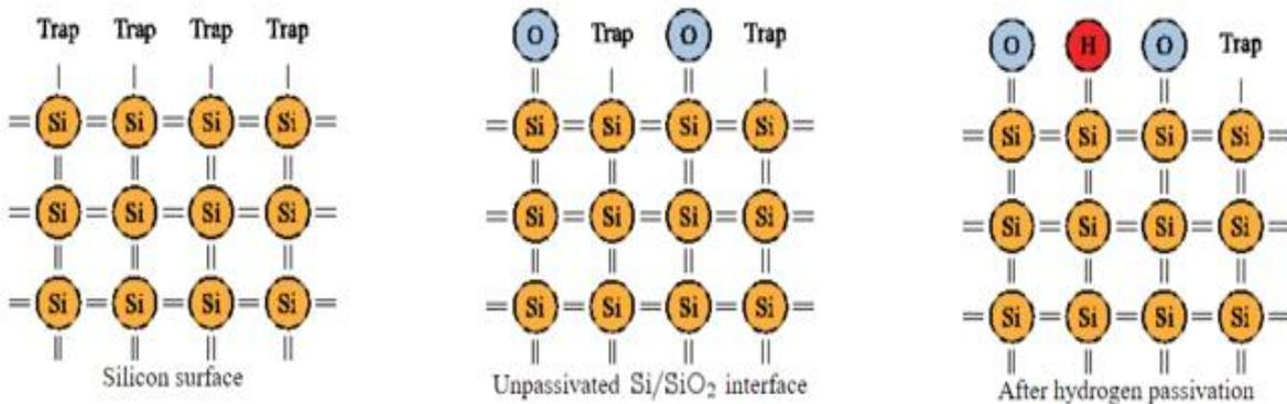
Figure 1.6 Chemical passivation by silicon oxide and hydrogen atoms [7].
