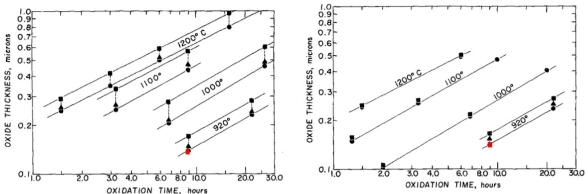
Figure 3.8 Left: The thermal Silicon Oxide thickness for different doping concentration of Boron with respect to the oxidation time during dry oxidation. Right: Similar for different doping concentration of Phosphorous [57]. Note: The line with the red square represents boron doping concentration of  $1 \text{ e}16 \text{ cm}^{-3}$  (Left) and phosphorous doping concentration of  $4 \text{ e}15 \text{ cm}^{-3}$  (Right).
