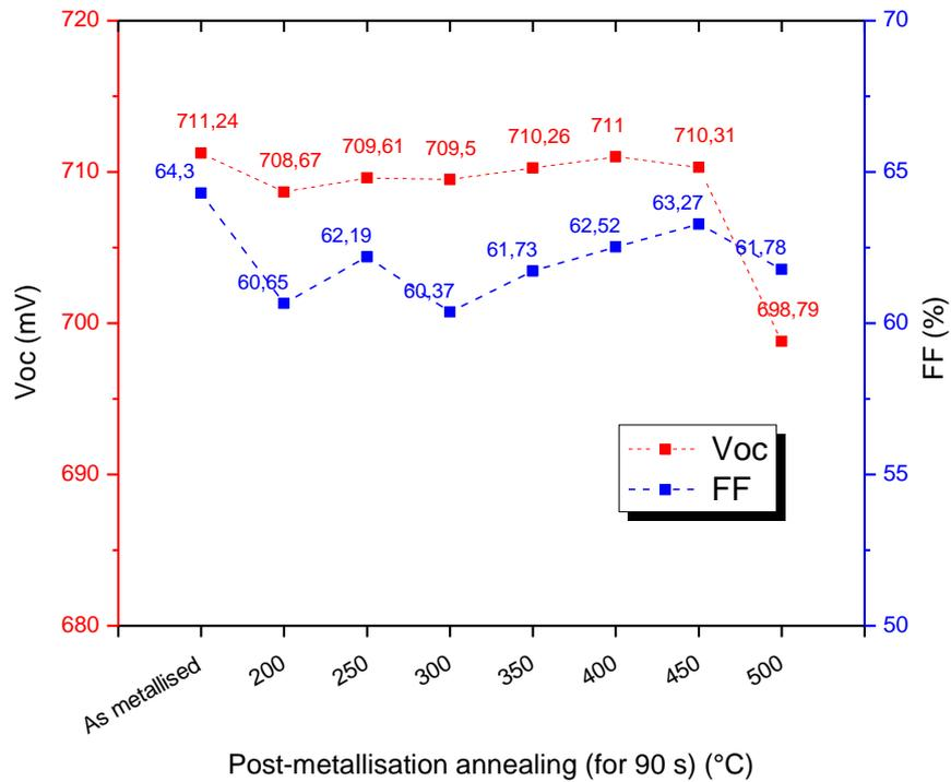
Figure 5.6 Voc and FF of Textured-Flat poly-poly solar cells along different post-metallisation annealing conditions
