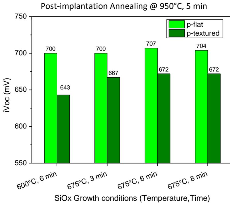
Figure 3.16 Passivation quality with respect to different thermal oxide conditions when annealed at 950°C, 5min. Top: For textured(wine) and flat(red) n+ poly-Si CSPC. Bottom: For textured (olive) and flat (green) p+ poly-Si CSPC.
