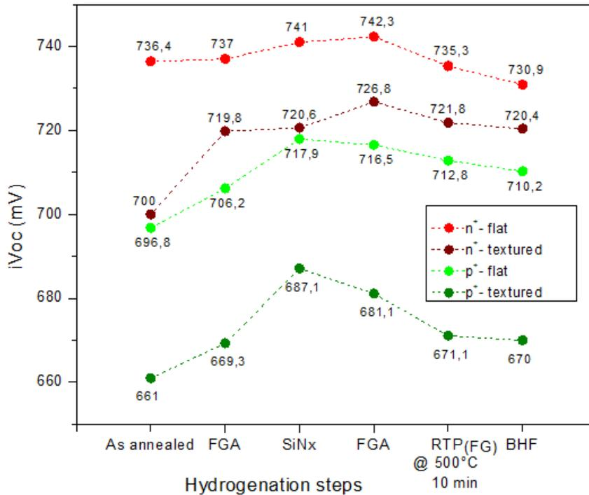
Figure 4.8 Passivation quality of the symmetric samples along the hydrogenation steps of SiN<sub>x</sub>-FGA-RTP. NOTE: The data points are connected with dotted line just to guide the eyes.
