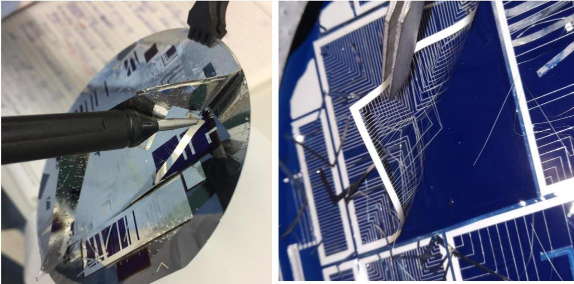
Figure 5.7 Metal peel-off during Lift-off process. Metallisation: Silver sputtering. Note: Left – on flat surface with 5  $\mu\text{m}$  thick metal. Right – on textured surface with 3  $\mu\text{m}$  thick metal.
