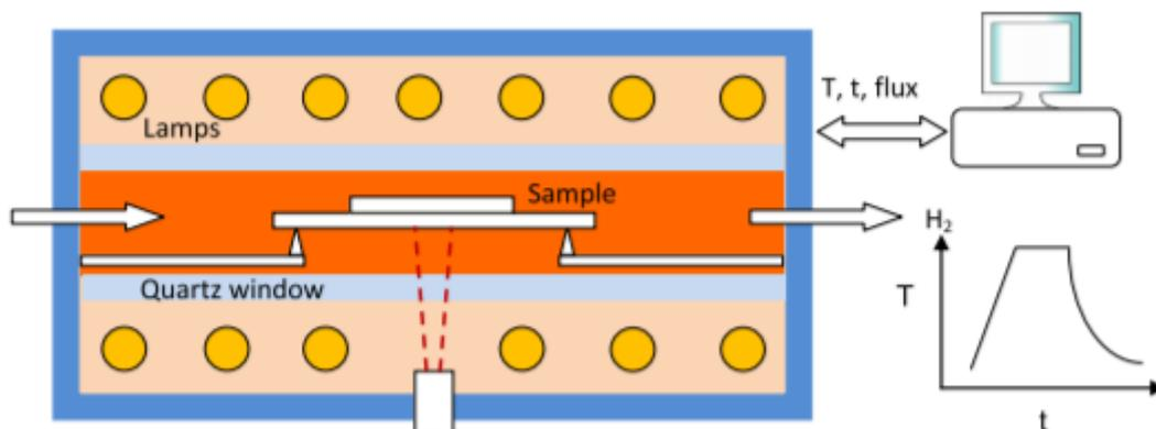
Figure 2.5 Schematic of Rapid Thermal Processing [23].
