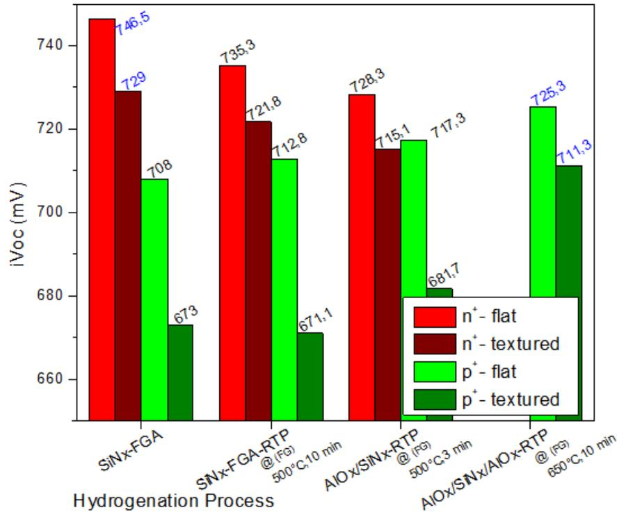
Figure 4.13 Passivation achieved with different hydrogenation processes for four different symmetric samples. NOTE: The hydrogenation conditions are mentioned along the x-axis. The last process is carried out only for the p<sup>+</sup> poly-Si samples. The best results are in blue.
