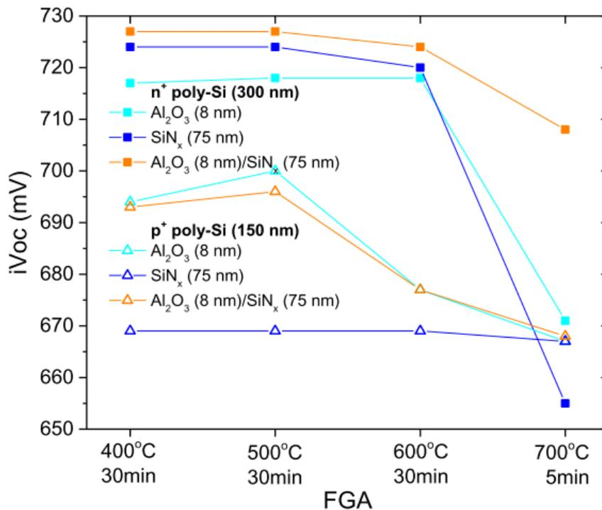
Figure 4.2 Passivation of the poly-Si CSPEC with respect to increase in annealing time and temperature [21].
