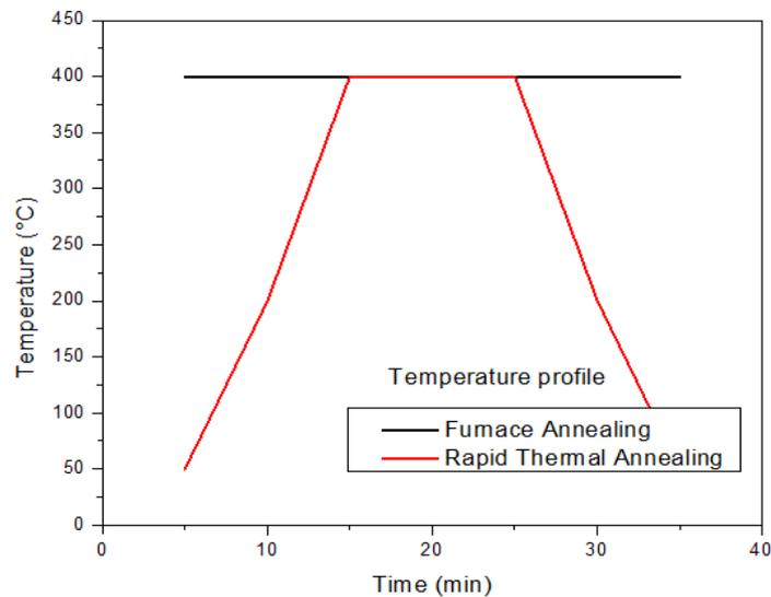
Figure 4.4 Temperature profile in furnace and rapid thermal annealing.
