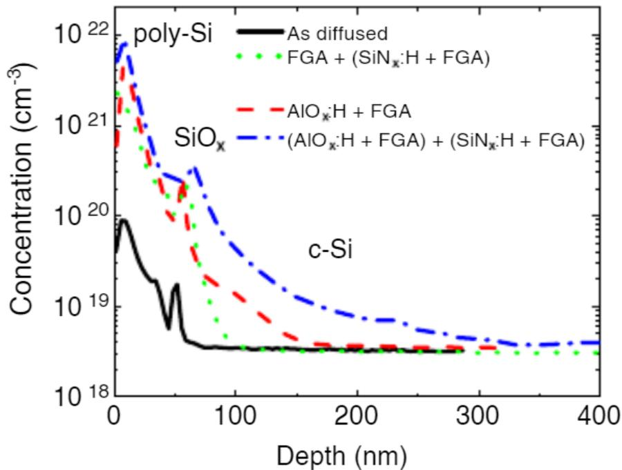
Figure 4.1 Hydrogen concentration profile taken by SIMS (Secondary Ion Mass Spectroscopy) with and without capping layers [67].
