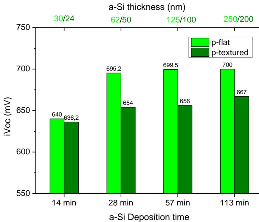
Figure 3.19 Passivation quality of poly-Si CSCP with respect to change in the thickness of the poly-Si layer (top x-axis) or with respect to the a-Si deposition time (bottom x-axis). Top: For textured(wine) and flat(red) n+ poly-Si CSCP. Bottom: For textured (olive) and flat (green) p+ poly-Si CSCP. NOTE: Thermal oxide growth condition is 675°C, 3 min and Post-implantation Annealing is done at 950°C, 5 min
