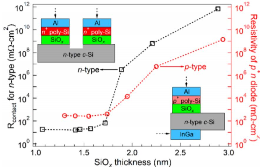
Figure 3.7 Contact resistivity of the  $n^+$  poly-Si (Black Squares) and  $p^+$  poly-Si layers (Red Circles) as a function of the thermal oxide thickness ranging from 1 nm to 3 nm [42].
