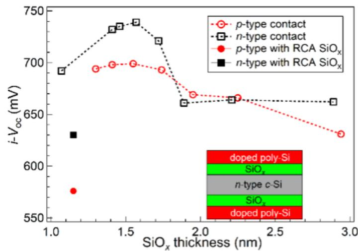
Figure 3.1 Effect of  $t\text{-SiO}_x$  on the  $iV_{oc}$  of  $n^+$  and  $p^+$ -polySi symmetric samples [42]
