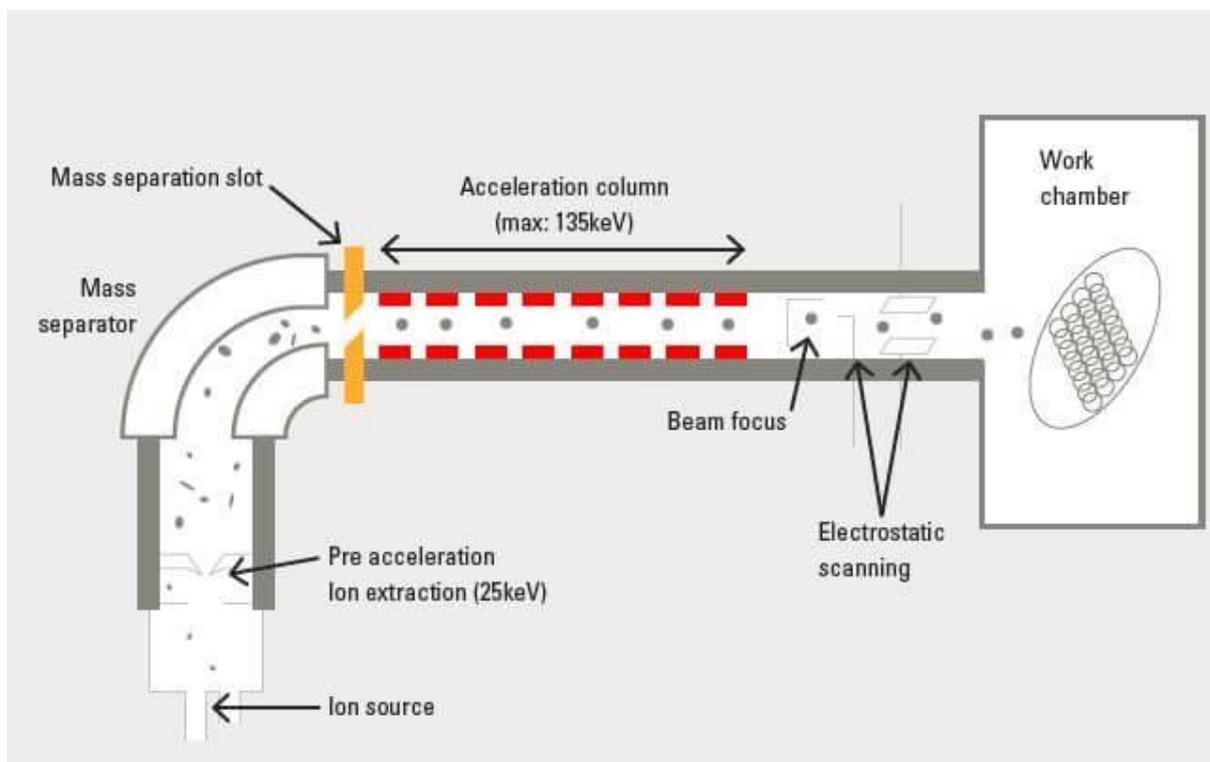
Figure 2.4 Schematic of a Varian ion implanter [19].
