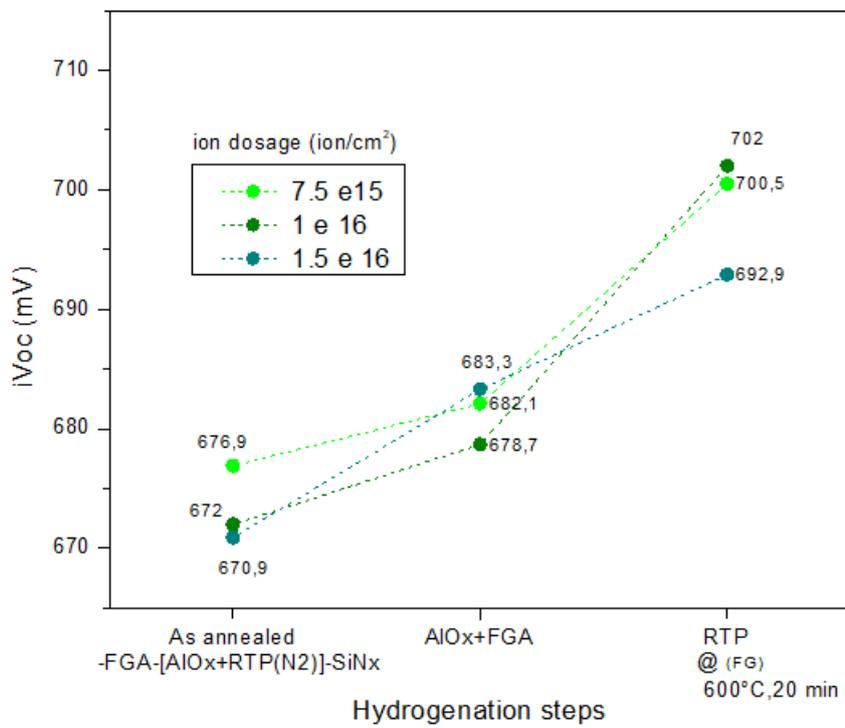
Figure 4.10 Passivation for textured p<sup>+</sup> poly-Si CSPC along the hydrogenation steps of AlO<sub>x</sub>/SiN<sub>x</sub>/AlO<sub>x</sub>-FGA-RTP @ 600°C, 20min. NOTE: Top – iV<sub>oc</sub> values throughout the hydrogenation step, Bottom – iV<sub>oc</sub> for the last three important steps to see the trend clearly.
