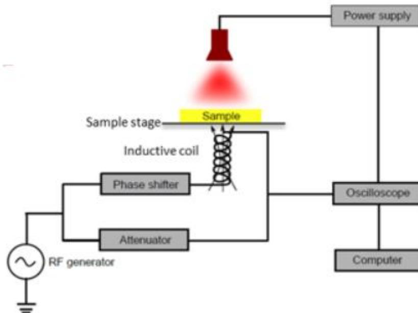
Figure 2.10 Schematic of Sinton lifetime measurement set-up [34]
