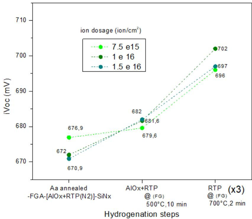
Figure 4.11 Passivation for textured p<sup>+</sup> poly-Si CSPC along the hydrogenation steps of AlO<sub>x</sub>/SiN<sub>x</sub>/AlO<sub>x</sub>-RTPs. NOTE: The annealing conditions are mentioned along the x-axis.
