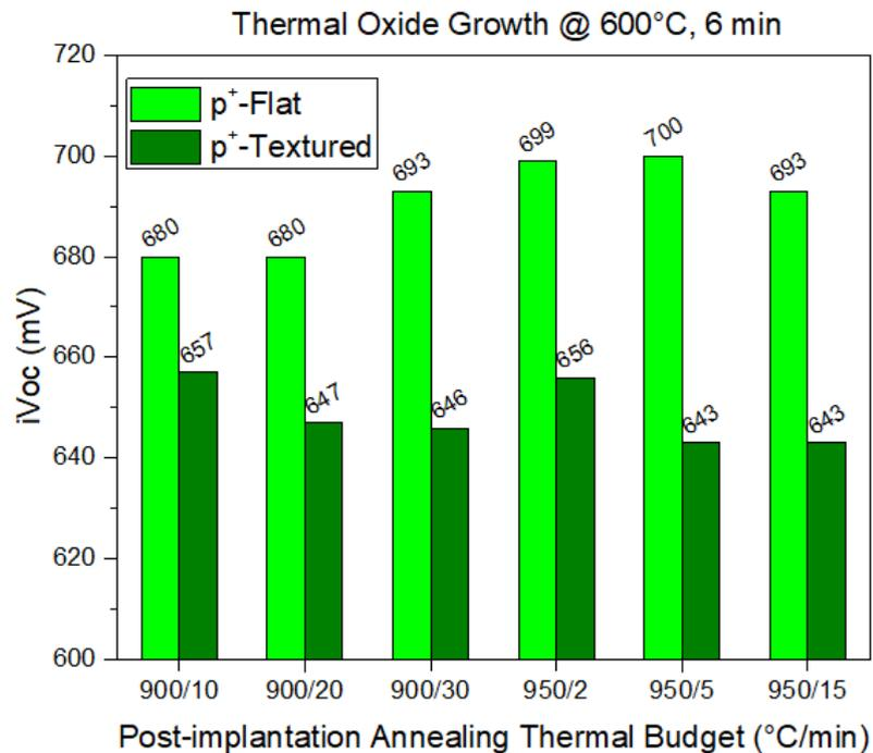
Figure 3.12 Passivation quality of thermal oxide grown at 600°C, 6 min with respect to the increase in post-implantation annealing thermal budget. Top: For textured(wine) and flat(red) n<sup>+</sup> poly-Si CSCP. Bottom: For textured (olive) and flat (green) p<sup>+</sup> poly-Si CSCP. NOTE: Along x-axis the values are expressed in (Temperature/Time) and it's not the rate of change of temperature.
