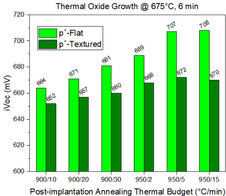
Figure 3.13 Passivation quality of thermal oxide grown at 675°C, 6 min with respect to the increase in post-implantation annealing thermal budget. Top: For textured(wine) and flat(red) n<sup>+</sup> poly-Si CSPC. Bottom: For textured (olive) and flat (green) p<sup>+</sup> poly-Si CSPC. NOTE: Along x-axis the values are expressed in (Temperature/Time) and it's not the rate of change of temperature.
