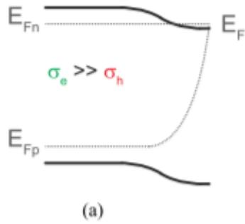
Here, the electron selectivity is achieved by introducing heavy  $n^+$  doping adjacent to the n-layer. The working is the same as front surface field introduced in Figure 1.8. Similar effect can also be achieved for hole selectivity as shown in Figure 1.7
