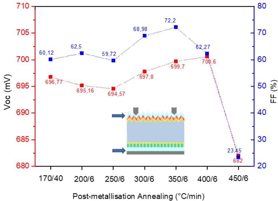
Figure 5.3  $V_{oc}$  and FF of Textured-Flat poly-poly solar cells along different post-metallisation annealing steps. Note: (a) Without TCO, (b) TCO on front side (c) Double side TCO. First annealing step is carried out in an oven. The rest are done by hot-plate annealing.
