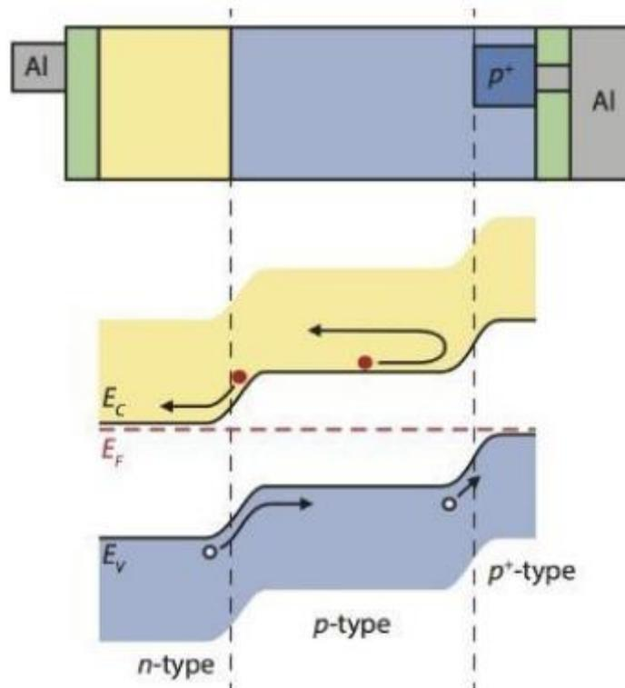
Figure 1.7 Band diagram of a back surface field [5].
