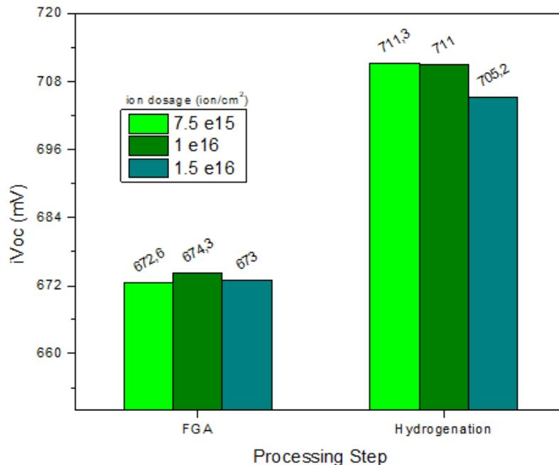
Figure 3.18 Passivation quality of textured  $p^+$  poly-Si CSPC with increase in doping concentrations before and after hydrogenation.
