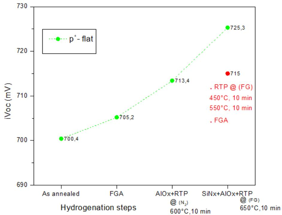
Figure 4.12 Passivation of p<sup>+</sup> poly-Si CSPC along the hydrogenation steps of AlO<sub>x</sub>/SiN<sub>x</sub>/AlO<sub>x</sub>-RTPs. NOTE: The annealing conditions are mentioned along the x-axis. Top – textured p<sup>+</sup> poly-Si. Bottom – flat p<sup>+</sup> poly-Si – The red dot shows the results of the other final annealing steps performed.
