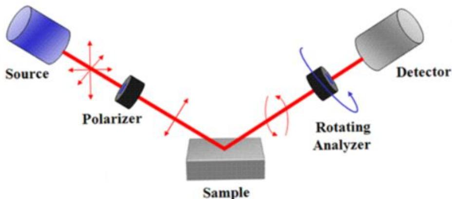
Figure 2.9 Working principle of Ellipsometry [34].
