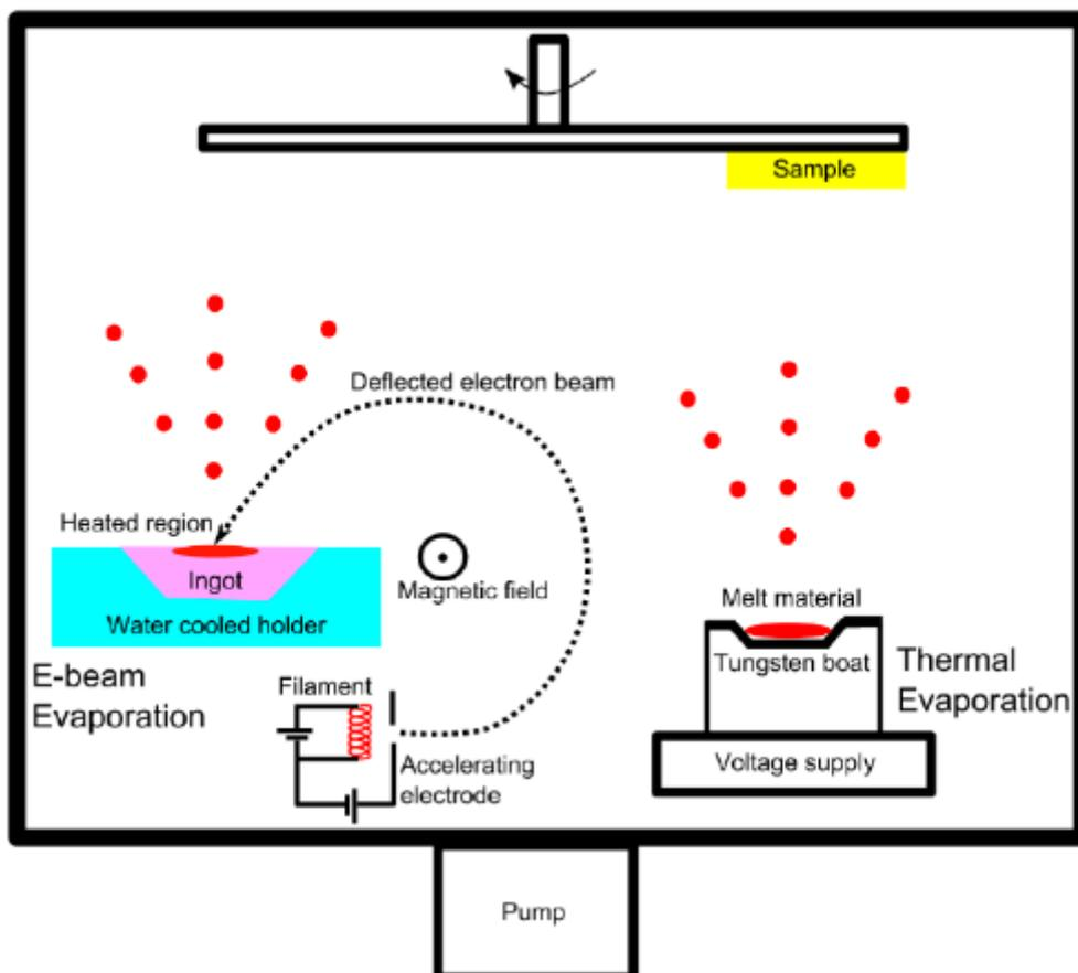
Figure 2.7 Thermal and e-beam evaporation of metal – Physical Vapour Deposition [30].
