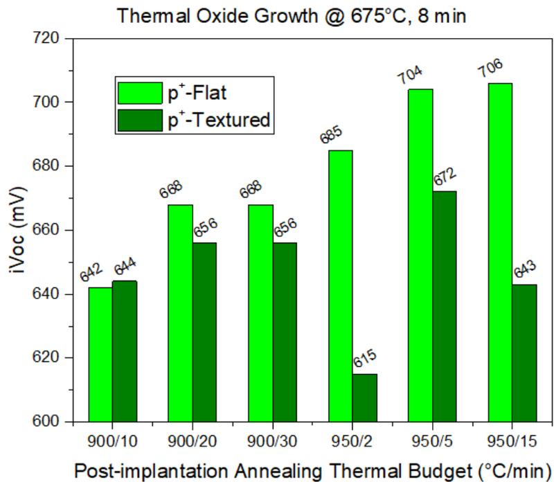
Figure 3.14 Passivation quality of thermal oxide grown at 675°C, 8 min with respect to the increase in post-implantation annealing thermal budget. Top: For textured(wine) and flat(red) n<sup>+</sup> poly-Si CSPC. Bottom: For textured (olive) and flat (green) p<sup>+</sup> poly-Si CSPC. NOTE: Along x-axis the values are expressed in (Temperature/Time) and it's not the rate of change of temperature.
