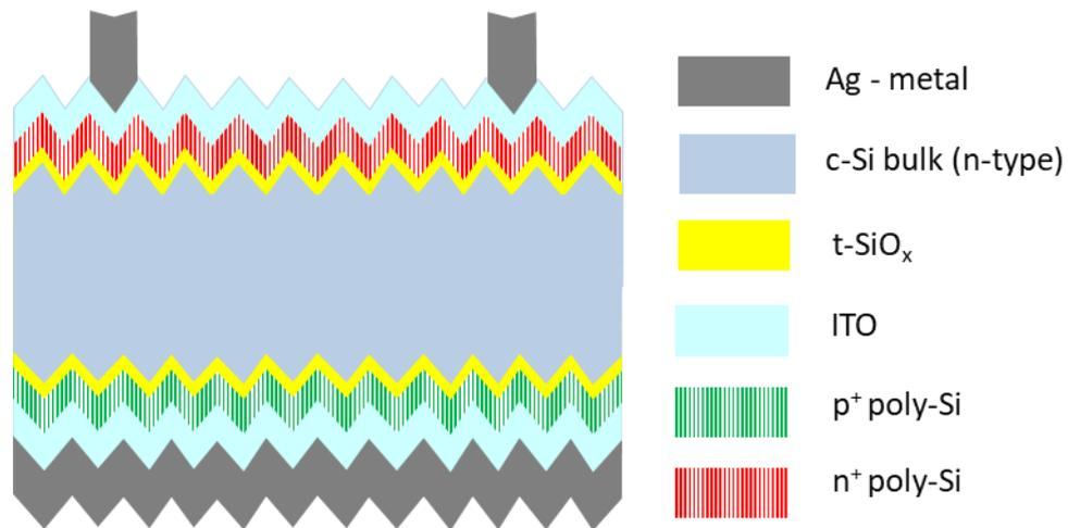
Figure 5.5 Schematic of a Textured-Textured poly-poly solar cell. Metallisation is done by SP.
