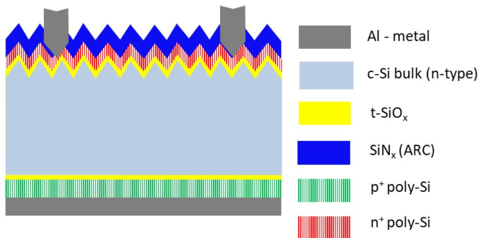
Figure 5.5 Schematic of a Textured-Flat poly-poly solar cell without TCO. Metallisation is done through e-beam Evaporation.
