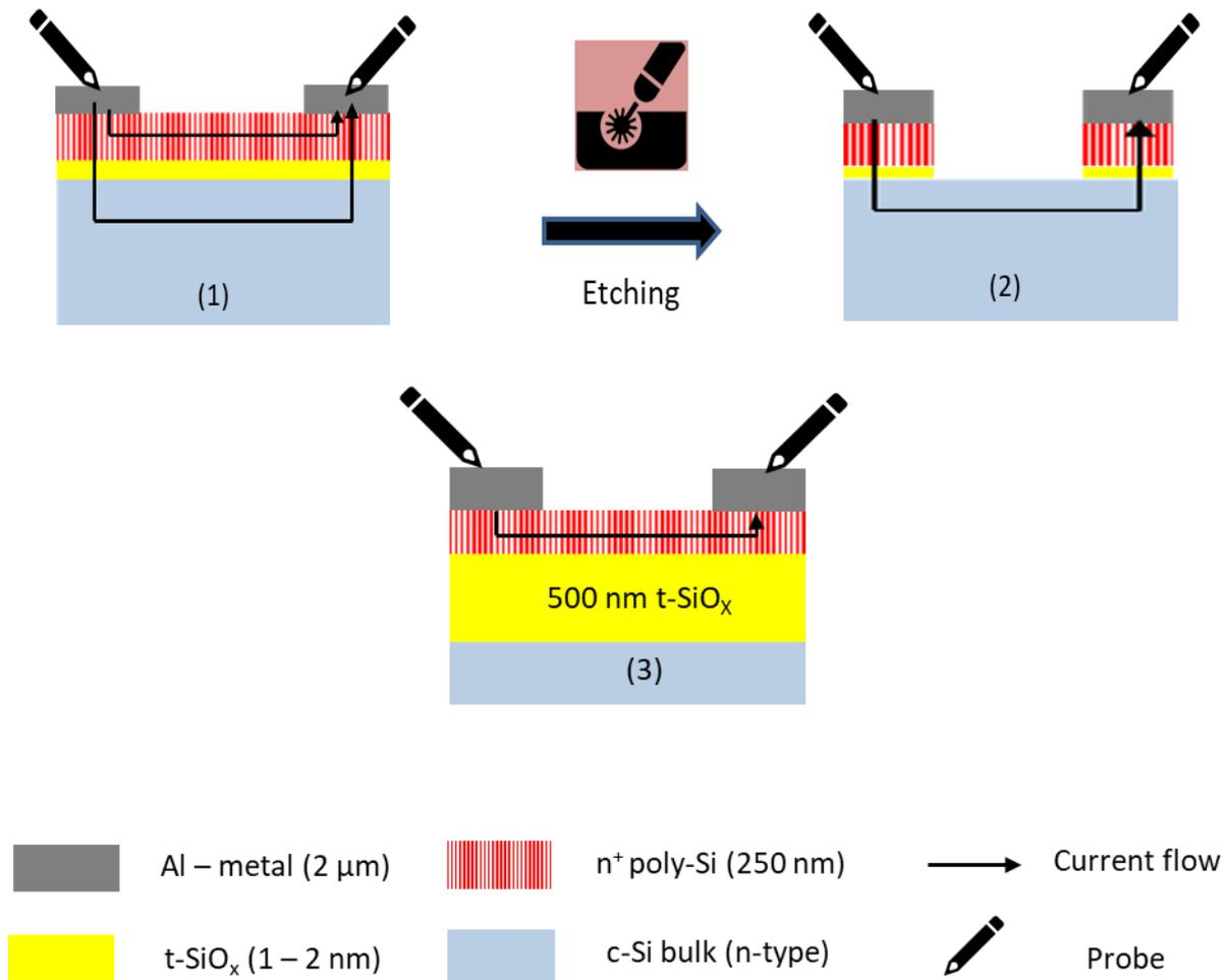
Figure 3.21 Schematic of the proposed sample structure for accurate measurement for the contact resistivity of the  $n^+$  CSPC. Sample (1)- Continuous poly-Si layer leading to lateral conductivity. Sample (2)- Etched sample to avoid lateral conductivity. Sample (3)- With thicker oxide to find the contact resistivity between metal and poly-Si layer.
