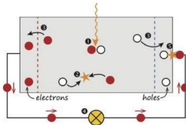
Figure 1.3 Solar cell model. 1. Generation of charge carriers 2. Recombination of charge carriers 3. Separation of charge carriers 4. Electrons passing through the external circuit 5. Recombination of electron-hole pair [5].
