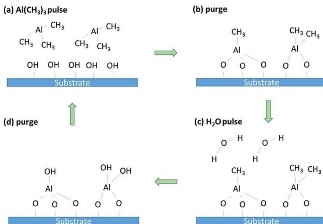
Figure 2.6 Aluminium Oxide growth mechanism by Atomic Layer Deposition [28].
