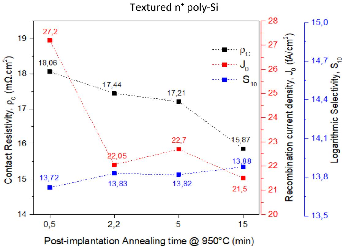
Figure 3.22 The change in contact resistivity ( $\rho_c$ ), recombination current density ( $J_0$ ) and logarithmic Selectivity ( $S_{10}$ ) with change in post-implantation annealing time at 950°C. NOTE: Top- Flat n<sup>+</sup> poly-Si CSPC, Bottom: Textured n<sup>+</sup> poly-Si CSPC. Thermal oxide growth condition - 675°C, 3 min. poly-Si thickness – 250 nm (flat). The data points are connected with dashed lines only for the purpose of guiding the eyes.
