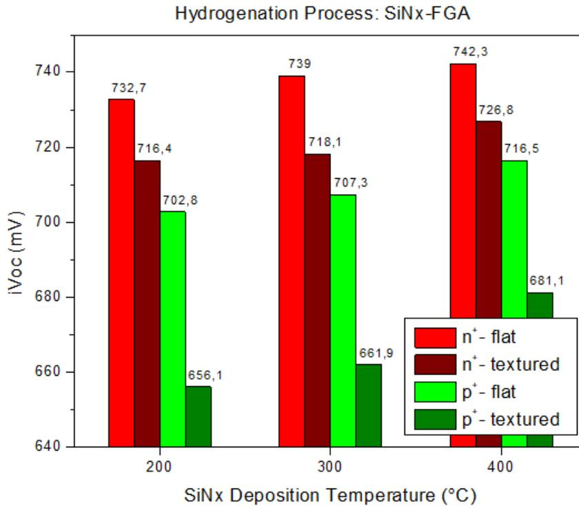
Figure 4.6 Passivation quality of SiN<sub>x</sub> capping layer after hydrogenation as a function of SiN<sub>x</sub> deposition temperature.
