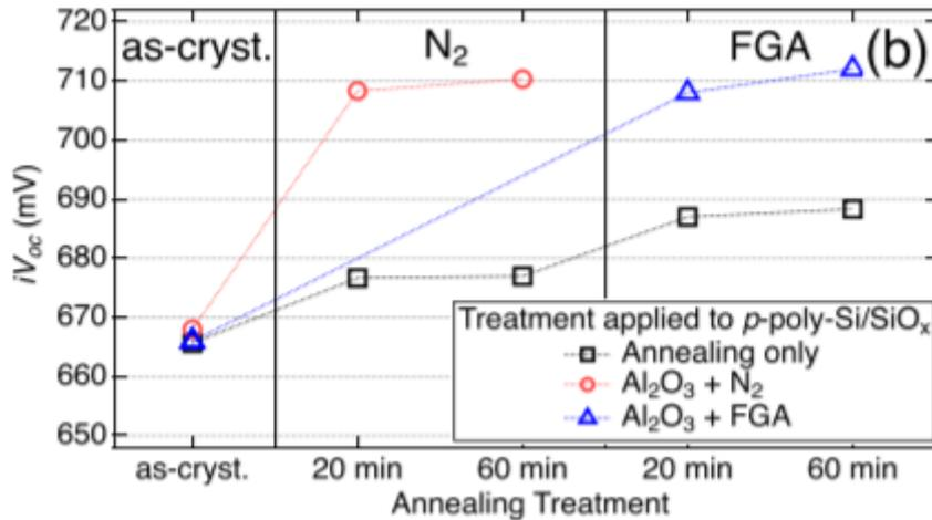
Figure 4.3 Passivation of  $p^+$  poly-Si CSPC with respect to annealing time in nitrogen and forming gas atmosphere with aluminium oxide capping layers [68].
