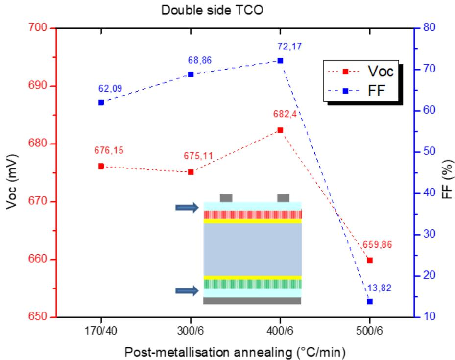
Figure 5.2  $V_{oc}$  and FF of Flat-Flat poly-poly solar cells along different post-metallisation annealing steps. Note: (a) Without TCO, (b) TCO on front side (c) Double side TCO. First annealing step is carried out in an oven. The rest are done by hot-plate annealing.
