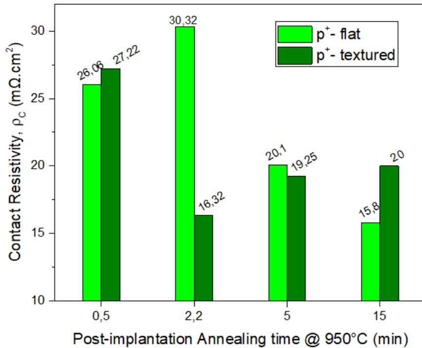
Figure 3.20 The contact resistivity of the CSPCs as a function of increasing post-implantation annealing time. Top: For textured(wine) and flat(red) n+ poly-Si CSPC. Bottom: For textured (olive) and flat (green) p+ poly-Si CSPC. NOTE: Thermal oxide growth condition is 675°C, 3 min and Post-implantation Annealing is done at 950°
