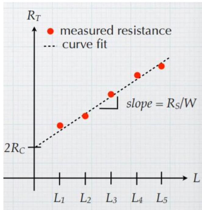
Figure 2.10 TLM – Resistance as a function of the distance between metals [35].
