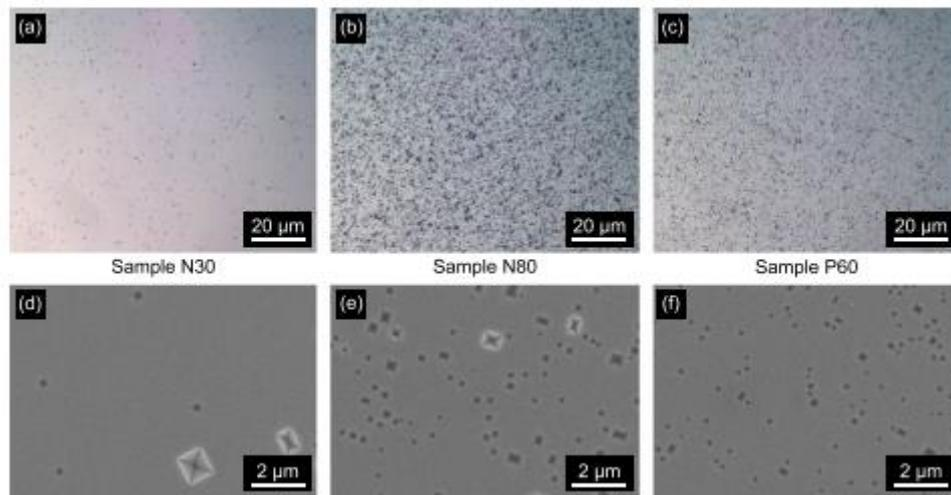
Figure 3.2 [a-c] OM and [d-f] SEM images of the pin hole for three different samples [43].
