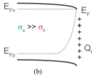
An external potential source or a layer with a large fixed charge capacity ( $Q_f$ ) is introduced to change the surface carrier concentration. Here a high surface concentration of electrons is achieved by having a layer with high fixed positive charges.
