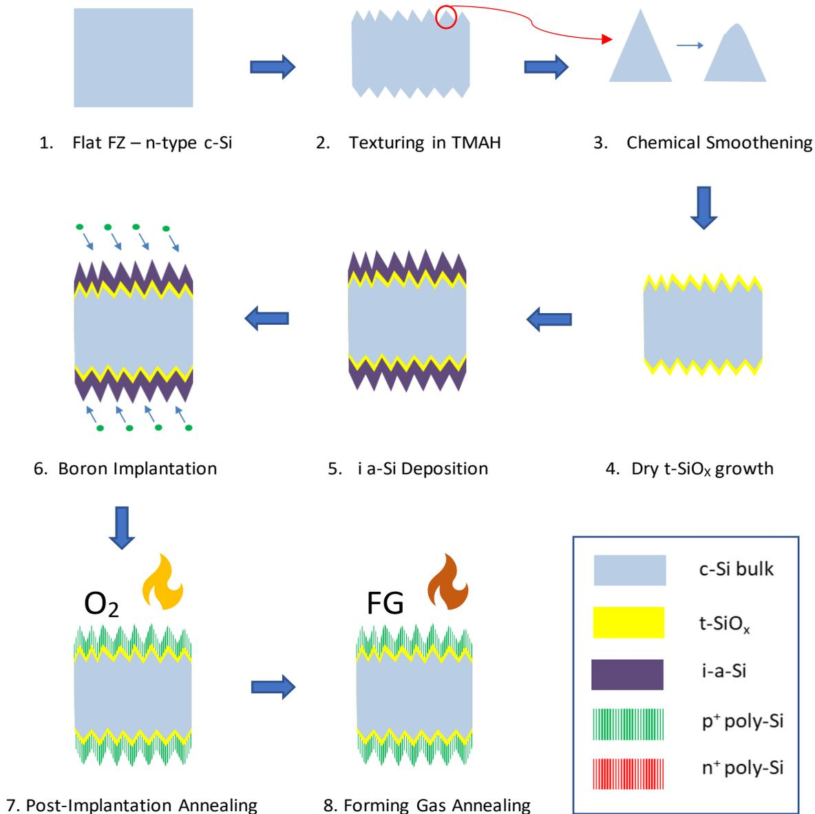
Figure 3.9 Flow chart for the fabrication of textured p<sup>+</sup> poly-Si symmetric sample.
