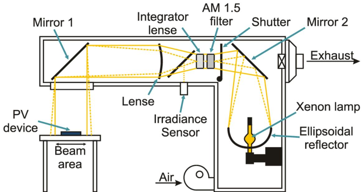
Figure 2.11 Current-Voltage measurement set-up [36].
