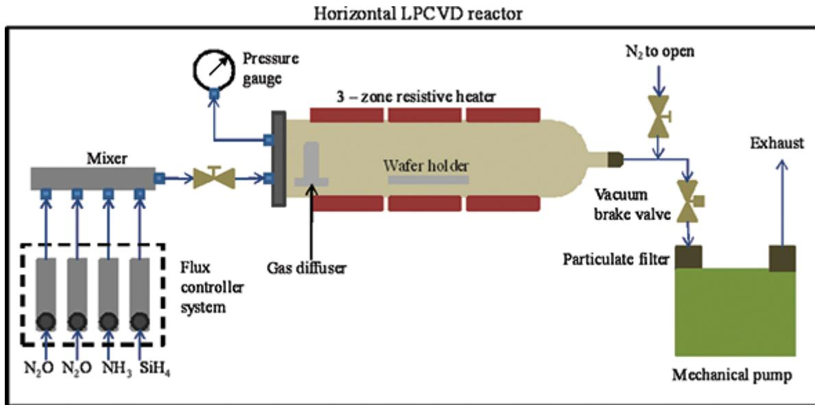
Figure 2.3 Schematic of a LPCVD reactor [18].
