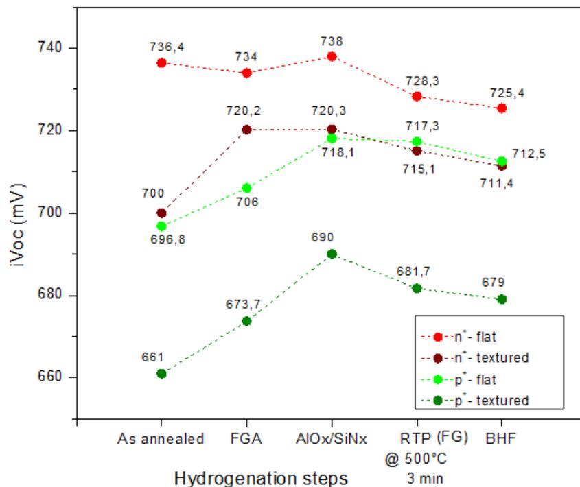
Figure 4.9 Passivation quality of the symmetric samples along the hydrogenation steps of  $\text{AlO}_x/\text{SiN}_x\text{-RTP}$ . NOTE: The data points are connected with dotted line just to guide the eyes.
