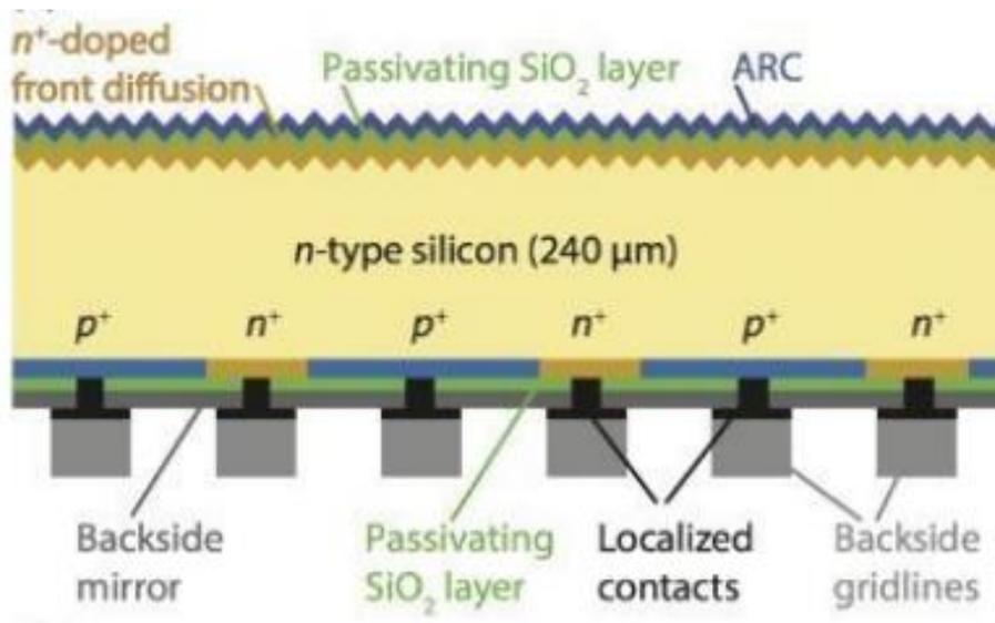
Figure 1.8 IBC solar cell architecture [5].
