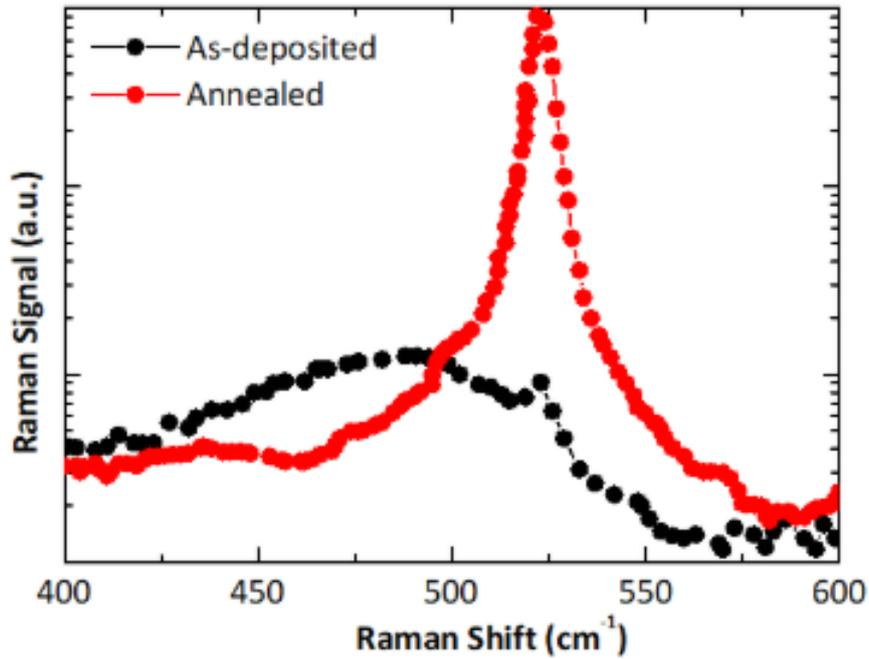
Figure 3.6 Raman spectra of a-Si (black) and poly-Si (orange) after annealing at 950°C [20].
