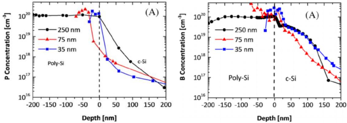
Figure 3.3 Electrochemical capacitance-voltage (ECV) profiling for the CSPC layers. Left: Doping profile of three different textured  $n^+$  poly-Si samples of thicknesses 250, 75 and 35 nm. Right: Similar plot for flat  $p^+$  poly-Si samples. [20] Note: The dotted line in the middle of the plot indicated the presence of a thin  $\text{SiO}_x$  layer of 1.5 nm
