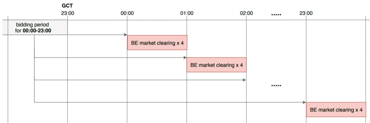
Fig. 4. Bidding procedure and market clearing in the joint BC-BE auction.
