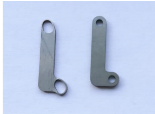
Figure 11: Left: Original design of the bar linkage, which got deformed during the experimental tests. Right: New design of the bar linkage.
