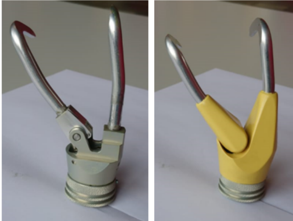
Figure 10: Prototype of the WILMER appealing prehensor with VC controlling mechanisms. Left: Without cosmetic cover. Right: With cosmetic cover.
