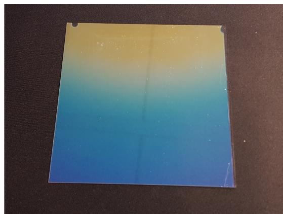
**Figure 7.14:** Color degradation in a multilayer structure based on magnesium fluoride and titanium dioxide. This effect indicates that the surface is not uniform.
