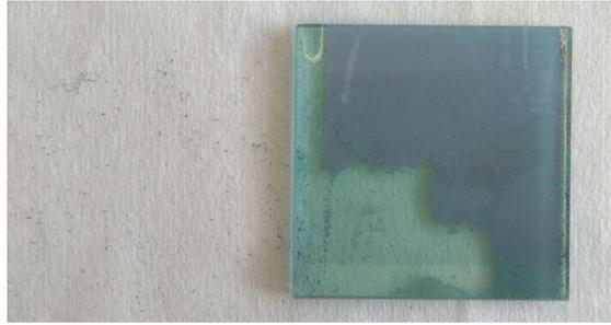
**Figure 7.11:** Stress in a flat-glass substrate sample after the deposition of seven layers. Some particle remains can be seen on the lateral side.
