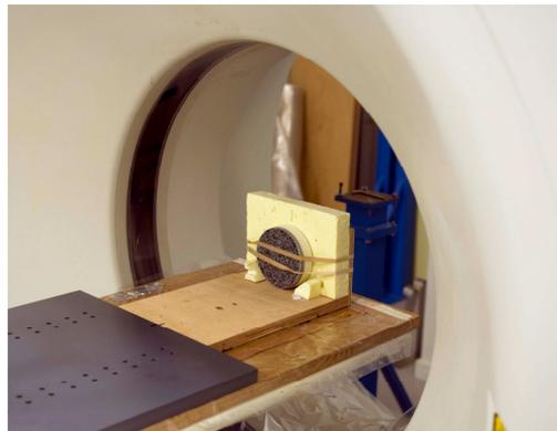
**Figure 4-26 Mounting of the sample for CT scanning**
