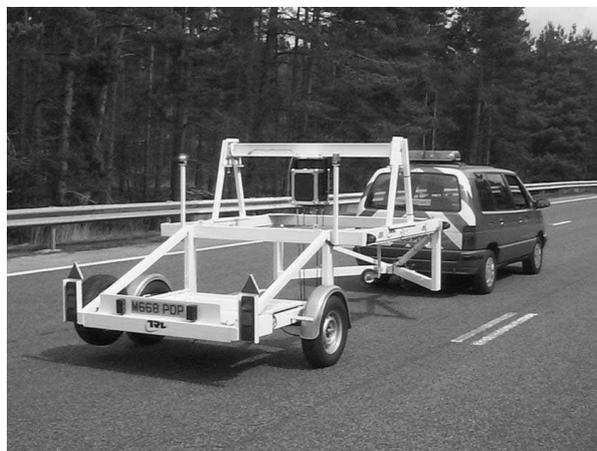
**Figure 2-21 Mobile MIRIAD system, developed by TRL [76]**
