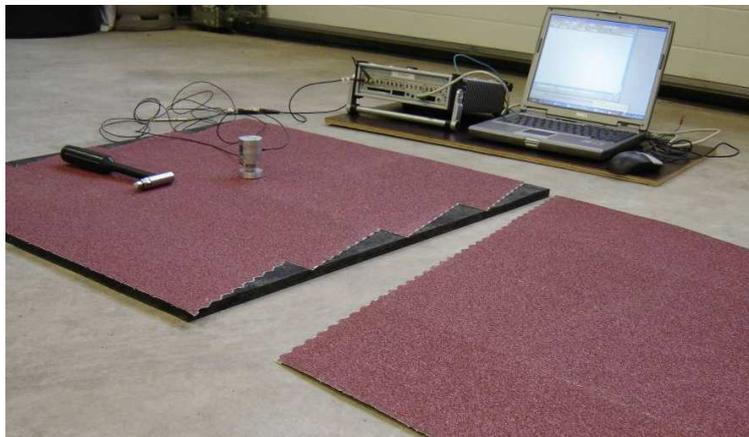
**Figure 2-26 Measurement device for mechanical impedance [81]**
