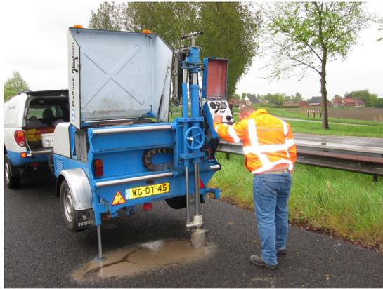
(c) Drilling the core
