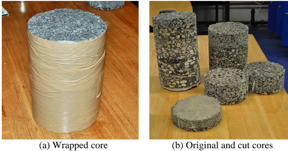
**Figure 4-11 Examples of the wrapped core and cut cores**
