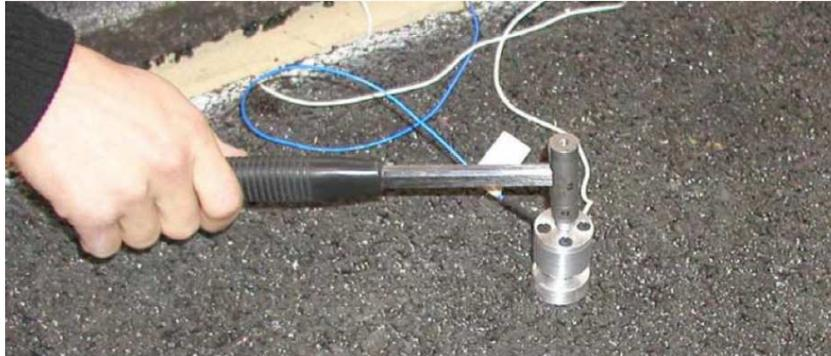
**Figure 2-25 Impedance head developed by Nilsson and Sylwan [81]**
