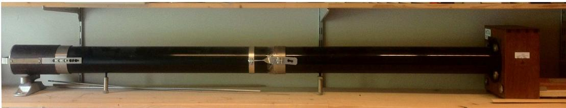
**Figure 4-17 Impedance tube for sound absorption measurement**
