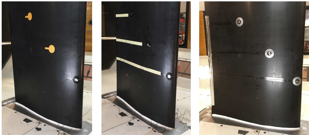
Figure 4. Sequence of microphones installation on the model.
