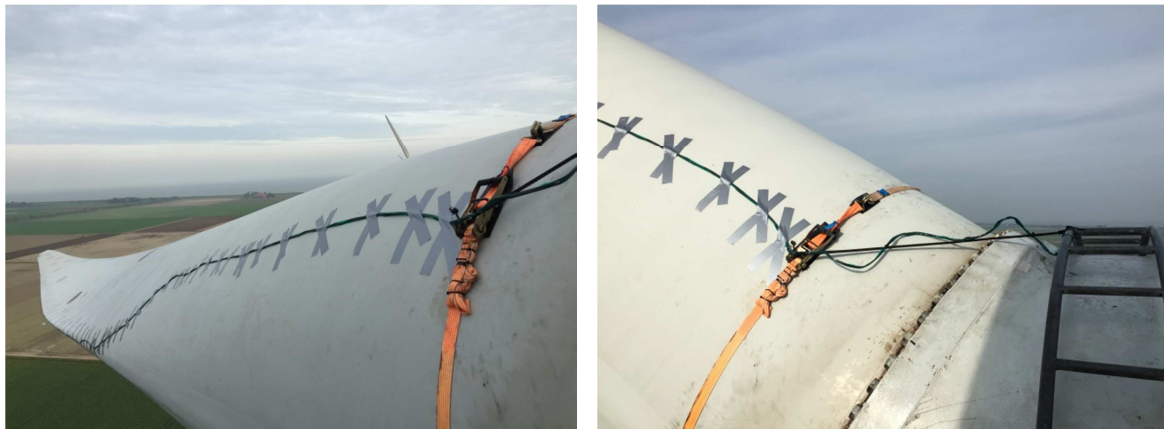
Figure 5. Microphones cabling rooting along the blade
