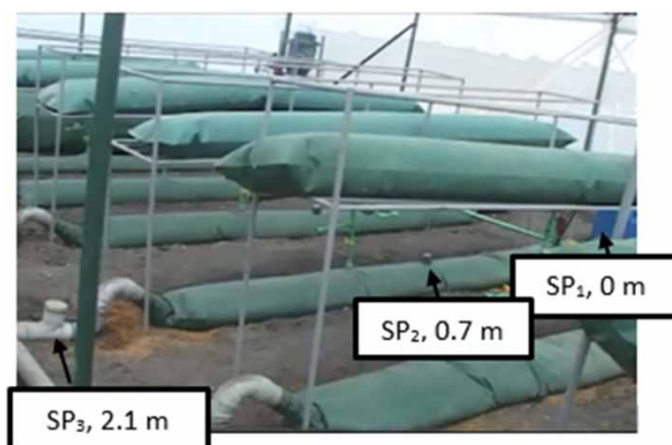
Figure 1 | Plug flow digester layout; reactors on the floor, biogas collection bags directly above; sampling points are indicated (SP1, 2 and 3).
