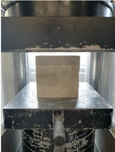
*Figure 3.9 Concrete cube before compression test. Cube is faced sideways and positioned in the center of the press.*
