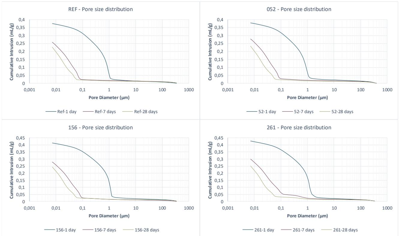
Figure 4.13 Pore size distributions per mixture. Blue=1 day porosity; Red=7 days porosity; Green=28 days porosity
