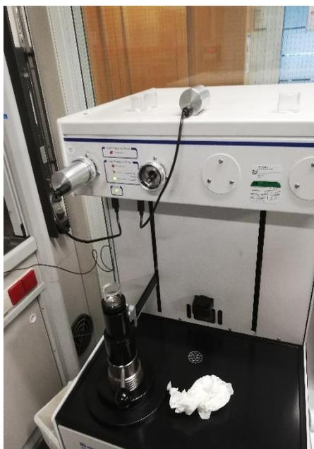
Figure 3.5 Mercury intrusion porosimeter
