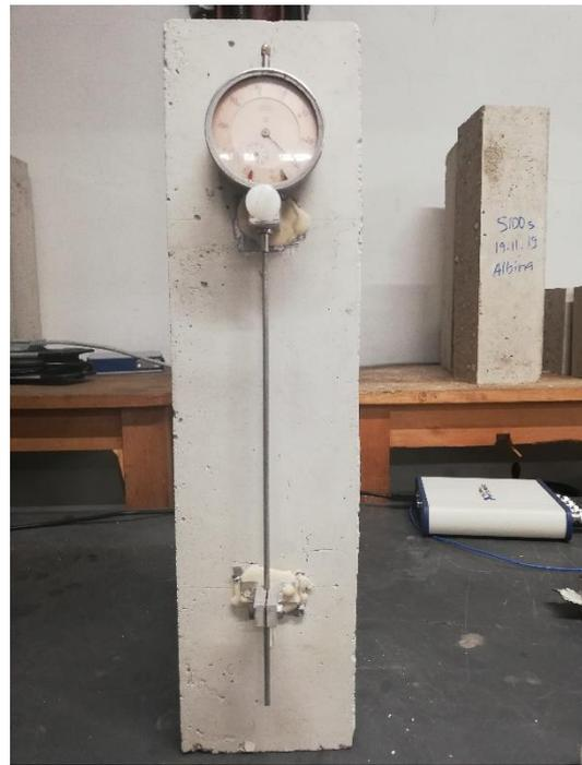
Figure 3.14 Concrete drying shrinkage setup. Prism is exposed to the air after removal of bitumen foil.
