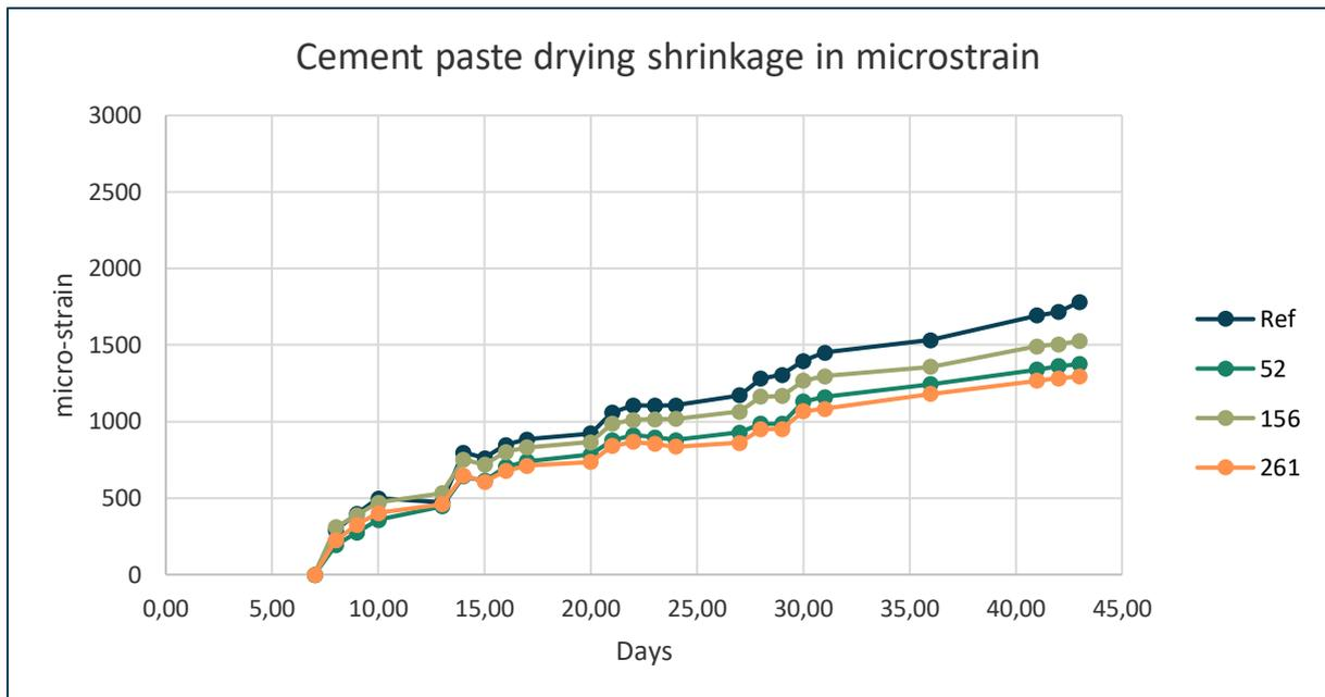
Figure 4.7 Cement paste CEM III/B and  $w/c=0.48$  drying shrinkage in micro strain starting at moment of unwrapping. Ref=Blue, 0 w% SRA, 52=Dark green, 0.52 w% SRA, 156=Light green, 1.56 w% SRA, 261=Orange, 2.61 w% SRA.
