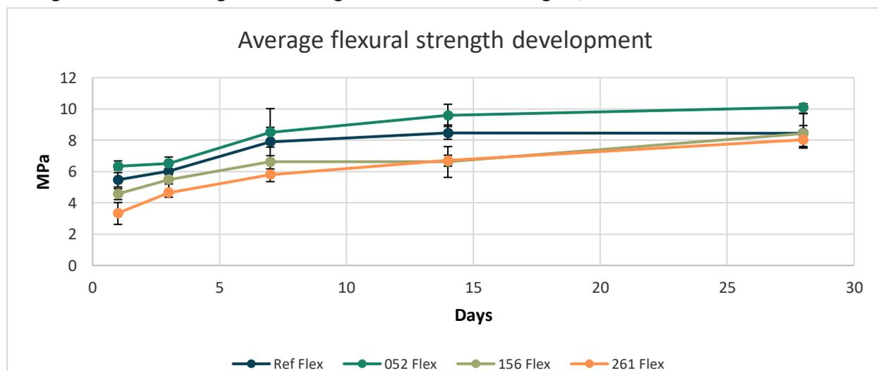
Figure 4.10 Average flexural strength development in MPa. Ref Flex=Blue, 0 w% SRA; 052 Flex=Dark green, 0.52 w% SRA; 156 Flex=Light green, 1.56 w% SRA; 261 Flex=Orange, 2.61 w% SRA.
