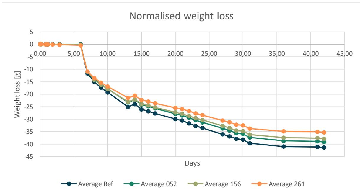
Figure 4.9 Average cement paste weight loss per mixture. Average Ref: Blue, 0 w% SRA; Average 052: Dark green; 0.52 w% SRA; Average 156: Light green, 1.56 w% SRA; Average 261: Orange, 2.61 w% SRA.
