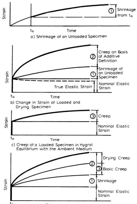
Figure 2.3 Time-dependent deformations in concrete subjected to a sustained load (Neville, 1995)
