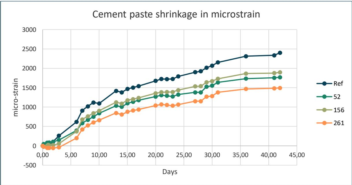
Figure 4.6 Cement paste CEM III/B and w/c=0.48 autogenous + drying shrinkage . First 7 days no loss of water, from day 7 onwards samples were exposed to drying. Ref=Blue, 0 w% SRA, 52=Dark green, 0.52 w% SRA, 156=Light green, 1.56 w% SRA, 261=Orange, 2.61 w% SRA.
