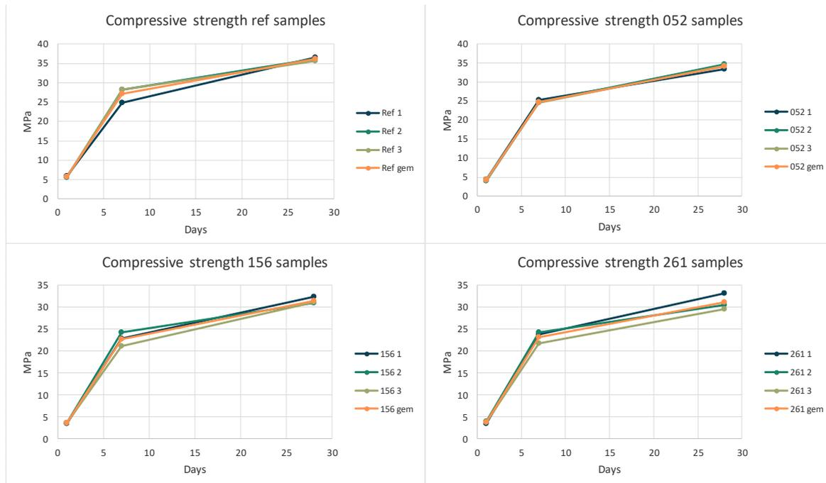
Figure 4.22 Concrete cube compressive stresses per mixture. Ref= 0 w% SRA; 052= 0.52 w% SRA; 156= 1.56 w% SRA; 261= 2.61 w% SRA.
