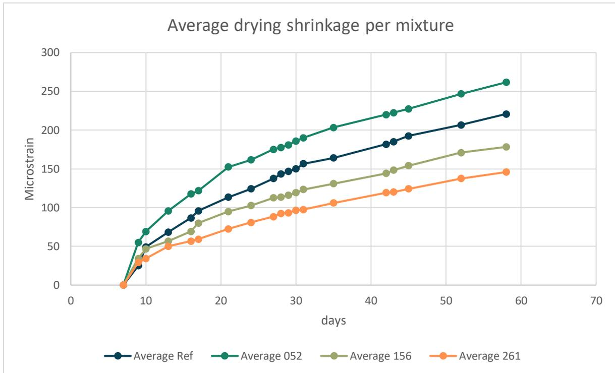
Figure 4.20 Average drying shrinkage per mixture from moment of unwrapping (day 7). Blue=Reference, 0 w% SRA; Dark green=052, 0.52 w% SRA; Light green=156, 1.56 w% SRA; Orange=261, 2.61 w% SRA.
