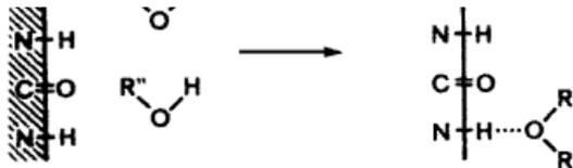
Figure 2.7 Hydrogen bonding (Rosen, 2004)
