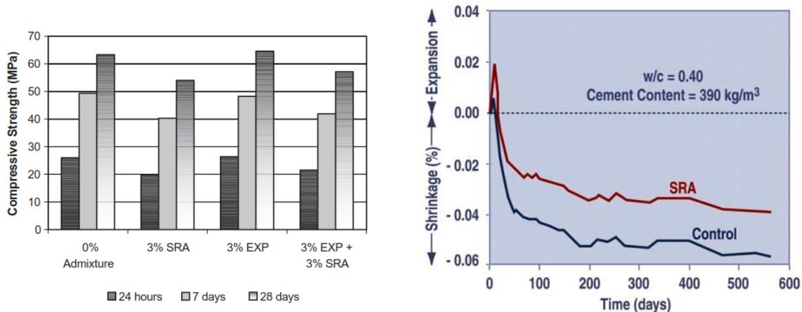
Figure 2.12 Shrinkage reductions with SRA similar to Sika Control 40. 390 kg/m<sup>3</sup> cement, 0.4 w/c and one week wet curing at 25 degrees Celsius. (Collepari et al., 2005)
