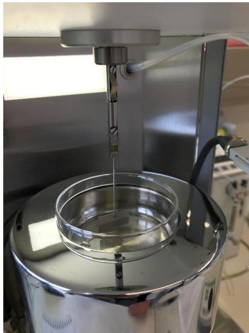
Figure 3.2 Glass vessel with Krüss Standard Plate
