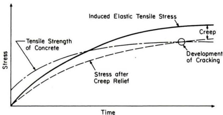
Figure 2.5 Schematic overview of crack development and interaction between shrinkage stress and creep (Neville, 1995)
