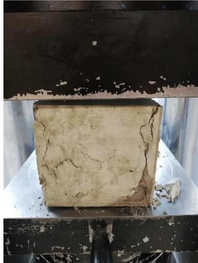
*Figure 3.10 Concrete cube after compression test.*
