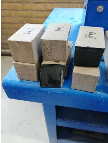
Figure 3.8 Paste compressive strength samples
