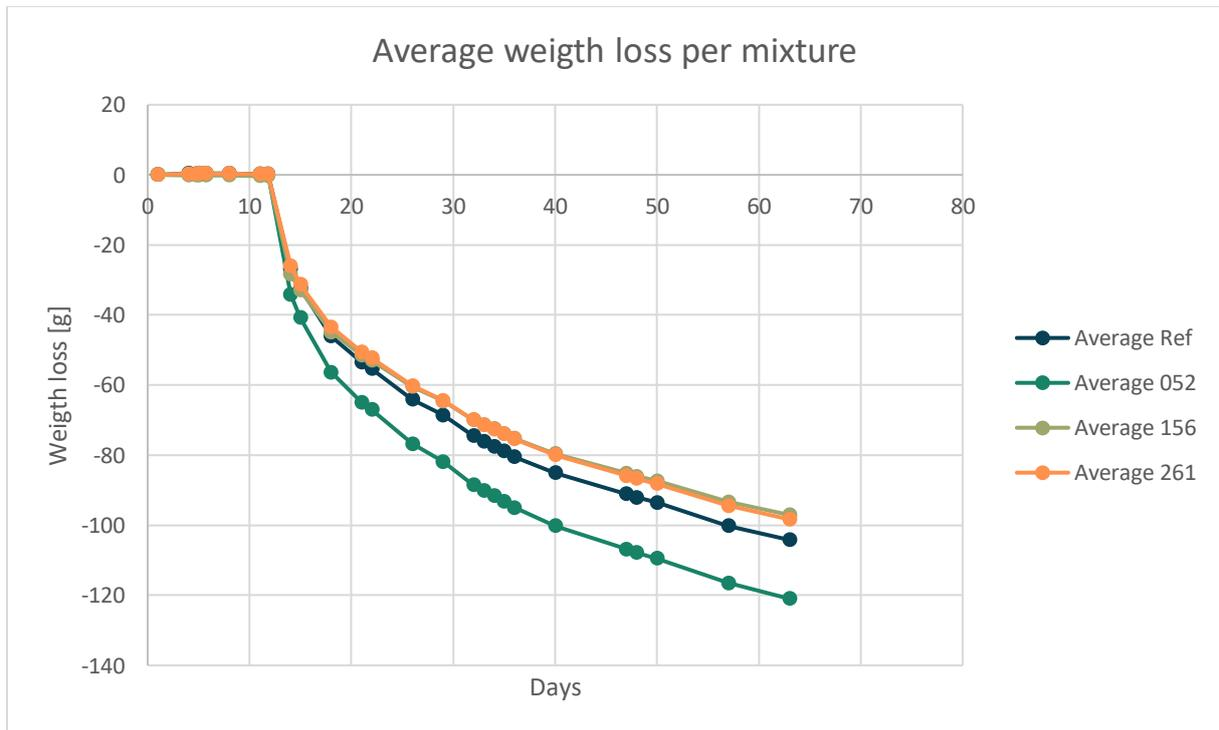
Figure 4.21 Weight loss per beam. First 7 days no weight loss was measured due to plastic foil. After 7 days samples were unwrapped and started drying. Mixtures Ref (0 w% SRA), 156 (1.56 w% SRA) and 261 (2.61 w% SRA) are very similar. Mixture 052 (0.52 w% SRA) loses more weight with respect to the other mixtures.
