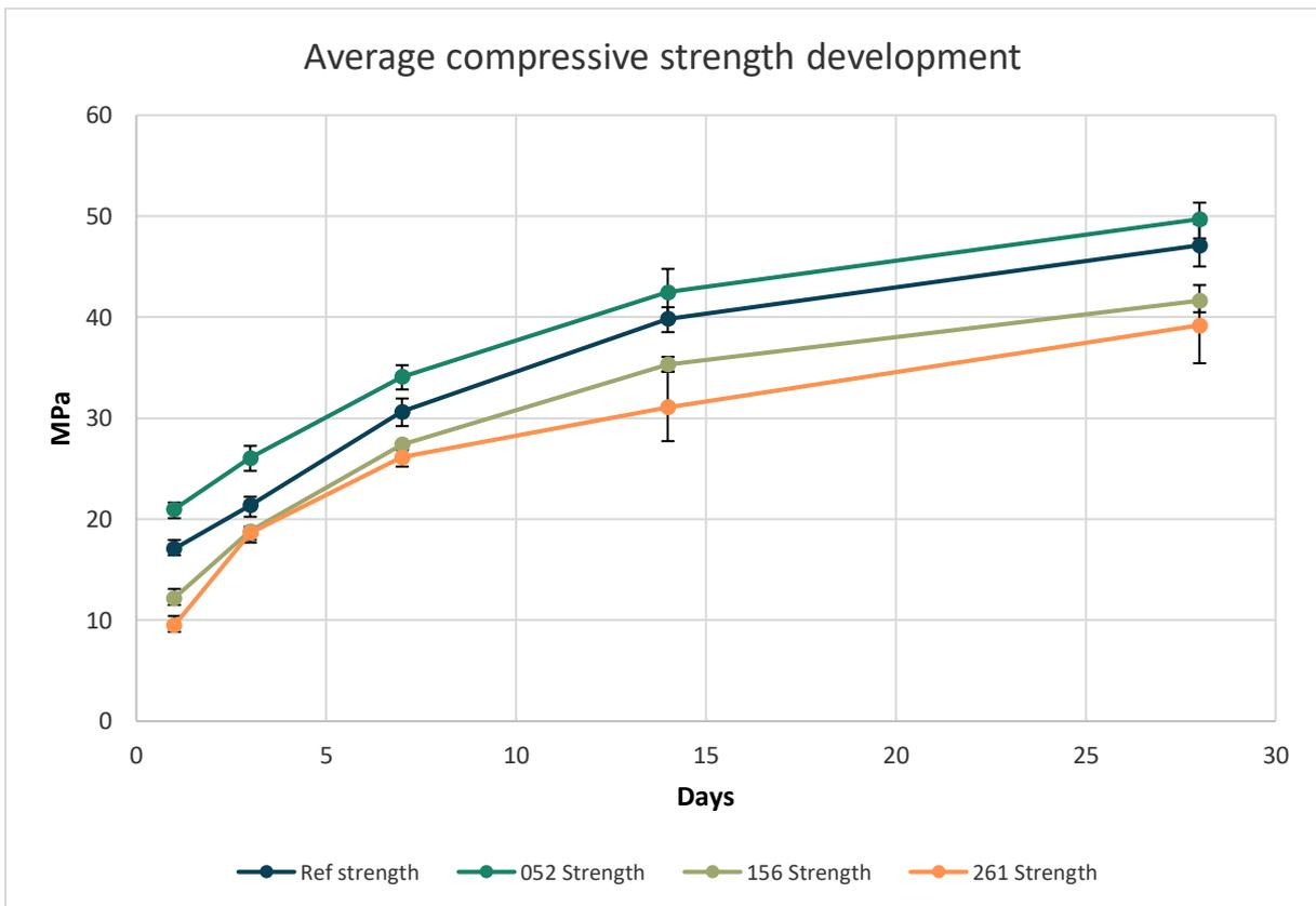
Figure 4.11 Average compressive strength in MPa. Ref strength=Blue, 0 w% SRA; 052 strength=Dark green, 0.52 w% SRA; 156 strength=Light green, 1.56 w% SRA; 261 strength=Orange, 2.61 w% SRA.
