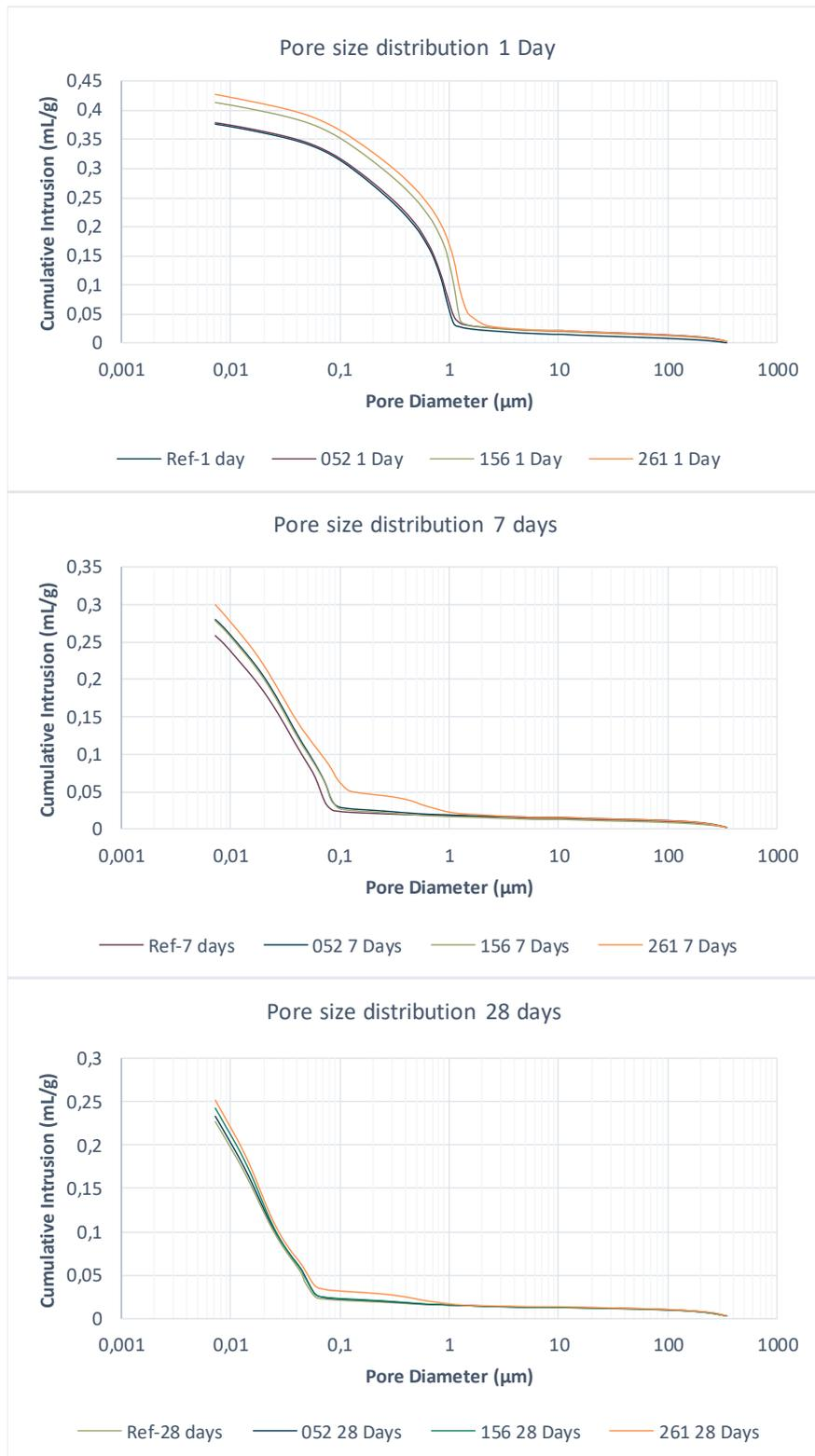
Figure 4.14 Comparison of pore size distributions. Top=Day 1 porosity per mixture; Middle=Day 7 porosity per mixture; Bottom=Day 28 porosity per mixture.
