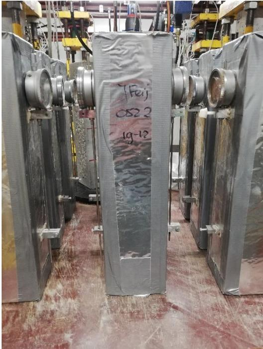
Figure 3.13 Concrete autogenous shrinkage setup. Prism is sealed with bitumen foil and duct tape. Two measuring clocks are attached on opposite sides per prism.
