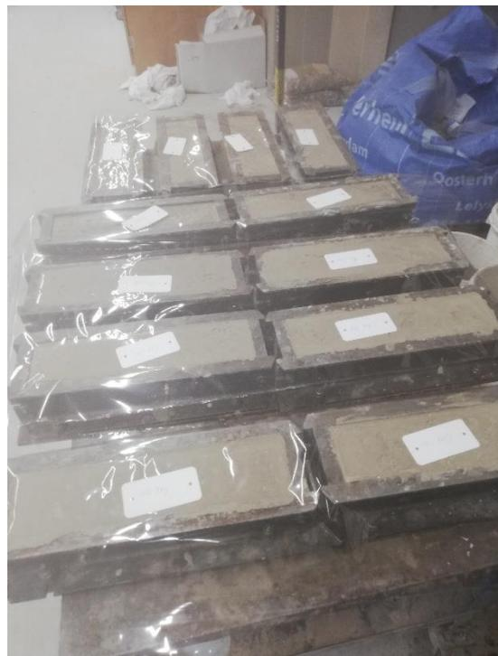
Figure 3.8 Cast concrete prisms. Prisms are labelled and sealed with plastic foil until demoulding.
