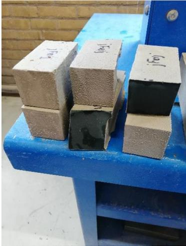
Figure 3.8 Paste compressive strength samples
