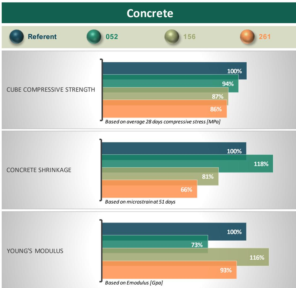
Figure 5.2 Results comparison concrete. Percentages are with respect to the reference mixture.
