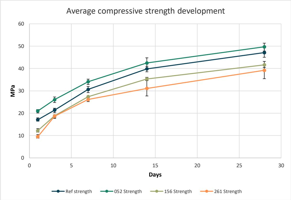
Figure 4.11 Average compressive strength in MPa. Ref strength=Blue, 0 w% SRA; 052 strength=Dark green, 0.52 w% SRA; 156 strength=Light green, 1.56 w% SRA; 261 strength=Orange, 2.61 w% SRA.
