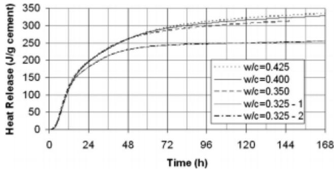
Figure 4.3 Cumulative heat curve of cement hydration for w/c ranging between 0.325-0.425 (Bentz, Peltz, & Winpigler, 2009)
