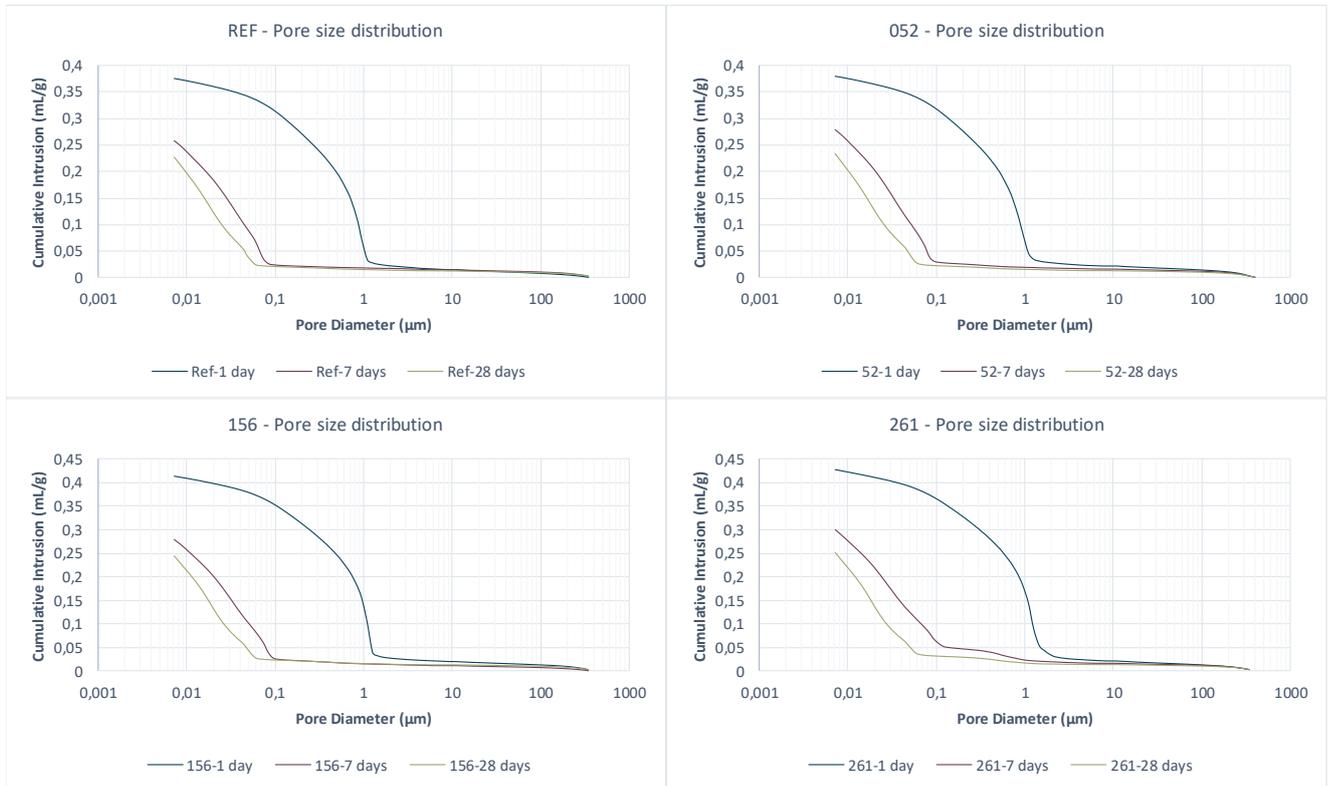
Figure 4.13 Pore size distributions per mixture. Blue=1 day porosity; Red=7 days porosity; Green=28 days porosity
