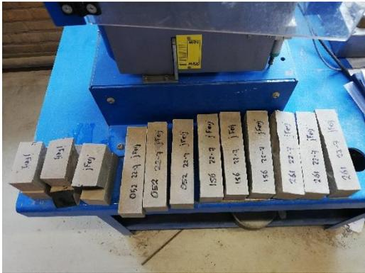
Figure 3.7 Left: broken flexural strength prisms; Right: Prisms ready for testing
