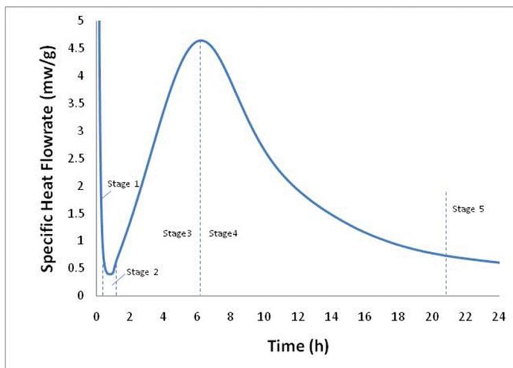
Figure 4.2 Specific Heat Flowrate during cement hydration process (Wadso, n.d.)
