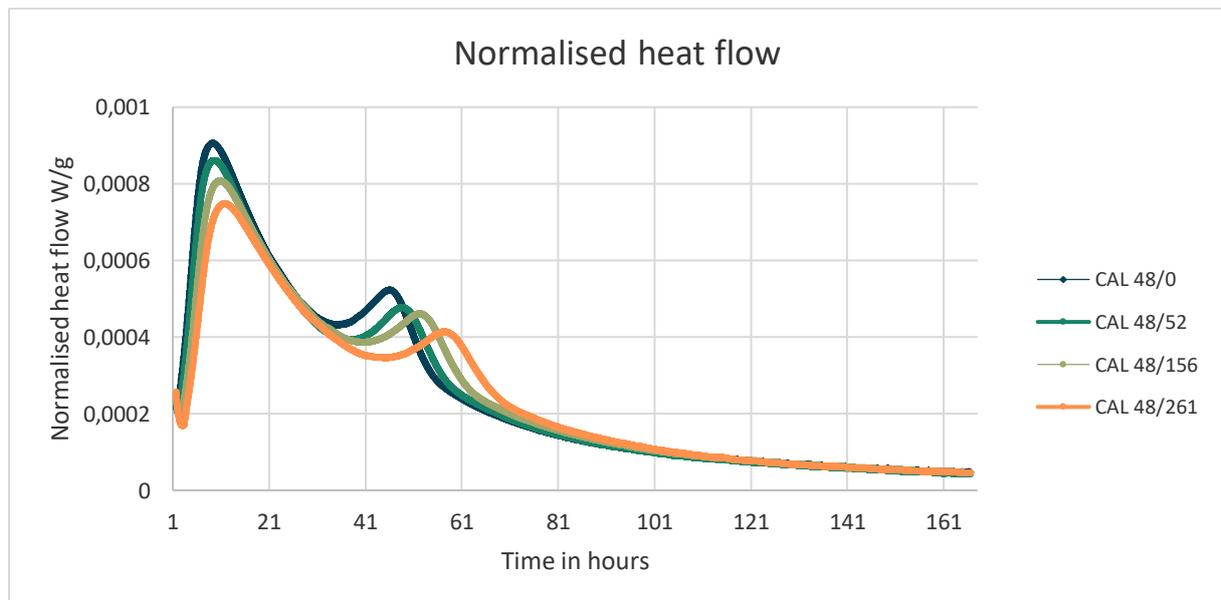
Figure 4.4 Heat flow curves of cement hydration of CEM III/B with w/c=0.48 during the first 7 days of hydration. CAL 48/0 (blue) is reference (0 w% SRA), CAL 48/52 (dark green) is mixture 052 (0.52 w% SRA), CAL 48/156 (light green) is mixture 156 (1.56 w% SRA), CAL 48/261 (orange) is mixture 261 (2.61 w% SRA).
