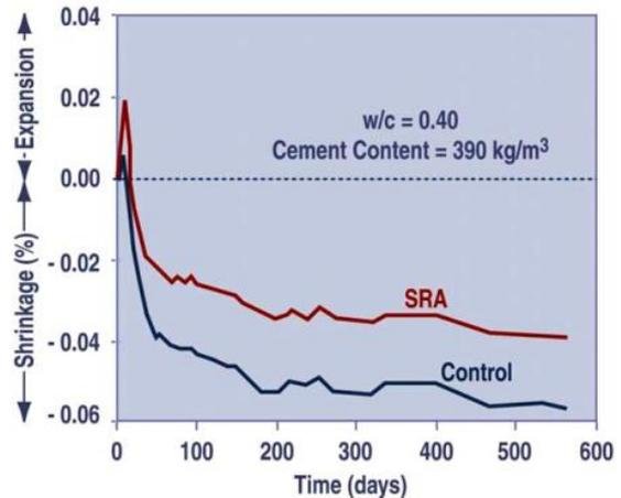
Figure 0.1 Shrinkage reductions with SRA similar to Sika Control 40. 390 kg/m<sup>3</sup> cement, 0.4 w/c and one week wet curing at 25 degrees Celsius. (Collepari et al., 2005)
