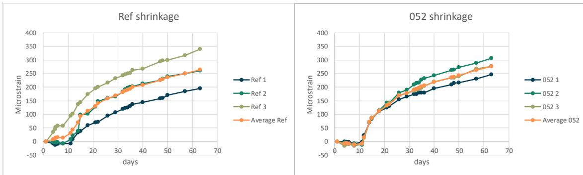
Figure 4.15 Ref autogenous and drying shrinkage; 0 w% SRA      Figure 4.16 052 autogenous and drying shrinkage; 0.52 w% SRA
