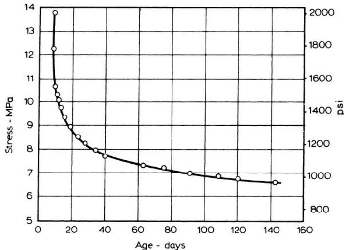
Figure 2.4 Relaxation of stress under a constant strain of  $360 \times 10^{-6}$  (Neville, 1995)
