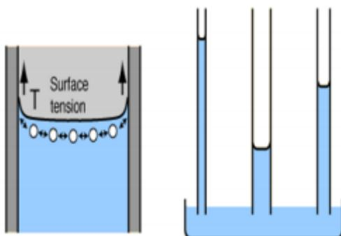
Figure 2.1 Capillary tension in tubes with different diameter (Ben Mya, 2020)
