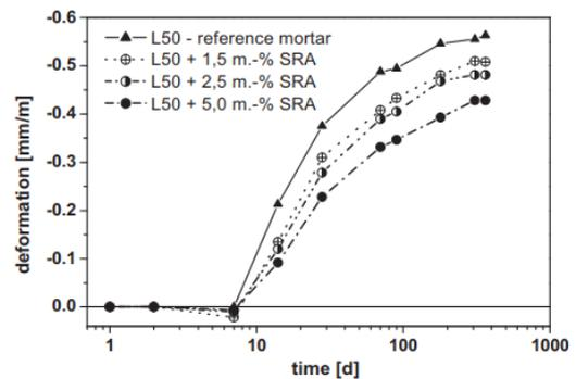
Figure 2.8 Free drying shrinkage of SRA mixes with different concentrations as a function of time (Eberhardt, 2010)
