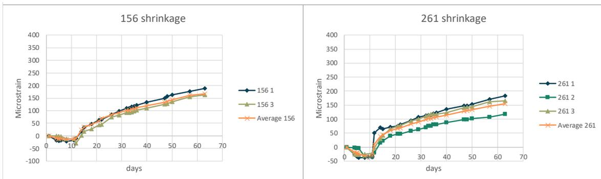
Figure 4.17 156 autogenous and drying shrinkage; 1.56 w% SRA      Figure 4.18 261 autogenous and drying shrinkage; 2.61 w% SRA
