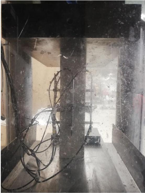
Figure 3.11 Elastic modulus test with attached LVDT's
