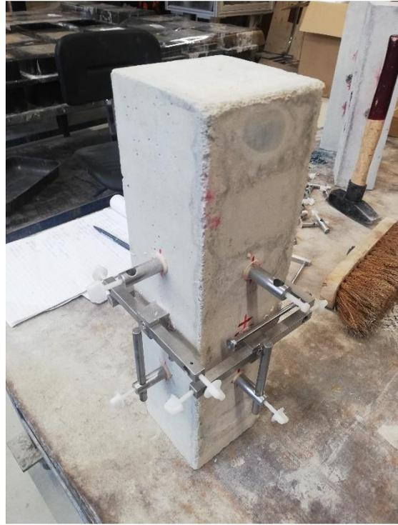
Figure 3.16 Prism with glued mounts for LVDT's
