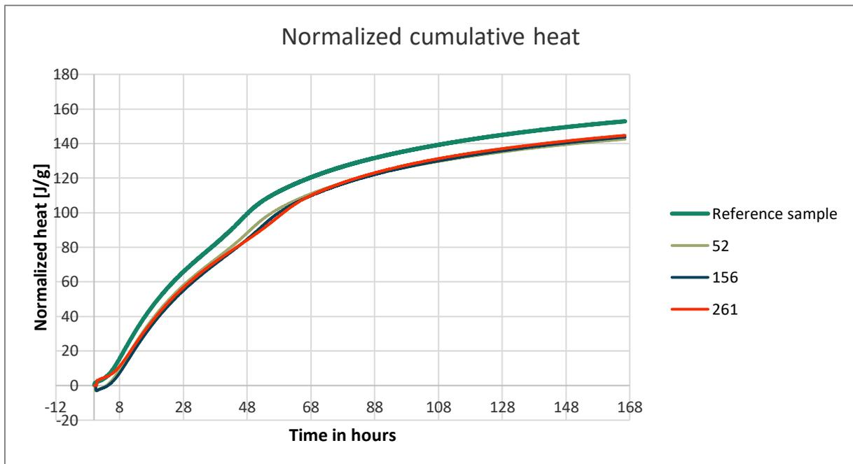
Figure 4.5 Normalized cumulative heat in [J/g] of cement hydration of CEM III/B with  $w/c=0.48$  during the first 7 days of hydration. Reference: Red, 0 w% SRA, 052: Green, 0.52 w% SRA, 156: Blue, 1.56 w% SRA, 261: Orange, 2.61 w% SRA.
