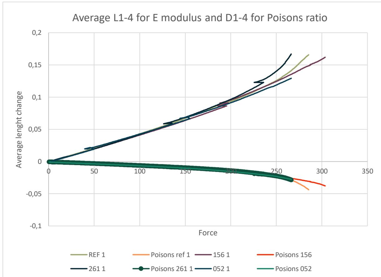
Figure 4.24 Average values L1-4 per mixture; Average values D1-4 per mixture
