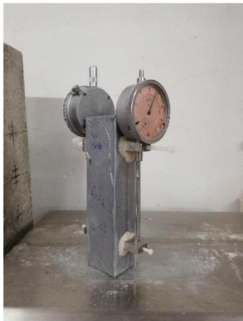
*Figure 3.6 Cement paste autogenous shrinkage setup. Sample is wrapped in watertight tape and measuring clocks are attached.*
