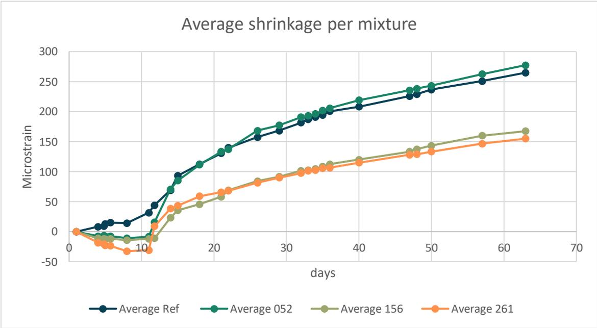
Figure 4.19 Average autogenous + drying shrinkage per mixture. First 7 days is autogenous shrinkage. After 7 days samples are exposed to drying and drying shrinkage is measured. Blue=Reference, 0 w% SRA; Dark green=052, 0.52 w% SRA; Light green=156, 1.56 w% SRA; Orange=261, 2.61 w% SRA.
