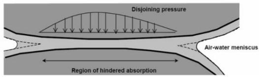
Figure 2.2 Shrinkage mechanisms. Copied from (Reinhardt, 1998, p. 151; Lura, 2003, p. 17)
