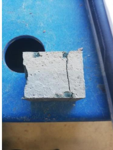
Figure 3.9 Compressive strength sample after failure
