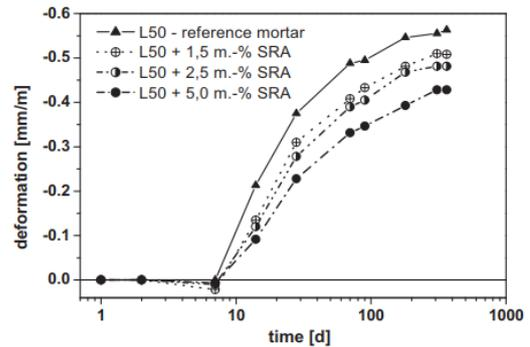
Figure 2.11 Free drying shrinkage of SRA mixes with different concentrations as a function of time (Eberhardt, 2010)
