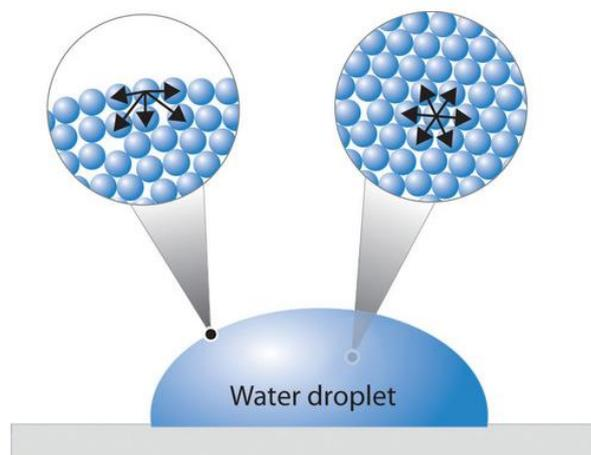
Figure 2.7 Surface tension of water, less interactions at the surface. (Chemistry Libretext, 2019.)
