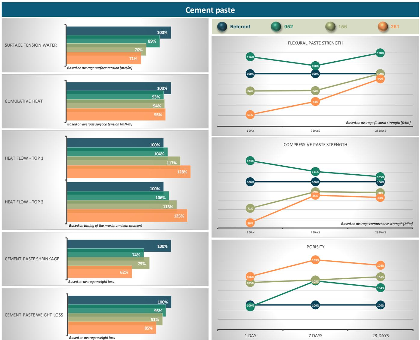
Figure 5.1 Results comparison cement paste. Percentages are with respect to the reference mixture.
